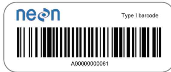
Figure 8. An example of a Type I barcode. These large-size, field-tolerant barcodes have a prefix of 'A' followed by 11 numbers.
