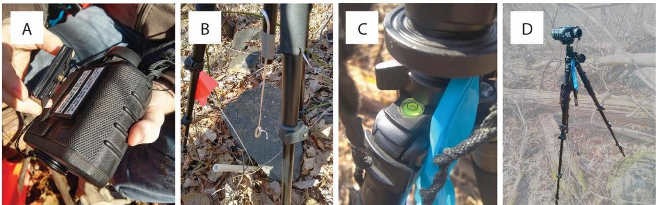
**Figure 8.** Mounting the TruPulse 360R to a non-magnetic tripod for acquiring high-precision horizontal distance measurements. (A) Attaching the tripod mounting plate to the TruPulse 360R; (B) centering the mounted unit and
