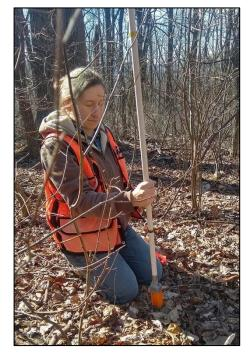
**Figure 11**. A reflective surface mounted to a staff and held at ground level for using the TruPulse 360R in Target Mode = Filter (Flt). Note the person holding the staff has her eyes closed to avoid looking directly at the laser.
