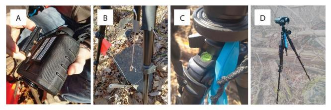
**Figure 8**. Mounting the TruPulse 360R to a non-magnetic tripod for acquiring high-precision horizontal distance measurements. (A) Attaching the tripod mounting plate to the TruPulse 360R; (B) centering the mounted unit and
