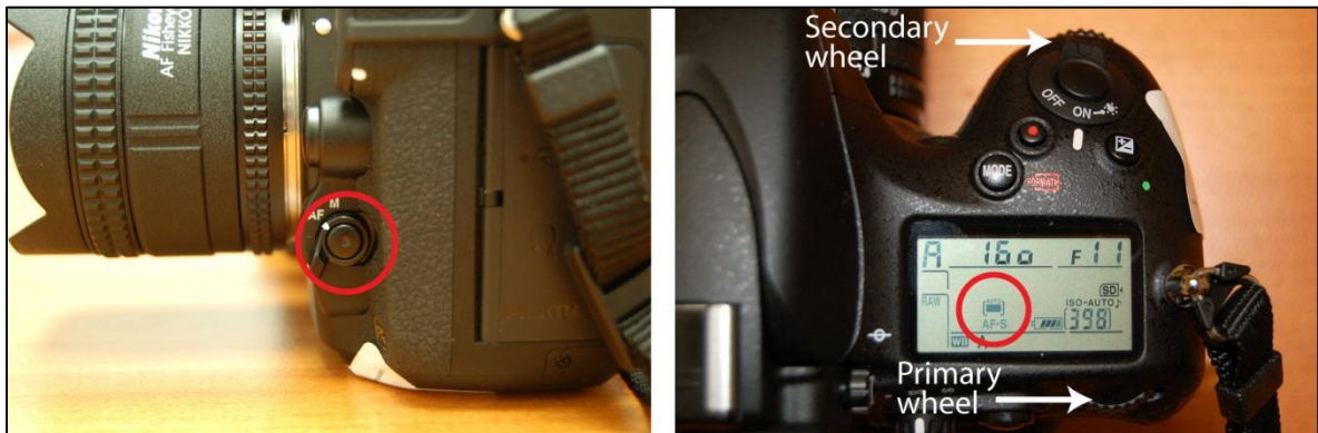
Figure 16. Nikon D800/D810: Configuring focus mode to auto-focus for downward-facing photos.
