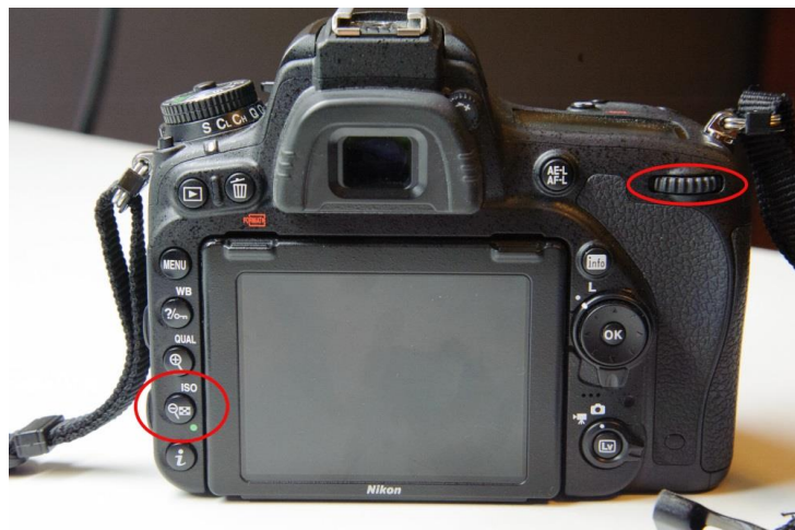
Figure 28. Nikon D750: Configuring ISO sensitivity settings.
