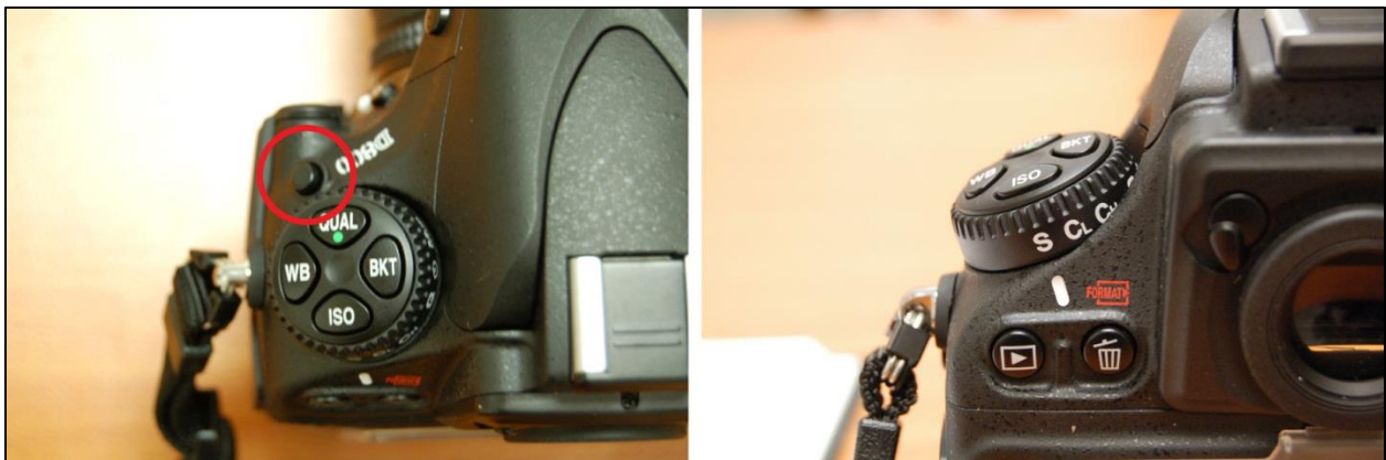
Figure 1. Nikon D800/D810: Setting the shutter-release mode.
