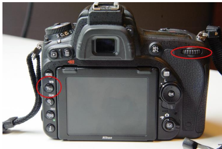
Figure 23. Nikon D750: Configuring white balance settings.
