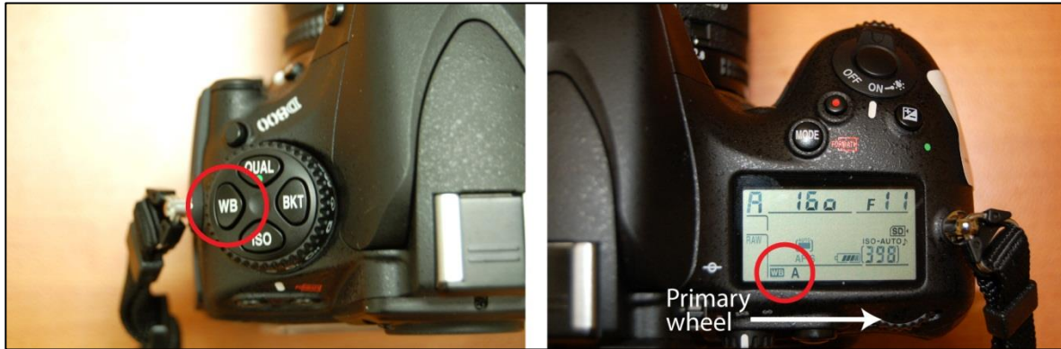
Figure 3. Nikon D800/D810: Adjusting white balance settings.
