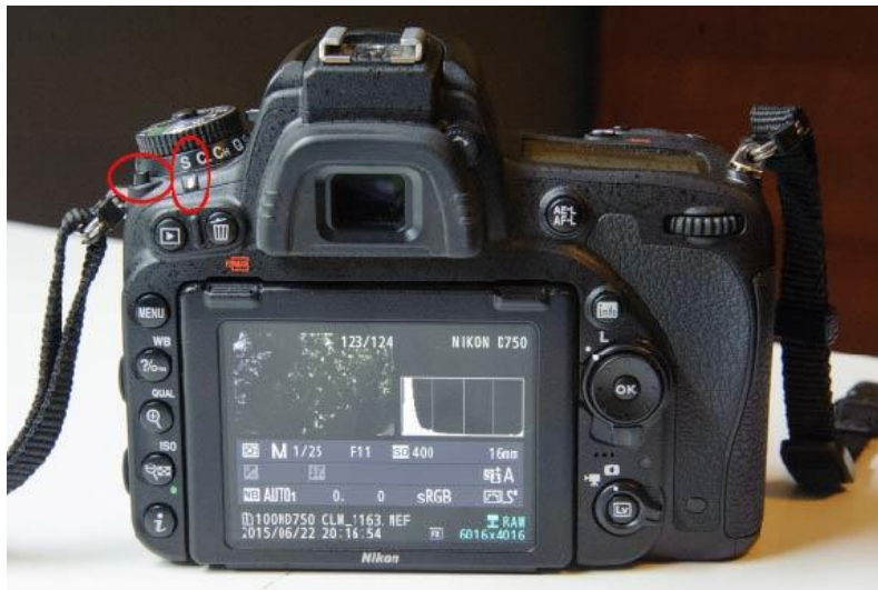
Figure 20. Nikon D750: Setting the shutter-release mode.
