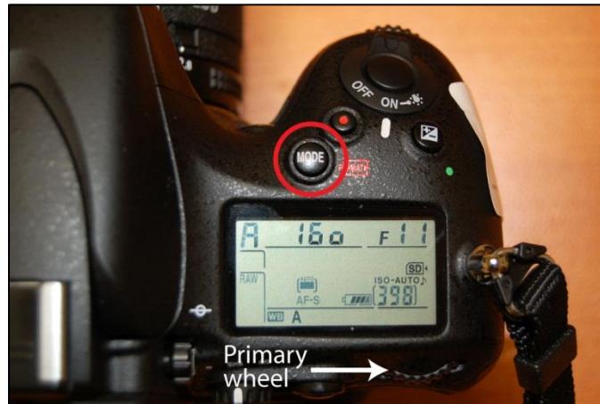
Figure 15. Nikon D800/D810: Setting the desired Exposure mode.
