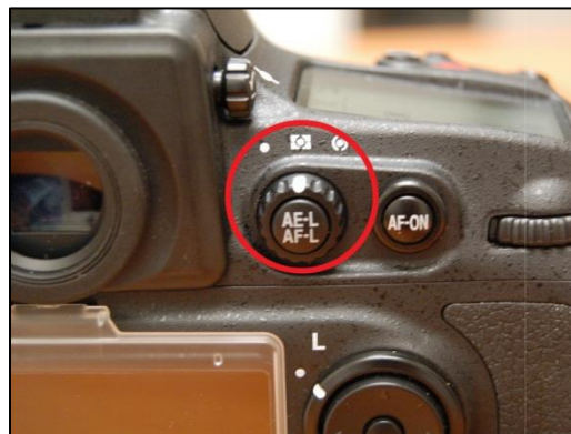
Figure 4. Nikon D800/D810: Setting the metering mode.
