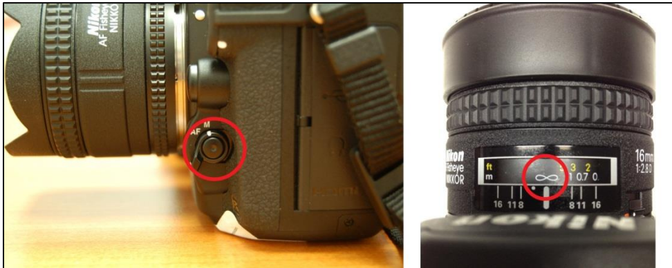
Figure 17. Nikon D800/D810: Configuring focus mode to manual for upward-facing photos.
