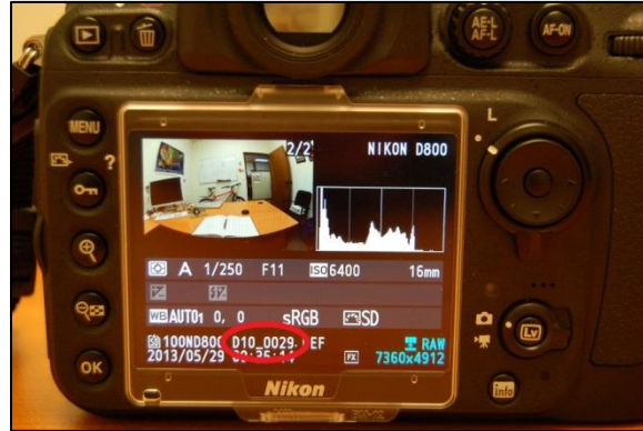
Figure 7. Nikon D800/D810: Locating the file name in the “overview” histogram view during file playback.
