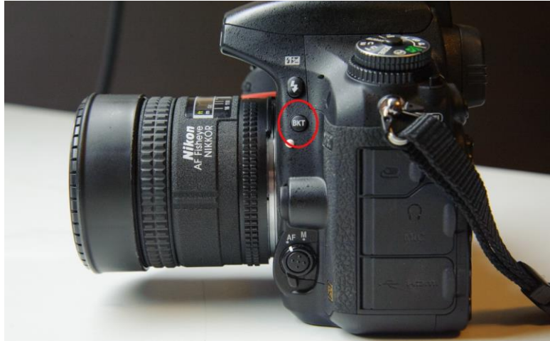
Figure 24. Nikon D750: Toggling bracketing on and off.
