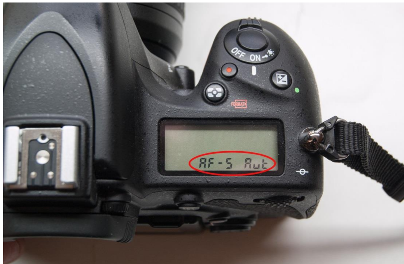
Figure 26. Nikon D750: Top LCD display when camera is configured for single-servo auto-focus auto-mode, where the camera software automatically determines which of the 51 available focus points are used to focus the lens on the subject.
