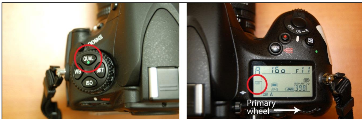
Figure 2. Nikon D800/D810: Setting image quality to RAW.
