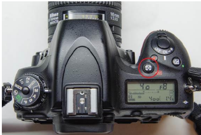
Figure 25. Nikon D750: Configuring the metering mode.
