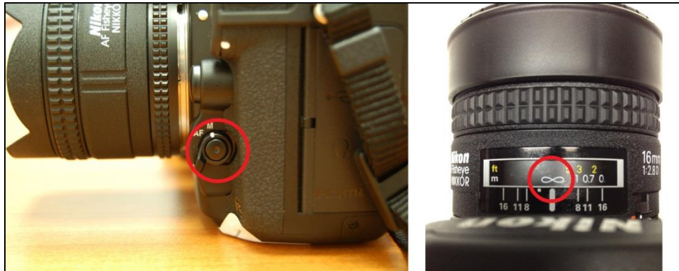
Figure 27. Nikon D750: Focus mode switch, with auto-focus selector button in middle of switch.
