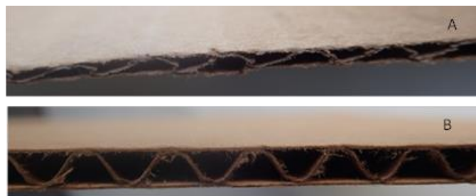
Figure 7. Ventilators with crushed corrugations (A) and fully expanded corrugations (B). Ventilators with crushed corrugations should not be used to press and dry specimens because they cannot channel air to dry the plant; instead, use ventilators with fully expanded corrugations. Ventilators with crushed corrugations are ideally suited for use during mounted specimen glue drying and as family separators in the herbarium cabinet.
