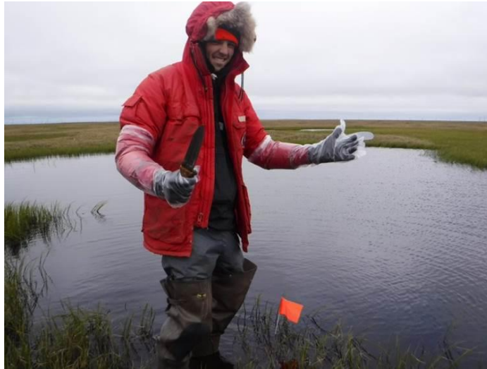
Figure 7. Technician preparing to collect an O horizon monolith in Alaska, using shoulder-length gloves and a hori hori.
