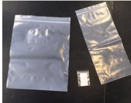
Figure 2. Different size bags to use for N-transformation incubations. Small bag is for the sample metadata.
