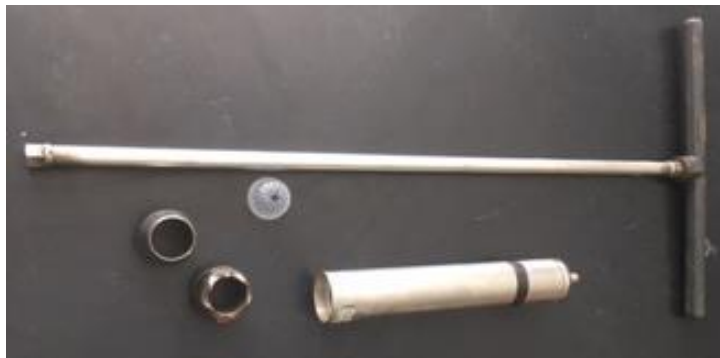
Figure 1. Components of the Multi-stage Sludge Sampler.
