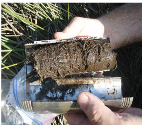
Figure 8. Example of a typical wetland soil core demonstrating a poorly defined boundary between O and M horizons (Photo credit: US Environmental Protection Agency). Note that gloves should be worn by NEON technicians when handling soil samples.
