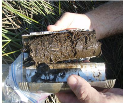
Figure 2. Example of a typical wetland soil core (Photo credit: US Environmental Protection Agency)
