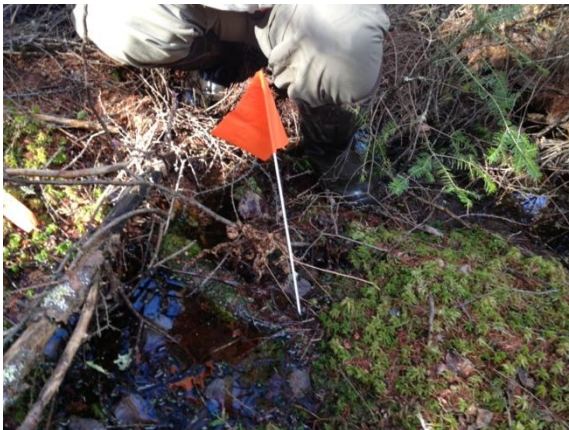
Figure 5. Soil sampling locations with standing water that is very patchy and heterogenous. D05 on the left, D03 DSNY on the right. In these cases, soil temperature can be measured in a dry spot within the chosen X,Y location.
