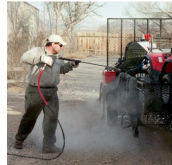
Figure 3. Power washing can be an effective way to clean equipment. Inspect after cleaning.
