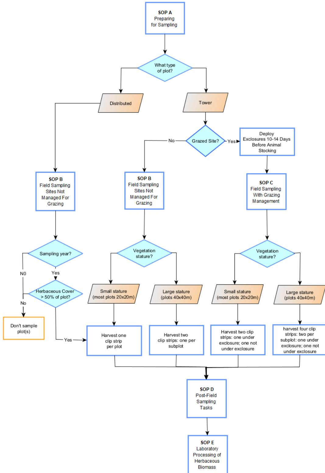
Figure 5. A high level workflow diagram that visually shows how the separate SOPs are sequentially connected.
