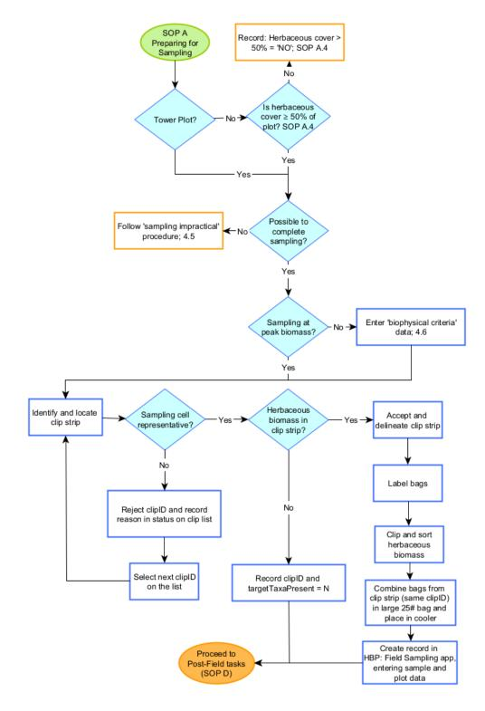
Figure 8. Workflow diagram for a sorted peak biomass bout at sites not managed for grazing (SOP B).
