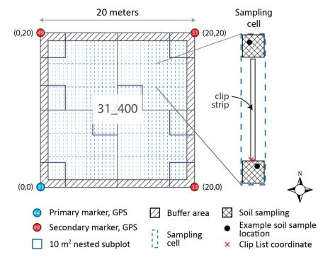
**Figure 2**. A Distributed Plot showing the locations of 3m x 0.5m sampling cells (dashed blue lines) that contain potential 2m x 0.1m clip strips. Coordinates corresponding to the SW corner of the clip strip (red 'X' in blowup) are provided to staff in plot-specific Clip Lists. Clip List coordinates are always relative to the SW corner of the plot (0,0). Sampling cells that overlap 10 m2 nested subplots are omitted from Clip Lists.
