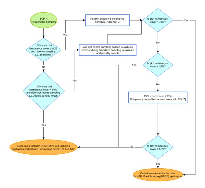
**Figure 7.** Workflow for determining if herbaceous biomass samples should be clipped at Distributed Plots as determined by the plot-scale herbaceous cover; see text in **A.4** for more information.
