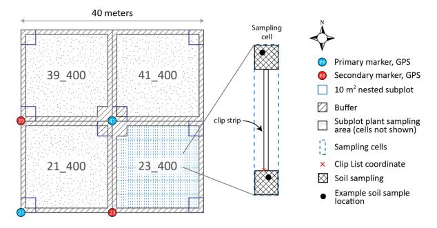
**Figure 3**. A 40m x 40m Tower Plot showing the location of 3m x 0.5m sampling cells (dashed blue lines) within the 20m x 20m subplot 23 400. Cells from the other subplots have been omitted for clarity. The clip strip coordinates
