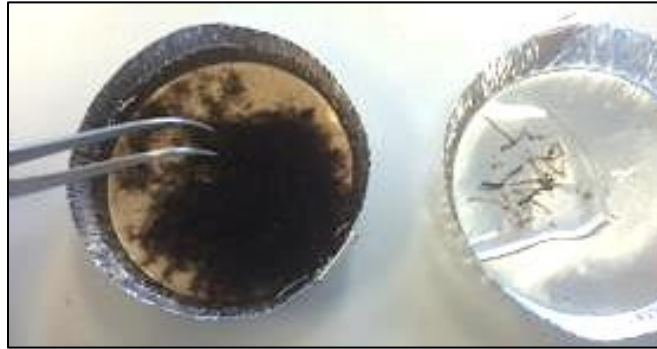
Figure 20. (Left) A dilution subsample, comprised of unsorted root fragments and organic matter, in an aluminum sorting tin. (Right) Sorted root fragments in a second, paired ‘root’ tin. The amount of material in the left tin is a good target when creating dilution subsamples.
