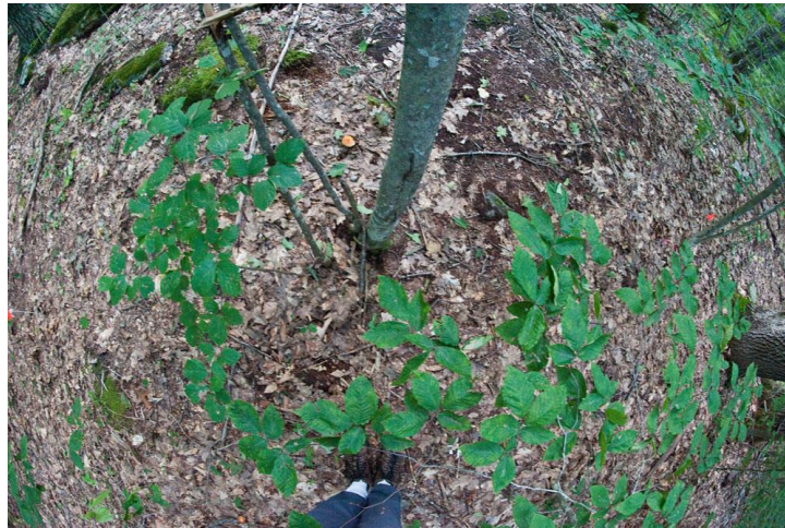
Figure 7. Example of a properly exposed downward-facing DHP at the D01 Harvard Forest site (photo by B. Chemel). Note that green leaves are clearly distinguishable from soil and litter. It is normal for a technician's feet and a portion of the legs to be included in the photo. These will be masked out by the end-user during image analysis.
