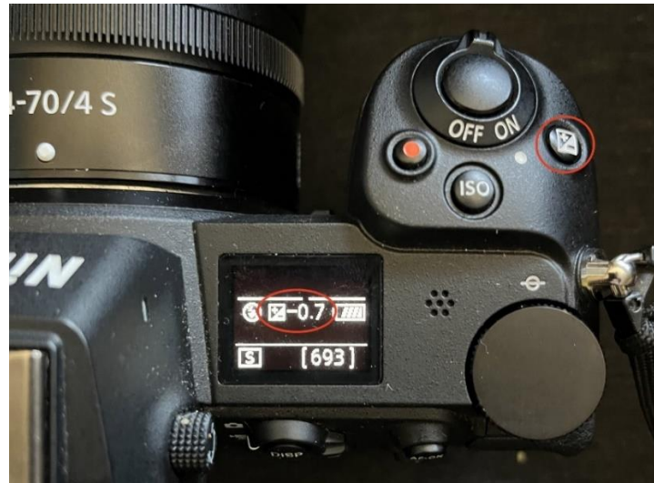
Figure 6. Adjusting exposure with the exposure compensation button. Depress the exposure compensation “+/-” button (upper-right red circle) and rotate the primary wheel to initially set the compensation to “-0.7” (center red circle).
