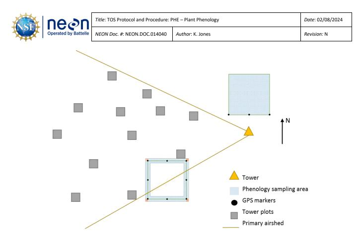
**Figure 1**. Generic site layout for plant phenology including the primary transect (lower left) and phenoCam plot (top right) in relation to Tower plots and primary airshed.
