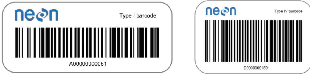
Figure 4. An example of a Type I and Type IV barcode. Type I barcodes are larger in size, field-tolerant barcodes with a prefix of 'A' followed by 11 numbers. Type IV barcodes are smaller in size with a prefix of 'D' followed by 11 numbers.
