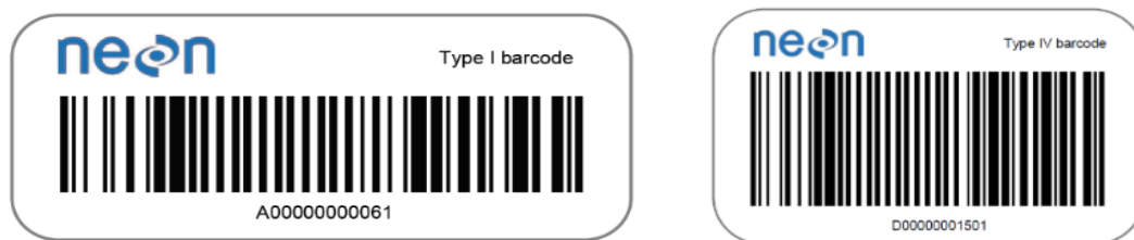
Figure 4. An example of a Type I (left) and Type IV barcode (right). Type I barcodes are larger in size, field-tolerant barcodes with a prefix of 'A' followed by 11 numbers. Type IV barcodes are smaller in size with a prefix of 'D' followed by 11 numbers.
