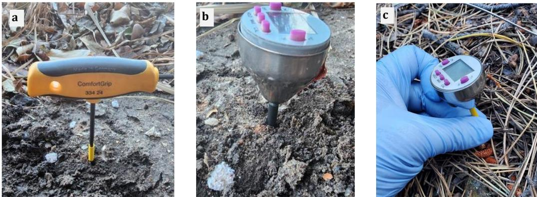
**Figure 13.** Creating a pilot hole, then taking a soil temperature reading at 10 cm depth.
