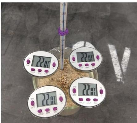
**Figure 8.** Temperature probe calibration setup.
