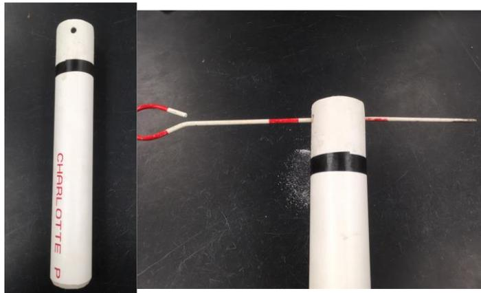
Figure 9. Example PVC cylinder used for soil N transformation sampling.
