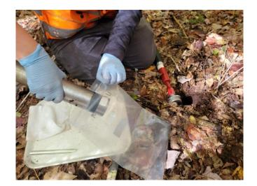
**Figure 17**. Dispensing soil core into bag for homogenization. For certain soils and sampling devices, tapping the corer with a rubber mallet may be very helpful in releasing soil from the barrel.
