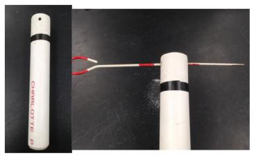
Figure 9. Example PVC cylinder used for soil N transformation sampling.
