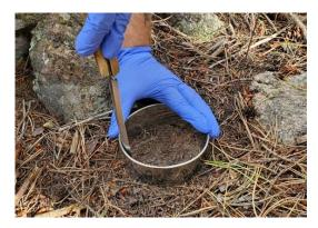
Figure 14. Example use of brownie cutter and hori-hori for O horizon sampling.
