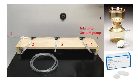
**Figure 23**. Filtration equipment for KCl extractions. Example of a manifold set-up (left) and other equipment including filtration unit (extraction funnel + collection cup) and filters (right).
