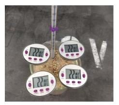
Figure 8. Temperature probe calibration setup.
