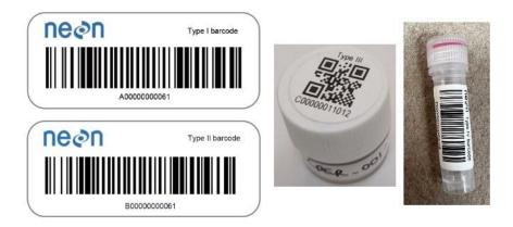
**Figure 10**. Barcode labels used for the various types of soil samples. Type I barcodes are weatherproof but are not cryo-safe; Type II, III, and IV barcodes are cryo-safe and are ideally sized for specific sample containers.
