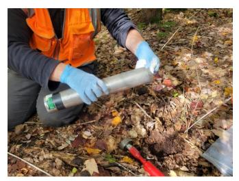
Figure 16. Field staff sterilizing a soil corer using a 70% ethanol wipe. Gloves should be pre-sterilized.
