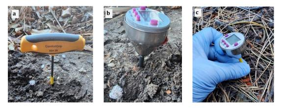
Figure 13. Creating a pilot hole, then taking a soil temperature reading at 10 cm depth.
