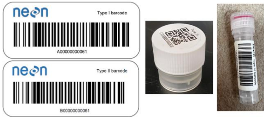
Figure 11. Barcode labels used for the various types of soil samples. Type I barcodes are weatherproof but are not cryo-safe; Type II, III, and IV barcodes are cryo-safe and are ideally sized for specific sample containers.
