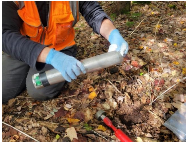
Figure 17. Field staff sterilizing a soil corer using a 70% ethanol wipe. Gloves should be pre-sterilized.
