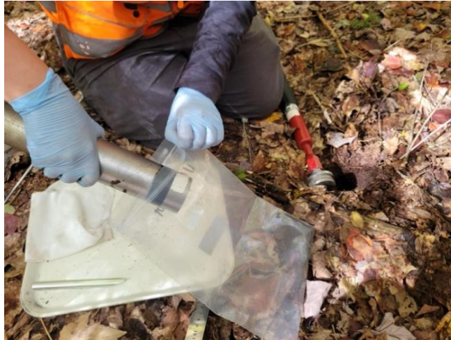
Figure 18. Dispensing soil core into bag for homogenization.
