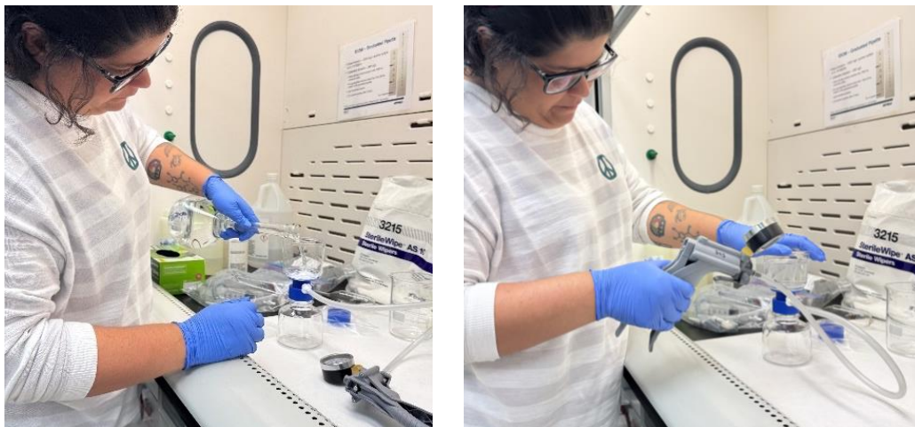
Figure 9. Pouring 70% ethanol into the filter unit and filtering using a hand pump
