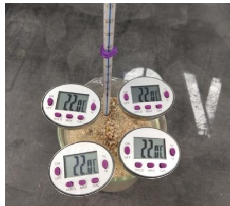
Figure 8. Temperature probe calibration setup.
