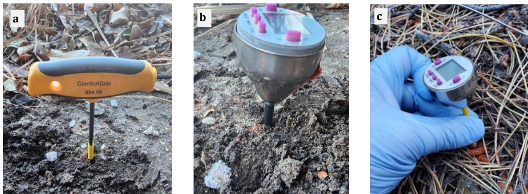
Figure 14. Creating a pilot hole, then taking a soil temperature reading at 10 cm depth.
