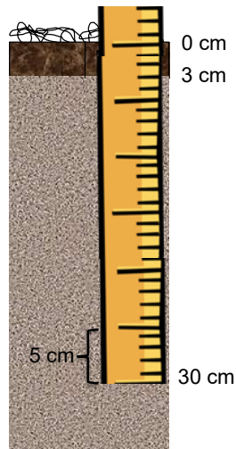
Figure 22. Example soil profile: O horizon sampleTopDepth = 0 cm, sampleBottomDepth = 3 cm; M horizon sampleTopDepth = 3 cm, sampleBottomDepth = 30 cm.
