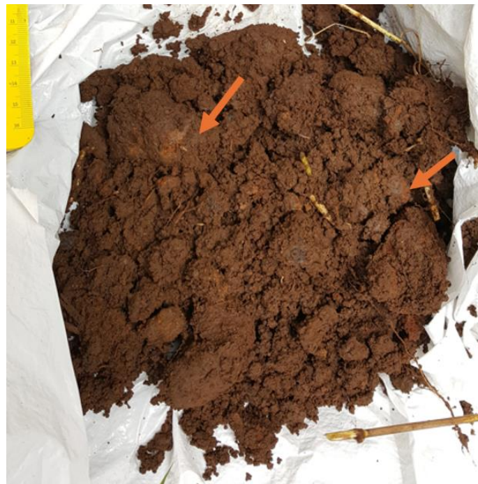
Figure 36. Organic horizon at PUUM containing ferrihydritic elements highlighted by orange arrows.
