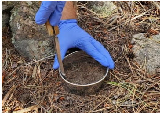
Figure 15. Example use of brownie cutter and hori-hori for O horizon sampling.
