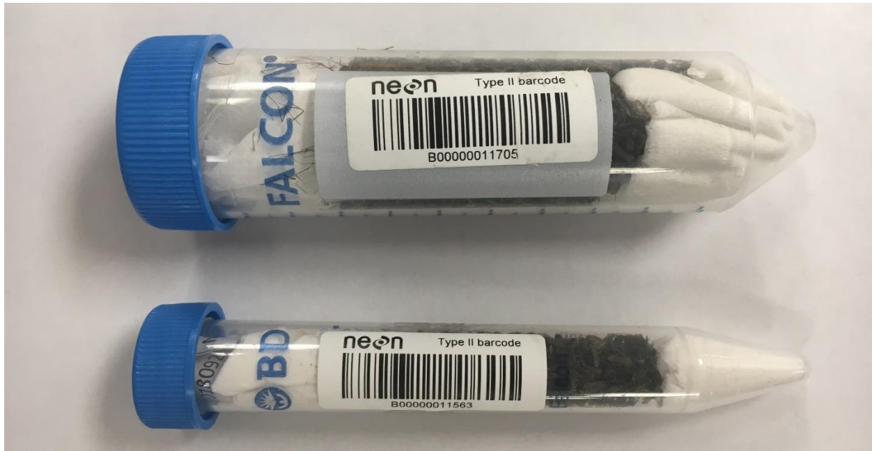
Figure 18. Example of 2 mosquito samples; medium (upper) and small (lower) capture events, respectively. Note that the human-readable sampleID is placed between the cap and upper tissue, away from the mosquitoes.
