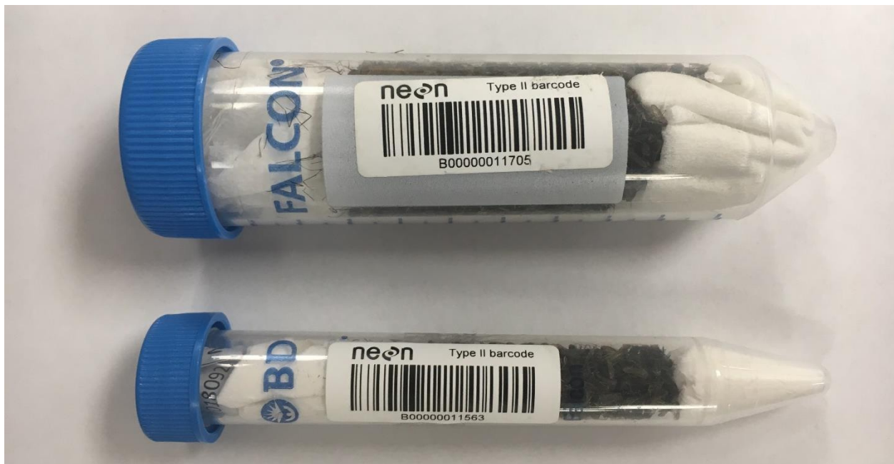
Figure 23. Example of 2 mosquito samples; medium (upper) and small (lower) capture events, respectively. Note that the human-readable sampleID is placed between the cap and upper tissue, away from the mosquitoes.
