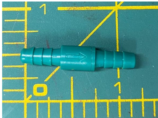
Figure 28. Barb showing arrow indicating direction of air flow.
