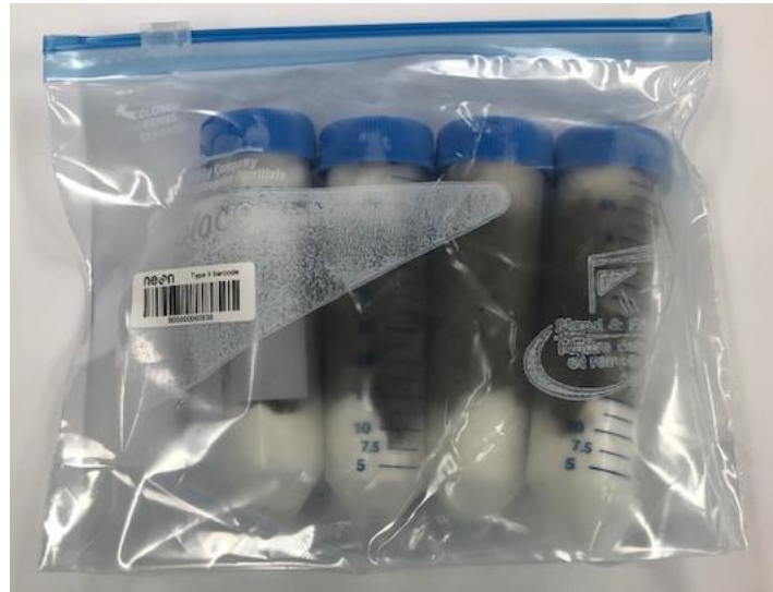
Figure 24. Example of a large volume sample that was placed into multiple vials; only one Type II barcode is used on the exterior of the cryosafe bag.
