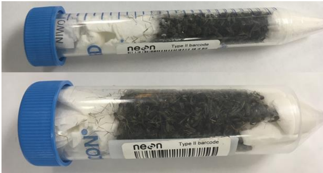
Figure 26. Proper amount of tissue cushioning the top and bottom of two mosquito samples. Note that it is important to place the sampleID label between the cap and upper tissue.
