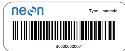
Figure 15. An example of a Type II barcode. These large-size, cryo-safe barcodes have a prefix of 'B' followed by 11 numbers.
