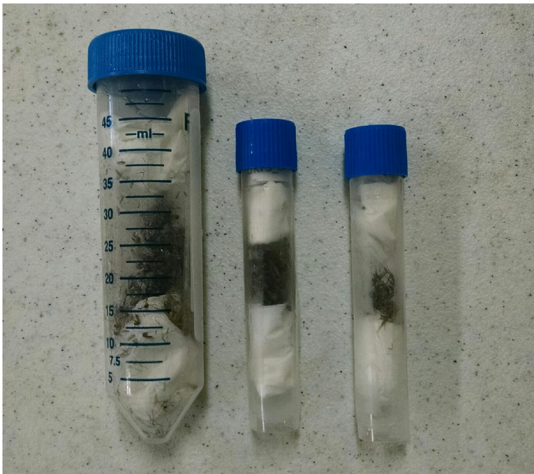
Figure 27. Three mosquito vials. The center vial has an appropriate amount of wadding above and below the sample of mosquitoes. The sample on the left and right have too little material to effectively cushion the sample. Note that the sampleID label must be placed between the upper tissue plug and the lid of the vial.
