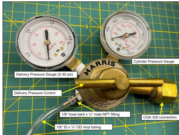
Figure 31. Example regulator with parts labeled.
