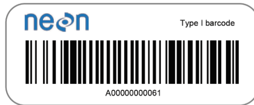
Figure 6. An example of a Type I barcode. These large-size, field-tolerant barcodes have a prefix of 'A' followed by 11 numbers.
