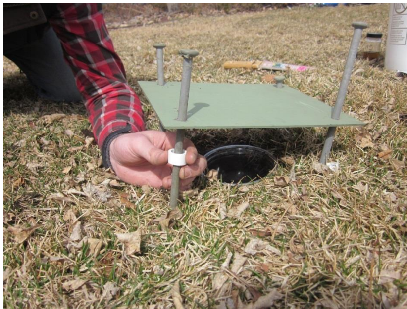
Figure 10. Installing pitfall lid with spacers. Note that the container is flush with the ground. If washers are used, they should be placed between the ground and the bottom of the spacer.
