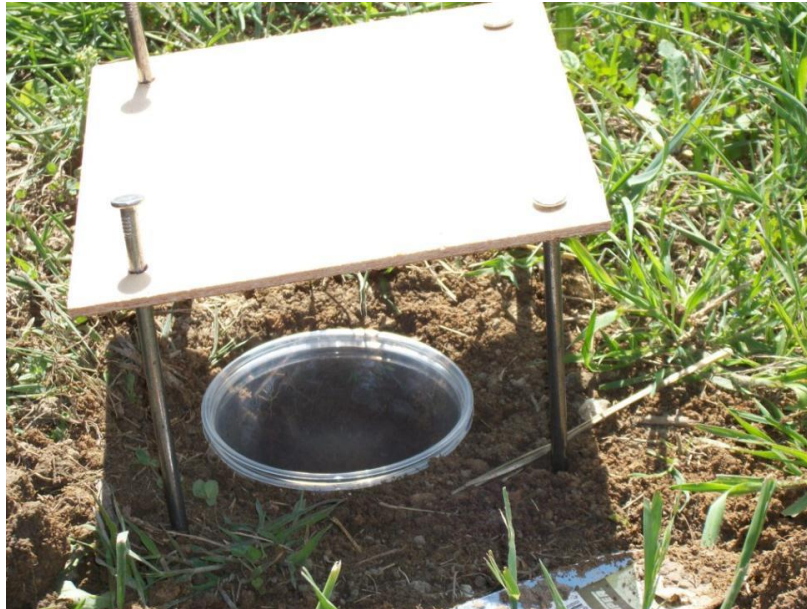
Figure 9. Positioning cover over pitfall trap. Note the pitfall is not sufficiently dug into the ground in this image. The lip should not stick up above the soil surface.
