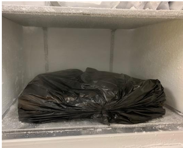
Figure 44. Cornell drawer properly prepared for decontamination and placed in the Ultralow freezer. Ensure the trash bag is tightly sealed to keep moisture and condensation away from the box.
