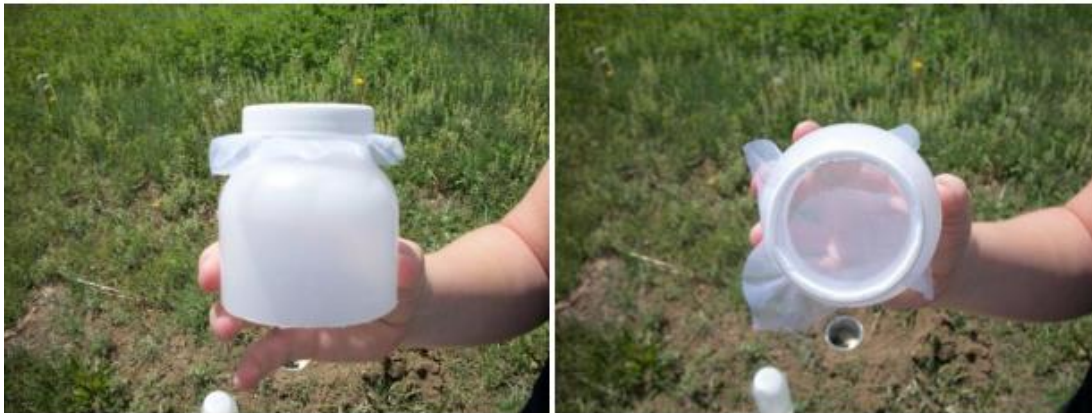
Figure 16. Mesh filter cloth fitted to the top of a modified Nalgene bottle.
