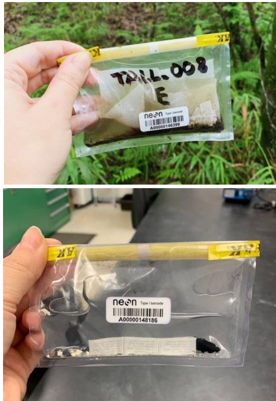
Figure 14. (Above) A packed field sample. (Below) A post-processing sample. Note the whirl of the pack needs to be tight and corner tabs tightly folded to reduce leaks. Storing samples upright in hard-sided containers can also reduce spills.
