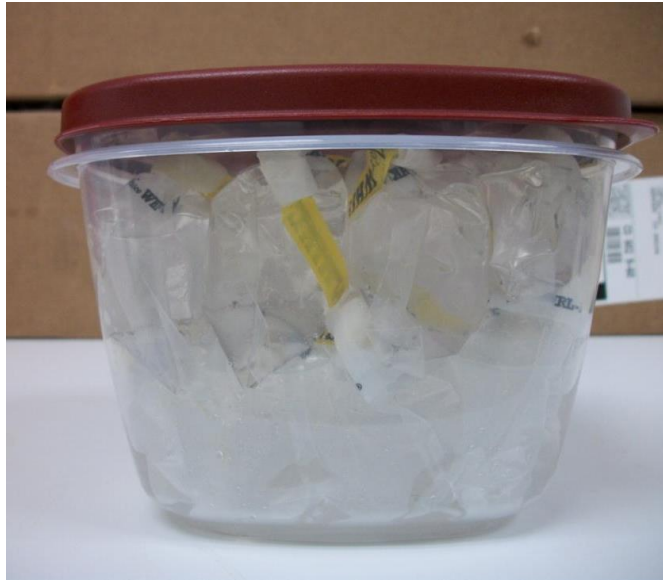
Figure 19. Samples from one sampling bout stored in a sealed container. Label containers using lab tape and permanent markers.
