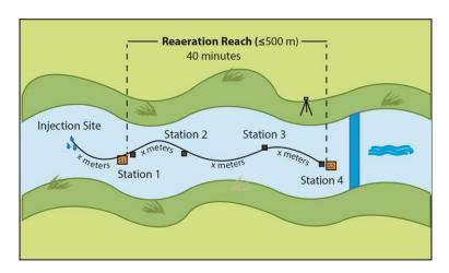
Figure 7. Schematic of stream reach with injection site and four downstream sampling stations. Travel time between Station 1 and 4 should be  $^{\sim}40$  minutes. Note that Reaeration station 1 is co-located with Sensor set 1 and Reaeration station 4 is co-located with sensor set 2.
