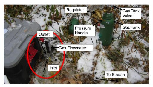
Figure 10. Gas tank, regulator, and flowmeter field setup
