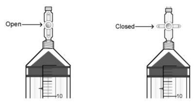
Figure 11. Example of a syringe and stopcock in the "open" and "closed" positions
