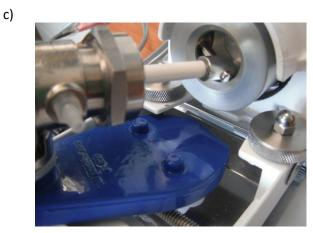
**Figure 19.** Fluid metering pump a) Components of pump drive (left) and pump head (right), b) Configuration of pump head (modified from fluidmetering.com/materials-construction.html), and c) Assembly of pump head into pump drive
