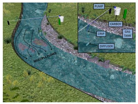
Figure 8. Field setup of the injection site with conservative tracer and inert gas
