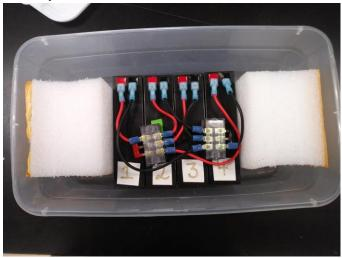
Figure 17. 8V batteries wired in parallel.
