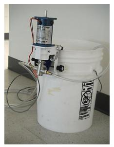
**Figure 9.** Mounting of the pump on the conservative tracer bucket
