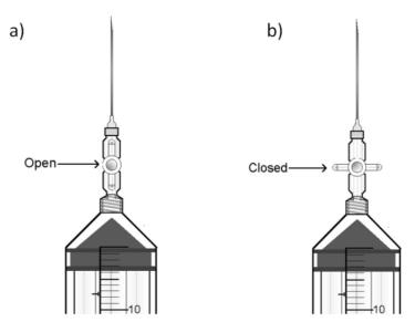
**Figure 14.** Example of a syringe with a stopcock with attached needles in the a) "open" and b) "closed" positions
