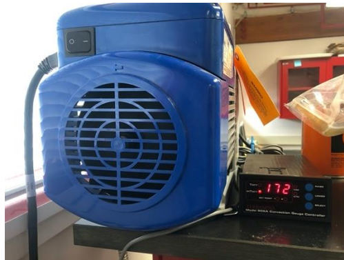
Figure 36. Power switch of vacuum pump and gauge controller reading <200 mTorr.
