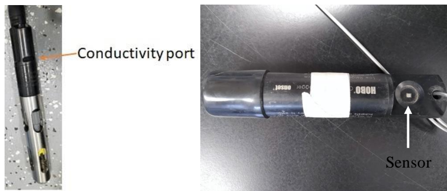
Figure 12. Conductivity sensor is located at the top of the handheld probe and HOBO logger. Ensure the entire probe is in the water and no air bubbles are around the sensors for accurate readings.
