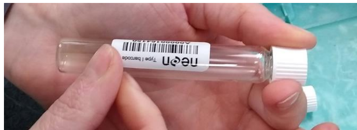
Figure 9. Example of appropriate attachment of reaeration gas vial labels.
