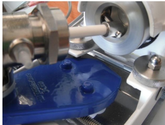
Figure 29. Fluid metering pump a) Components of pump drive (left) and pump head (right), b) Configuration of pump head (modified from fluidmetering.com/materials-construction.html ), and c) Assembly of pump head into pump drive.
