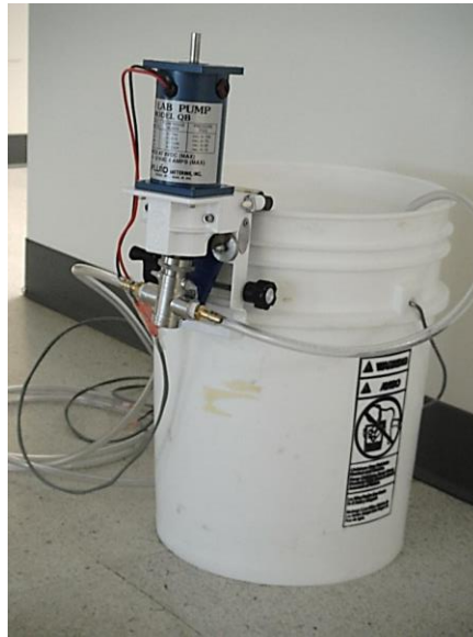
Figure 15. Mounting of the pump on the conservative tracer bucket
