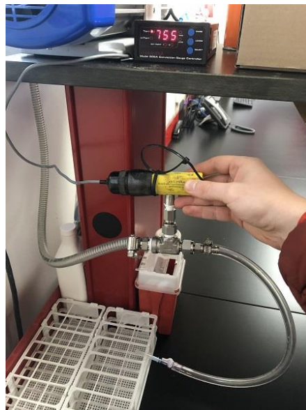
Figure 34. The vacuum pump system for evacuating one vial at a time.
