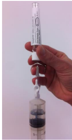
Figure 22. Insertion of the needle into a gas vial through the rubber septum.
