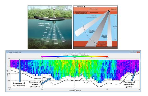
**Figure 57**. Unmeasured areas in the ADCP profile where velocity is extrapolated. Top left: ADCP blanking distance and cell size distribution (credit: SonTek); top right: unmeasured areas of the profile relative to ADCP beams (credit: SonTek); below: the WinRiver II velocity contour with unmeasured areas delineated.
