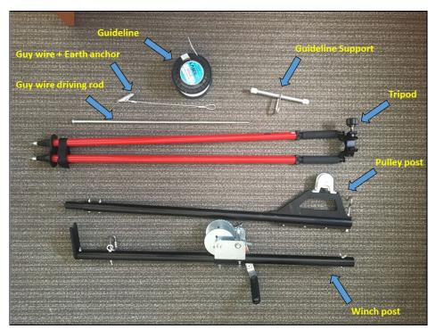
Figure 20. Parts included with the Temporary High Line Assembly.
