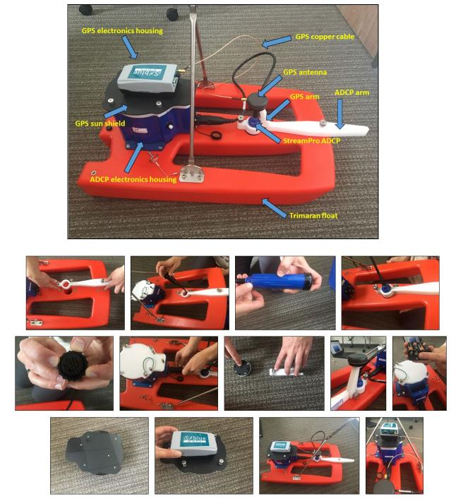
**Figure 15**. Above: Trimaran float, StreamPro ADCP, and SX Blue II GPS antenna components; Below: Illustrated workflow (top left to bottom right) detailing how to configure the StreamPro ADCP unit and SX Blue II GPS antenna to the trimaran float.
