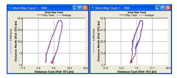
**Figure 71**. Left: A moving bed is likely present as indicated by the open loop; Right: a moving bed is not likely present as indicated by the closed loop.
