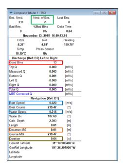
**Figure 56**. Composite Tabular window in WinRiver II, green box: number of ensembles (hold until 10 at transect start/end points); red box: Number of Good Bins (must be >2 to begin transect); purple box: total discharge; blue boxes: water and boat speed; orange box: distance made good (total transect length); brown box: duration (total transect duration must be  $\geq$ 180 seconds).
