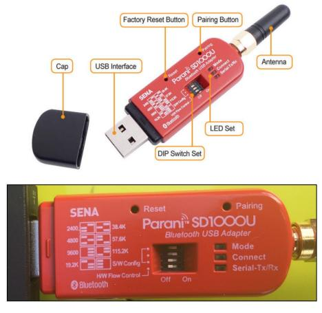
**Figure 17**. Top: Parani-SD1000U USB Bluetooth Adapter with default settings. Bottom: Correct settings for ADCP and GPS Bluetooth configuration.
