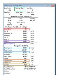
**Figure 31**. Composite Tabular window in WinRiver II, green box: Number of Ensembles (hold until 10 at transect start/end points); red box: Number of Good Bins (must be >2 to begin transect); purple box: Total Discharge; blue boxes: Water and Boat speed; orange box: Distance made good (MG = total transect length); brown box: Duration (total transect duration must be  $\geq$ 180 seconds).
