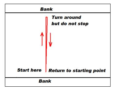
Figure 70. Illustration of the Loop Moving Bed Test procedure.
