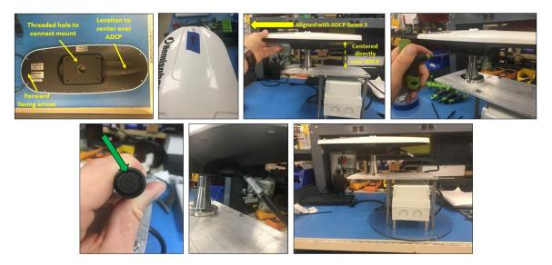
Figure 39. Installing the Hemisphere V102 GPS antenna onto the ARC-Boat GPS mount.
