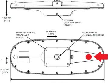
**Figure 40**. Hemisphere V102 GPS antenna schematics. Top: the back of the unit with cable port show; Middle: the side of the unit showing one of two set screw locations; Bottom: the base of the unit, the red circle to the right of the unit indicates the location that must be centered over the ADCP, the white arrow to the left of the unit indicates the direction the unit must face so that it is oriented toward Beam 3 of the ADCP.
