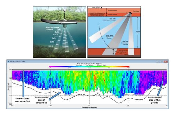
**Figure 74**. Unmeasured areas in the ADCP profile where velocity is extrapolated. Top left: ADCP blanking distance and cell size distribution (credit: SonTek); top right: unmeasured areas of the profile relative to ADCP beams (credit: SonTek); below: the WinRiver II velocity contour with unmeasured areas delineated.
