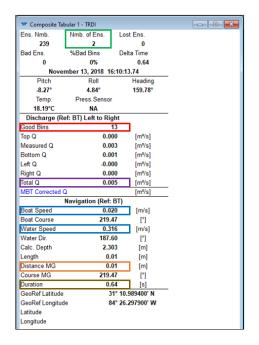
**Figure 73**. Composite Tabular window in WinRiver II, green box: number of ensembles (hold until 10 at transect start/end points); red box: Number of Good Bins (must be >2 to begin transect); purple box: total discharge; blue boxes: water and boat speed; orange box: distance made good (total transect length); brown box: duration (total transect duration must be  $\geq$ 180 seconds).
