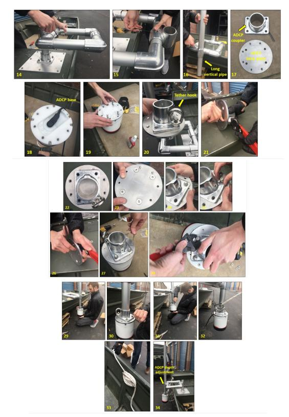
Figure 65. Assembly of the ADCP mount on a piloted boat.
