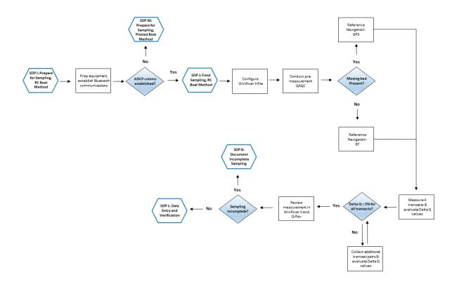
**Figure 8**. A detailed workflow diagram that visually shows the workflow for river sites using the Remote Controlled Boat Method.
