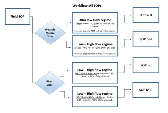
Figure 3. A high level workflow diagram that visually shows how the separate SOPs are sequentially connected.
