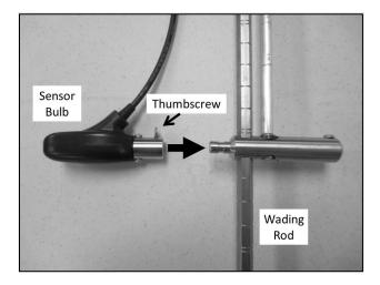
Figure 10. Velocity meter and the thumbscrew that attaches it to the wading rod.
