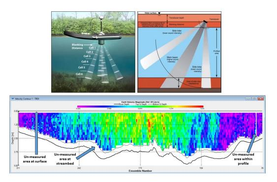
**Figure 32.** Unmeasured areas in the ADCP profile where velocity is extrapolated. Top left: ADCP blanking distance and cell size distribution (credit: SonTek); top right: unmeasured areas of the profile relative to ADCP beams (credit: SonTek); below: the WinRiver II velocity contour with unmeasured areas delineated.
