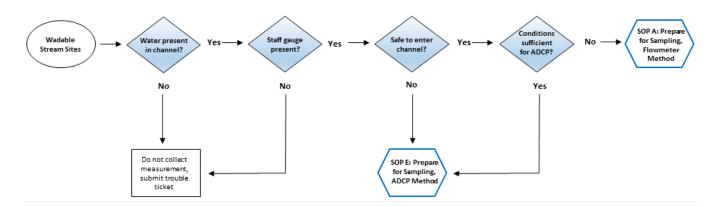
Figure 4. A high level workflow diagram that visually shows the workflow for wadable stream sites.
