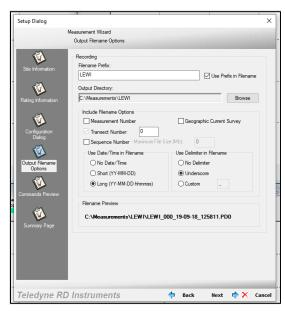
**Figure 44**. Required settings in the WinRiver II Output Filename Options dialogue box within the Measurement Wizard.
