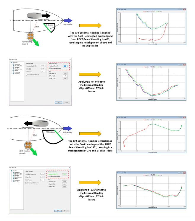
Figure 41. Applying External Heading offsets to align GPS and Bottom Track Ship Tracks.
