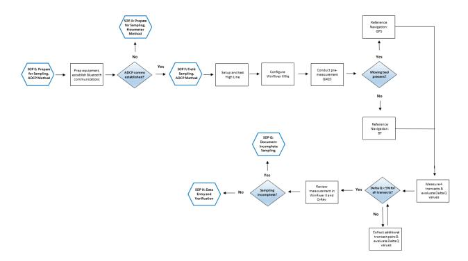
**Figure 6**. A detailed workflow diagram that visually shows the workflow for wadable stream sites using the ADCP Method.
