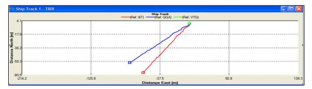
**Figure 30**. Above: Bottom Track and GPS data are in good agreement, indicating proper compass calibration, an accurate Magnetic Variation value, and low GPS latency; Below: Bottom Track and GPS data are in poor agreement, indicating poor compass calibration, an inaccurate Magnetic Variation value, and/or high GPS latency.
