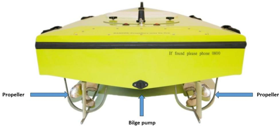
**Figure 47.** Above: Top of the ARC-Boat (not pictured: ADCP Adapter with GPS mount); Below: Stern of the ARC-Boat
