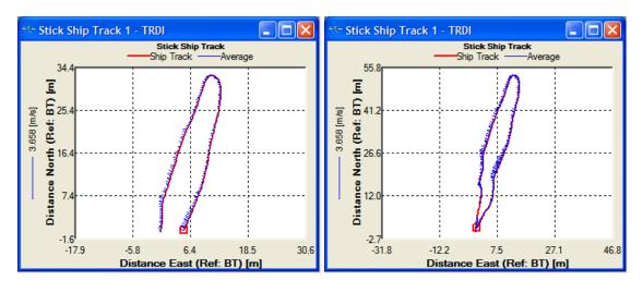
**Figure 53**. Left: A moving bed is likely present as indicated by the open loop; Right: a moving bed is not likely present as indicated by the closed loop.
