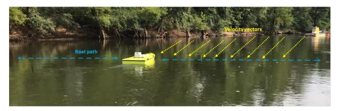
**Figure 48**. When surface water velocity is sufficient operate the ARC-Boat in such a way that the bow is pointed into the velocity vectors and the boat is crabbed across the channel.
