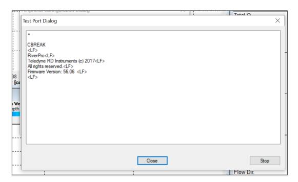
Figure 64. River Pro ADCP Test Port Dialog indicating that ADCP data is streaming from the ADCP to the laptop.
