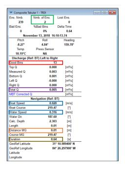
**Figure 56**. Composite Tabular window in WinRiver II, green box: number of ensembles (hold until 10 at transect start/end points); red box: Number of Good Bins (must be >2 to begin transect); purple box: total discharge; blue boxes: water and boat speed; orange box: distance made good (total transect length); brown box: duration (total transect duration must be ≥180 seconds).
