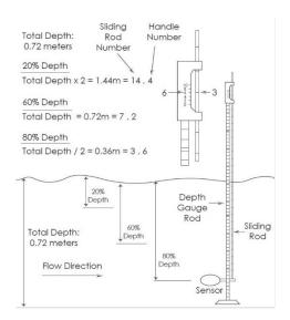
**Figure 14**. Wading rod adjustments at 60% (one-point), and 20% and 80% (two-point) depths. Station depth = 0.72m.
