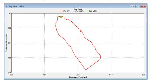
**Figure 51**. The WinRiver II Ship Track window observed during a loop moving bedtest. The green box indicates the boat starting position, the line shows the boat path as it is navigating across the channel and turned back around toward the starting bank, and the red box indicates the boat ending position.
