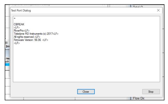
Figure 43. River Pro ADCP Test Port Dialog indicating that ADCP data is streaming from the ADCP to the laptop.
