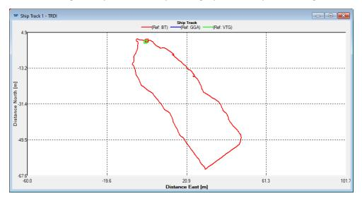
**Figure 26**. The WinRiver II Ship Track window observed during a loop moving bedtest. The green box indicates the boat starting position, the line shows the boat path as it is navigating across the channel and turned back around toward the starting bank, and the red box indicates the boat ending position.
