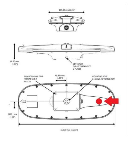
**Figure 40**. Hemisphere V102 GPS antenna schematics. Top: the back of the unit with cable port show; Middle: the side of the unit showing one of two setscrew locations; Bottom: the base of the unit, the red circle to the right of the unit indicates the location that must be centered over the ADCP, the white arrow to the left of the unit indicates the direction the unit must face so that it is oriented toward Beam 3 of the ADCP.
