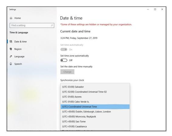
**Figure 24**. Set the PC used for the discharge measurement to (UTC) Coordinated Universal Time and match the ADCP clock to this setting.
