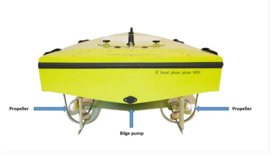
**Figure 47**. Above: Top of the ARC-Boat (not pictured: ADCP Adapter with GPS mount); Below: Stern of the ARC-Boat
