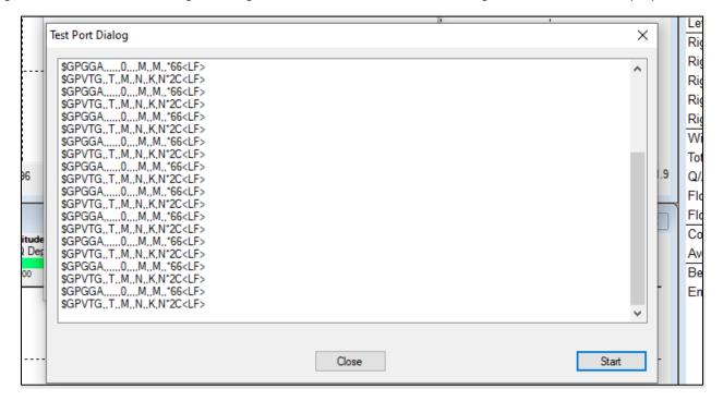
Figure 19. GPS Test Port Dialog indicating that GPS data is streaming from the GPS antenna to the laptop.
