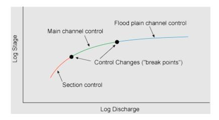
Figure 79. Schematic representation of control range in a rating curve. (Illustration: Braca 2008).
