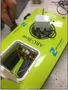
**Figure 38**. The ARC-Boat setup with the RiverPro ADCP adapter. A: connect the long set screws to the top of the ADCP; B: connect a fully charged 12V battery inside the ADCP adapter; C: connect the long set screws to the circular base plate of the adapter with the wingnuts, connect the ADCP cable coming out of the adapter to the
