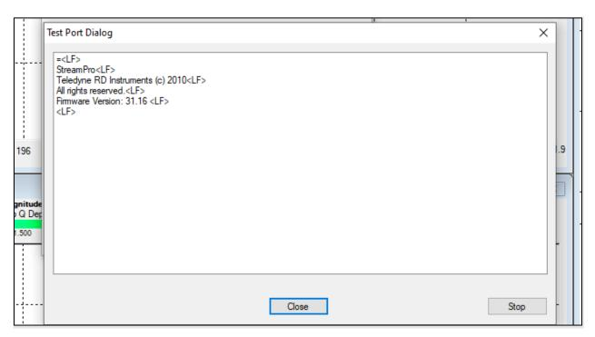
Figure 18. ADCP Test Port Dialog indicating that StreamPro ADCP data is streaming from the ADCP to the laptop.
