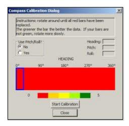
**Figure 25**. WinRiver II compass calibration dialog box. Upon initializing the compass calibration, all bars begin as bright red as shown above. Perform the compass calibration until all bars are the dark green color indicated in the far right side of the color scale.
