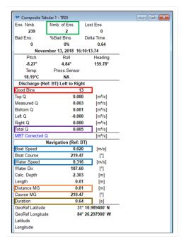
**Figure 73**. Composite Tabular window in WinRiver II, green box: number of ensembles (hold until 10 at transect start/end points); red box: Number of Good Bins (must be >2 to begintransect); purple box: total discharge; blue boxes: water and boat speed; orange box: distance made good (total transect length); brown box: duration (total transect duration must be ≥180 seconds).
