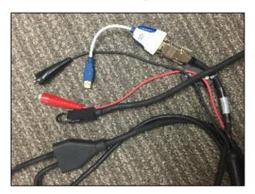
**Figure 63**. Serial cables that connect the ADCP to the 12V battery and the laptop PC. Note the white RS-232 USB adapter that must be included in the set.
