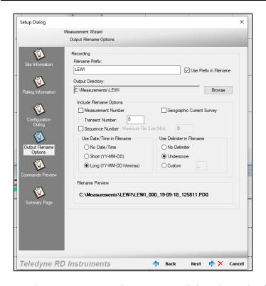
**Figure 66**. Required settings in the WinRiver Output Filename Options dialogue box within the Measurement Wizard.
