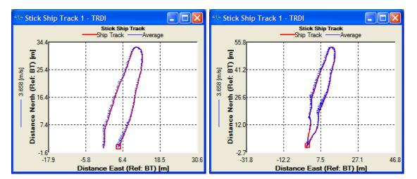
**Figure 28**. Left: A moving bed is likely present (not open loop); Right: a moving bed is not likely present (note closed loop).
