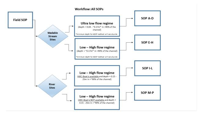
Figure 3. A high level workflow diagram that visually shows how the separate SOPs are sequentially connected.
