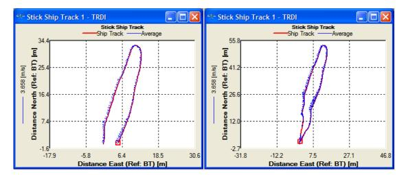
**Figure 71**. Left: A moving bed is likely present as indicated by the open loop; Right: a moving bed is not likely present as indicated by the closed loop.
