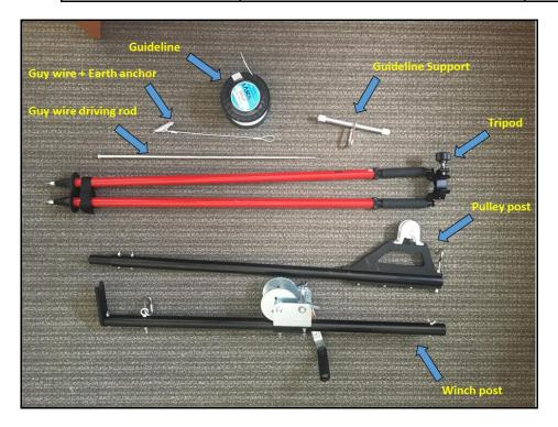
Figure 20. Parts included with the Temporary High Line Assembly.
