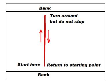
Figure 27. Illustration of the Loop Moving BedTest procedure.
