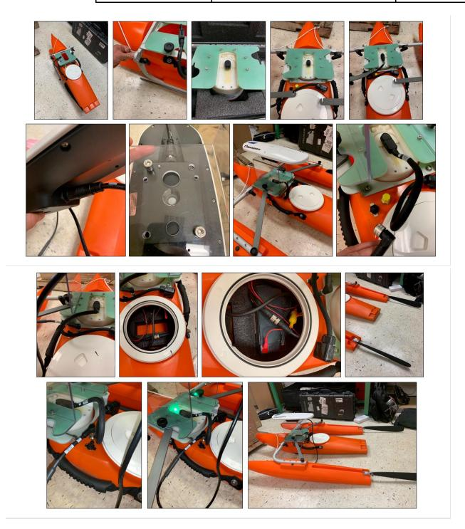
**Figure 16**. Illustrated workflow (top left to bottom right) detailing how to configure the RiverPro ADCP unit and the Hemisphere GPS antenna to the trimaran float.
