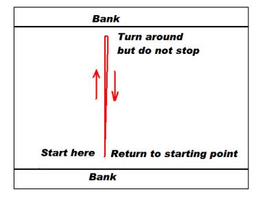
**Figure 70**. Illustration of the Loop Moving Bed Test procedure.
