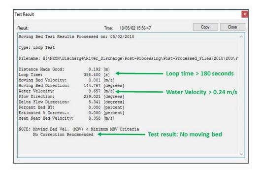
**Figure 72**. Moving Bed Loop Test Result window. In this example the required conditions were met in order to evaluate a moving bed (Loop time, water velocity) and a moving bed was not detected (the moving bed velocity < the moving bed velocity criteria), thus no correction was recommended.
