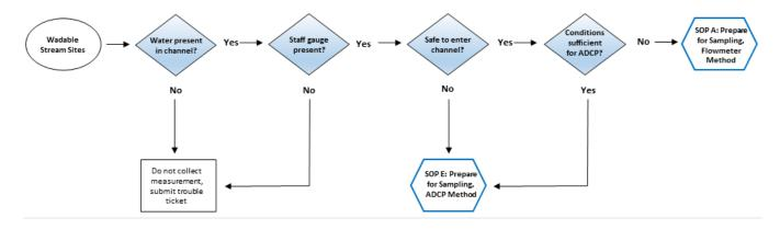
Figure 4. A high level workflow diagram that visually shows the workflow for wadable stream sites.
