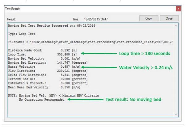
**Figure 29**. Moving Bed Loop Test Result window. In this example the required conditions were met to in order to evaluate a moving bed (Loop time, water velocity) and a moving bed was not detected (the moving bed velocity < the moving bed velocity criteria), thus no correction was recommended.
