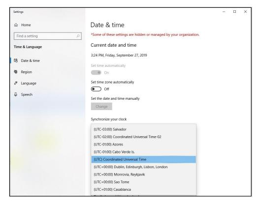
**Figure 67**. Set the PC used for the discharge measurement to (UTC) Coordinated Universal Time and match the ADCP clock to this setting.
