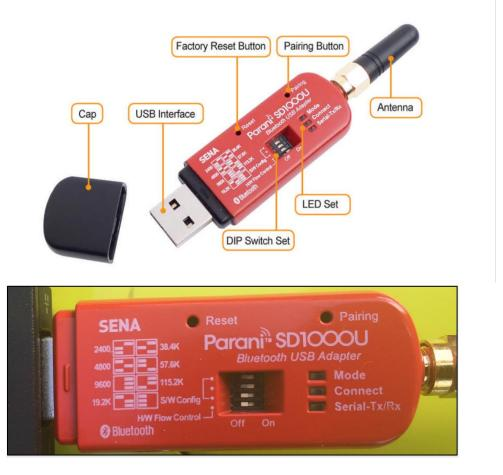
**Figure 42**. Top: Parani-SD1000U USB Bluetooth Adapter with default settings. Bottom: Correct settings for ADCP and GPS Bluetooth configuration.
