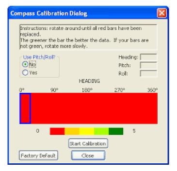
**Figure 50**. ADCP Compass Calibration dialog box. The entirety of the horizontal bar is red upon initiating the test. Rotate the boat slowly and steadily so that bar is colored dark green throughout.
