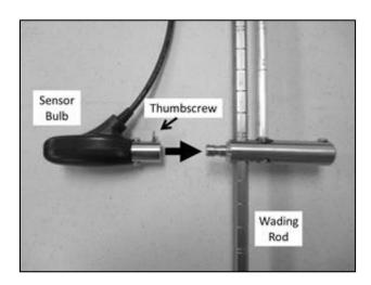
Figure 10. Velocity meter and the thumbscrew that attaches it to the wading rod.
