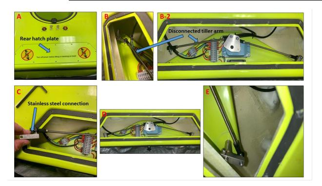
Figure 77. Repairing a disconnected tiller on the ARC-Boat.
