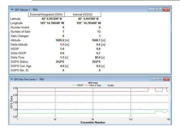
**Figure 45**. Above: GPS Tabular window that confirms GPS data is available and is being collected; Below: GPS Time Series window that indicates GPS data is streaming.
