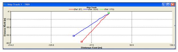
**Figure 55**. Above: Ship Track graphs to evaluate Bottom Track vs GPS data. Above: Track and GPS data are in good agreement, indicating proper compass calibration, an accurate Magnetic Variation value, and low GPS latency; Below: Bottom Track and GPS data are in poor agreement, indicating poor compass calibration, an inaccurate Magnetic Variation value, and/or high GPS latency.
