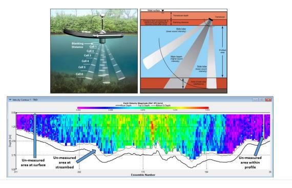
**Figure 32.** Unmeasured areas in the ADCP profile where velocity is extrapolated. Top left: ADCP blanking distance and cell size distribution (credit: SonTek); top right: unmeasured areas of the profile relative to ADCP beams (credit: SonTek); below: the WinRiver II velocity contour with unmeasured areas delineated.
