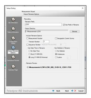
**Figure 22**. Required settings in the WinRiver II Output Filename Options dialogue box within the Measurement Wizard.
