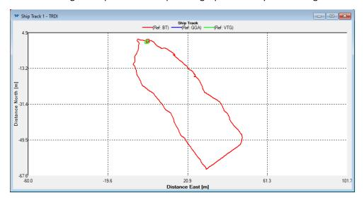
**Figure 69**. The WinRiver II Ship Track window observed during a loop moving bedtest. The green box indicates the boat starting position, the line shows the boat path as it is navigating across the channel and turned back around toward the starting bank, and the red box indicates the boat ending position.
