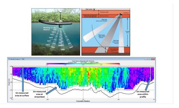
**Figure 74**. Unmeasured areas in the ADCP profile where velocity is extrapolated. Top left: ADCP blanking distance and cell size distribution (credit: SonTek); top right: unmeasured areas of the profile relative to ADCP beams (credit: SonTek); below: the WinRiver II velocity contour with unmeasured areas delineated.
