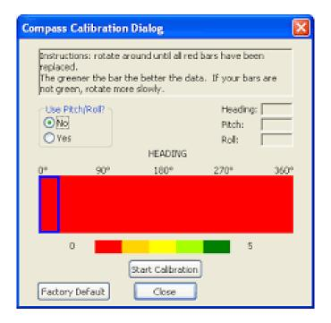
**Figure 68**. ADCP Compass Calibration dialog box. The entirety of the horizontal bar is red upon initiating the test. Rotate the boat slowly and steadily so that bar is colored dark green throughout.
