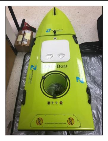
Figure 37. The ARC-Boat is the preferred deployment method to measure discharge at NEON river sites.
