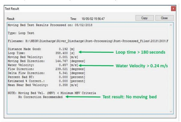
**Figure 54**. Moving Bed Loop Test Result window. In this example the required conditions were met in order to evaluate a moving bed (Loop time, water velocity) and a moving bed was not detected (the moving bed velocity < the moving bed velocity criteria), thus no correction was recommended.
