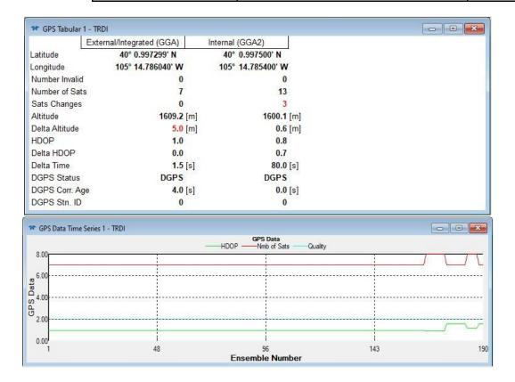
**Figure 23**. Above: GPS Tabular window that confirms GPS data is available and is being collected; Below: GPS Time Series window that indicates GPS data is streaming.
