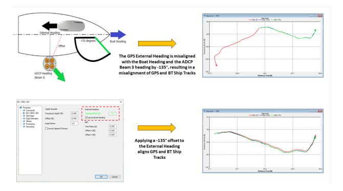
Figure 41. Applying External Heading offsets to align GPS and Bottom Track Ship Tracks.
