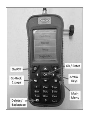
Figure 11. HACH FH950 flowmeter with displayed Start menu.
