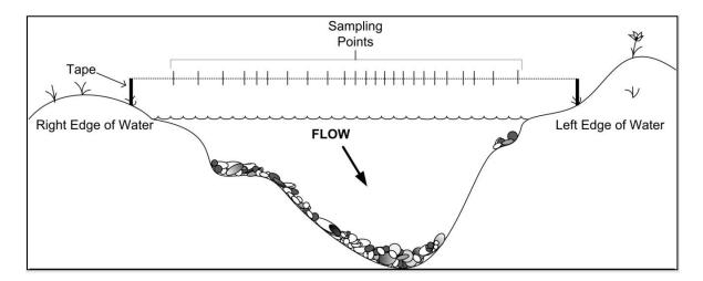
**Figure 13**. Example of uneven station spacing across a discharge transect at a wadable stream site using the Flowmeter Method. Note that non-laminar flow is assumed in this example.
