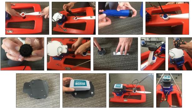
Figure 15. Above: Trimaran float, StreamPro ADCP, and SX Blue II GPS antenna components; Below: Illustrated workflow (top left to bottom right) detailing how to configure the StreamPro ADCP unit and SX Blue II GPS antenna to the trimaran float.
