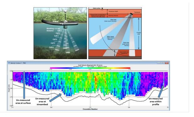
**Figure 57**. Unmeasured areas in the ADCP profile where velocity is extrapolated. Top left: ADCP blanking distance and cell size distribution (credit: SonTek); top right: unmeasured areas of the profile relative to ADCP beams (credit: SonTek); below: the WinRiver II velocity contour with unmeasured areas delineated.
