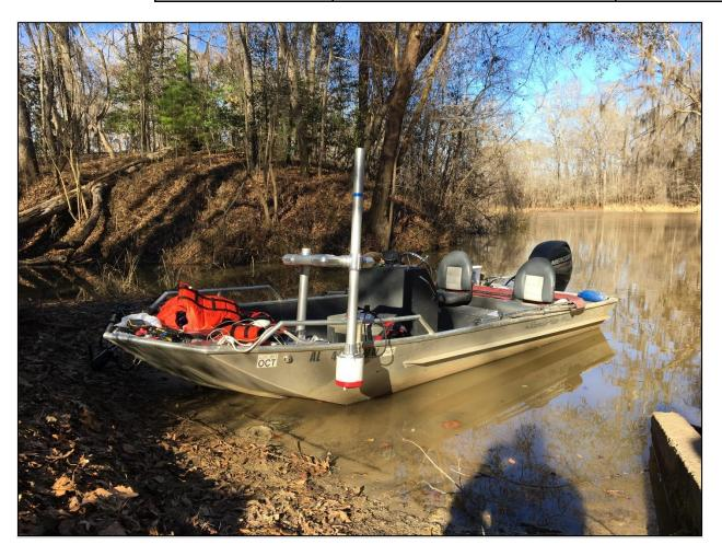
Figure 62. The Kentucky II mount (USGS) is used to deploy the ADCP when measuring discharge at NEON river sites using the piloted boat method.
