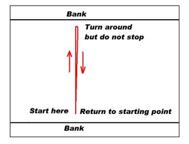
Figure 52. Illustration of the Loop Moving Bed Test procedure.
