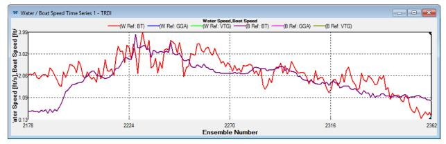
**Figure 33**. Water Speed vs. Boat Speed graph. Above: Improper technique. The boat speed (purple line) is erratic and higher than the water velocity (red line). Below: Proper technique. Maintain an even boat speed so that the purple and red lines are more in line and boat speed remains generally lower than water speed.
