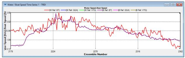
**Figure 58**. Water Speed vs. Boat Speed graph. Above: Improper technique. The boat speed (purple line) is erratic and higher than the water velocity (red line). Below: Proper technique. Maintain an even boat speed so that the purple and red lines are more in line and boat speed remains generally lower than water speed.
