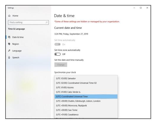
**Figure 46**. Set the PC used for the discharge measurement to (UTC) Coordinated Universal Time and match the ADCP clock to this setting.
