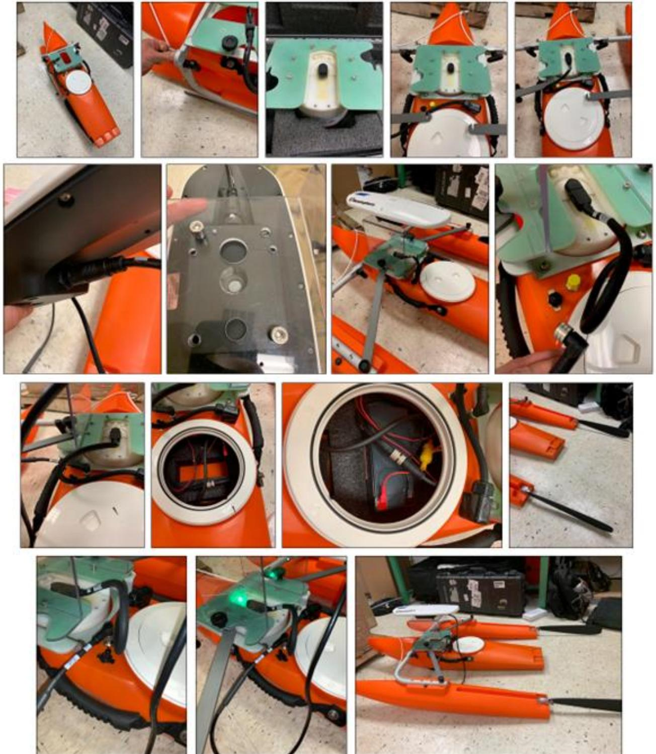
**Figure 10.** Illustrated workflow (top left to bottom right) detailing how to assemble the RiverPro ADCP unit and the Hemisphere GPS antenna onto the trimaran float.
