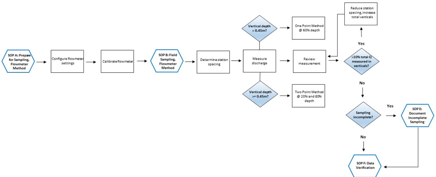
Figure 6. A detailed workflow diagram that visually shows the workflow for wadable stream sites using the flowmeter method.
