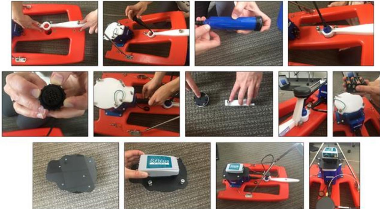
**Figure 9.** Above: Trimaran float, StreamPro ADCP, and SX Blue II GPS antenna components; Below: Illustrated workflow (top left to bottom right) detailing how to assemble the StreamPro ADCP unit and SX Blue II GPS antenna onto the trimaran float.
