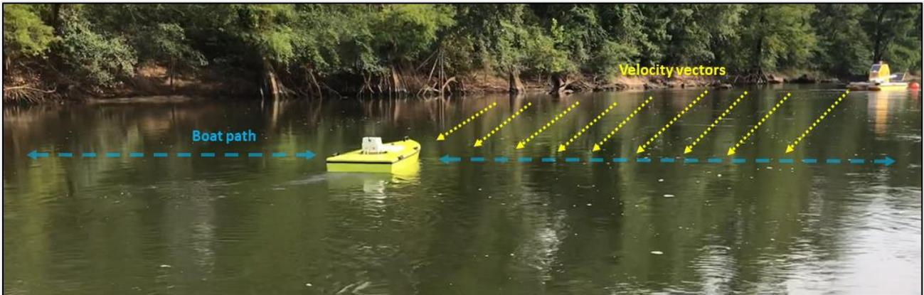
**Figure 19.** When surface water velocity is sufficiently high, operate the ARC-Boat in such a way that the bow is pointed into the velocity vectors and the boat is crabbed across the channel.
