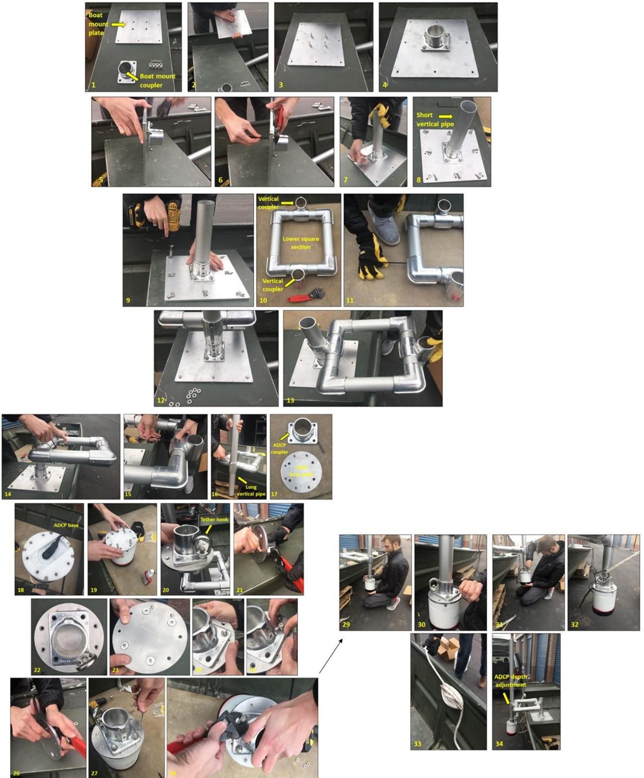
Figure 22. Assembling the ADCP mount on a piloted boat.
