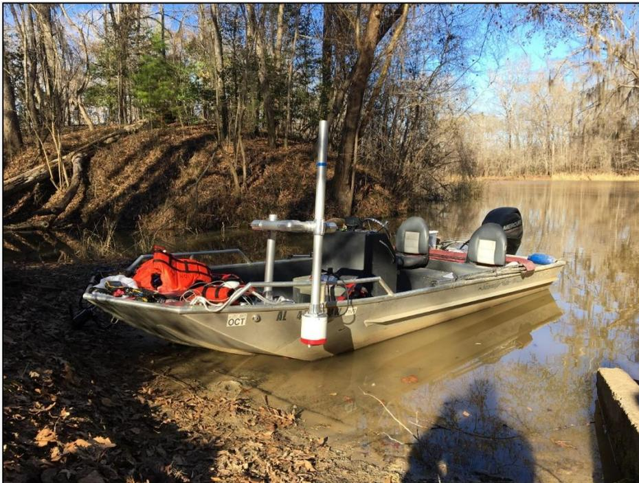
**Figure 21.** The ADCP mount deploys the ADCP off the side of a piloted boat.
