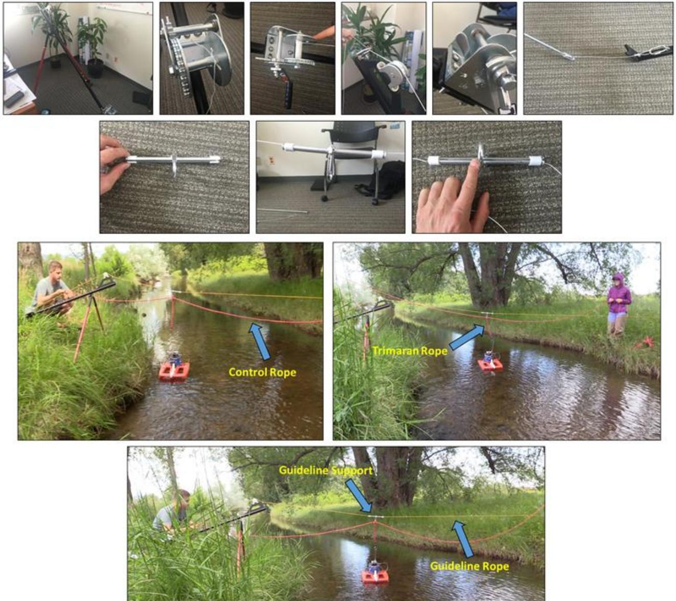
Figure 14. Installing the High Line Assembly.
