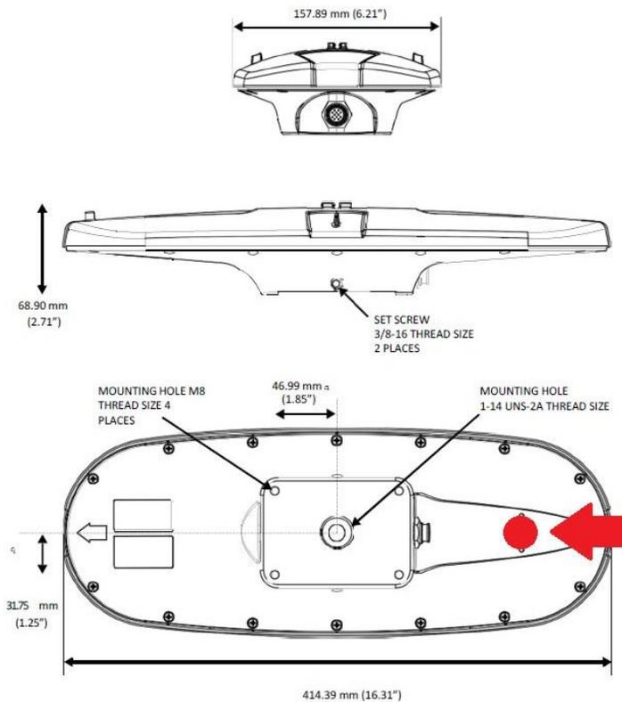
**Figure 17.** Hemisphere V102 GPS antenna schematics. Top: the back of the unit with cable port show; Middle: the side of the unit showing one of two set screw locations; Bottom: the base of the unit, the red circle to the right of the unit indicates the location that must be centered over the ADCP, the white arrow to the left of the unit indicates the direction the unit must face so that it is oriented toward Beam 3 of the ADCP.
