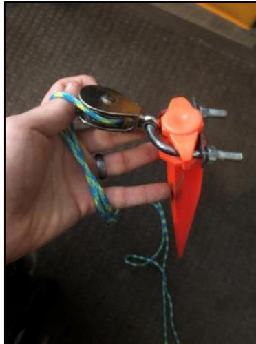
**Figure 11.** U-Bolt/Fixed Pully configuration used for the Pully Assembly trimaran float deployments. This example the U-Bolt is placed over a snow stake, rather than a post or unistrut.
