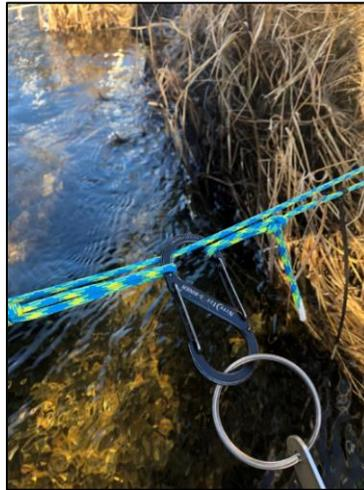
**Figure 12.** Paracord/S-Biner Carabiner/float ringer connection used for the Pulley Assembly during trimaran float deployments.
