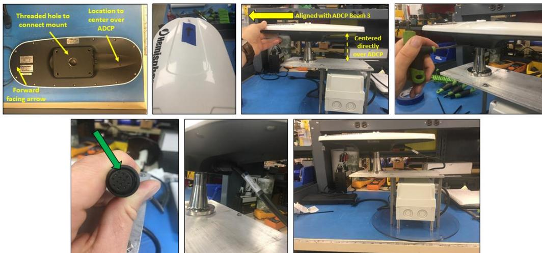
**Figure 16.** Installing the Hemisphere V102 GPS antenna onto the ARC-Boat GPS mount.
