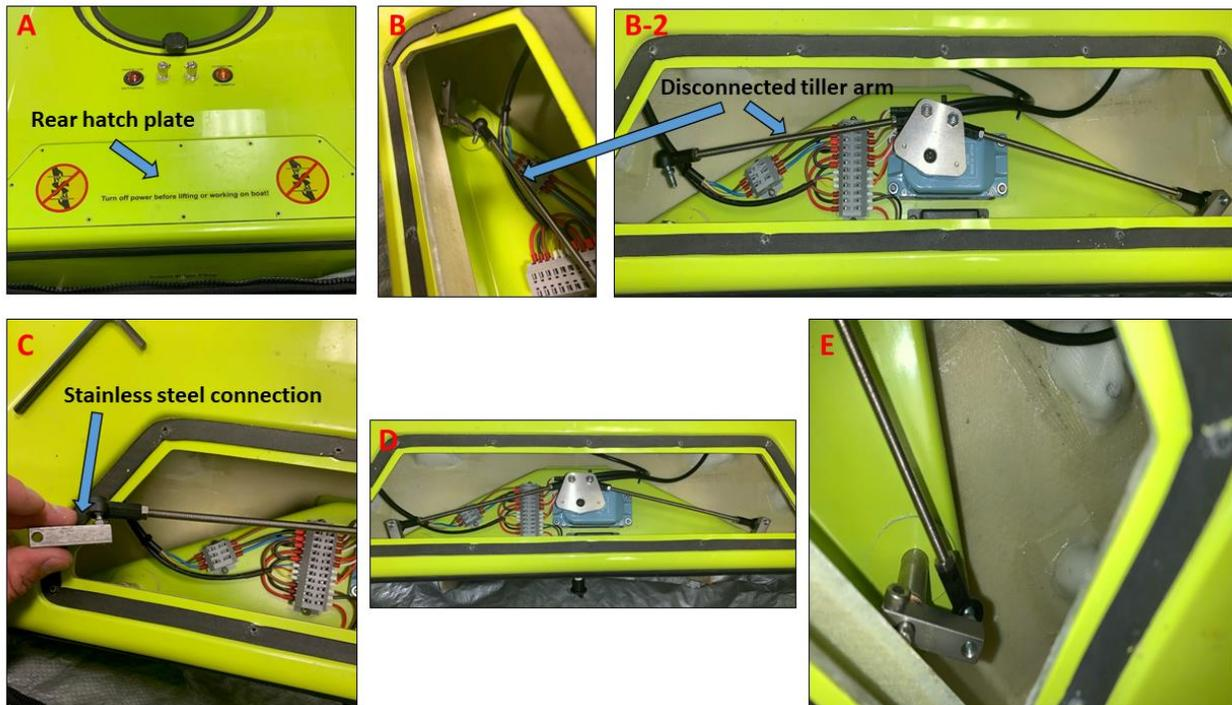
**Figure 8.** Repairing a disconnected tiller on the ARC-Boat.
