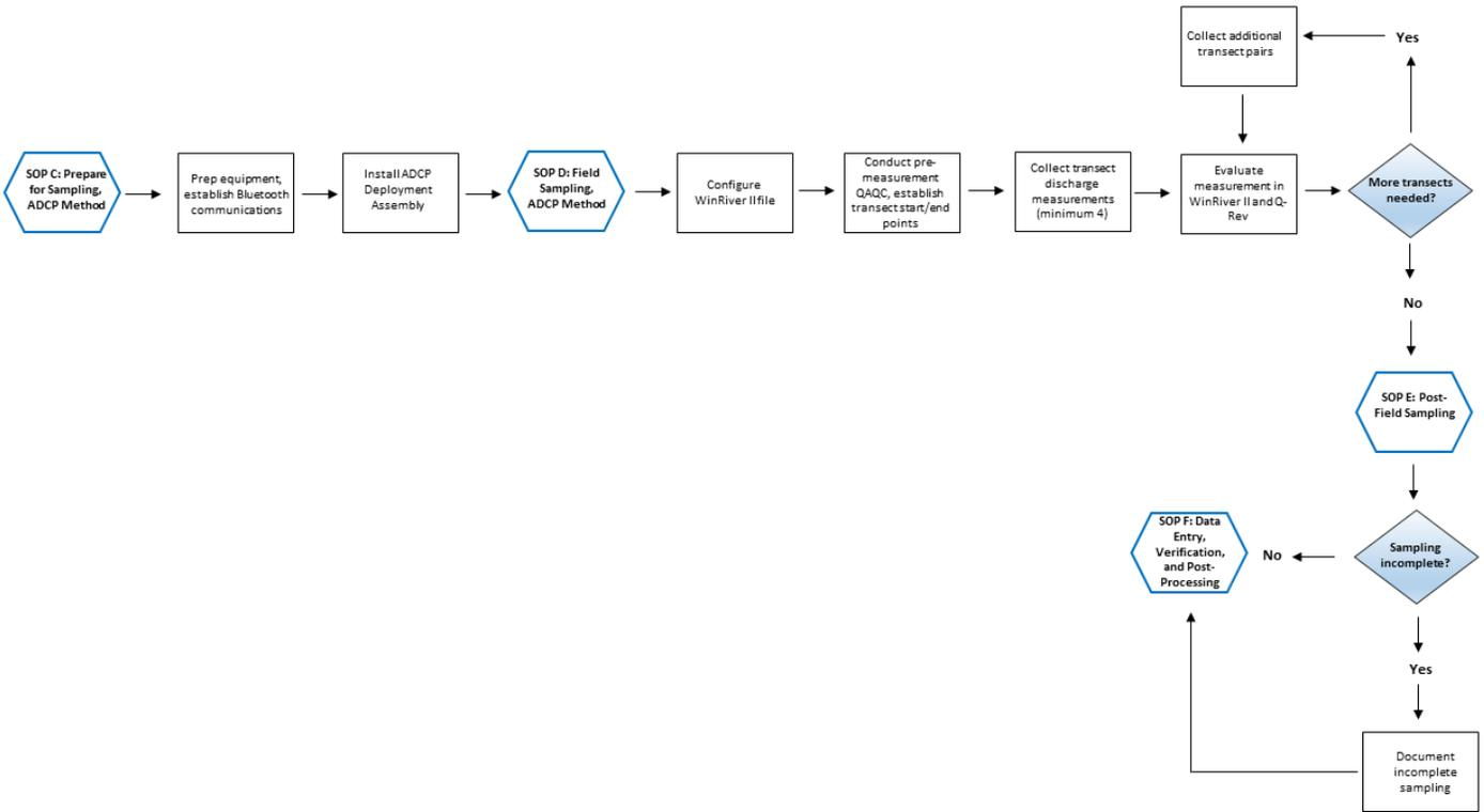
**Figure 7.** A detailed workflow diagram that visually shows the workflow for wadable stream and river sites using the ADCP method.
