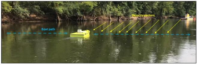
**Figure 19**. When surface water velocity is sufficiently high, operate the ARC-Boat in such a way that the bow is pointed into the velocity vectors and the boat is crabbed across the channel.
