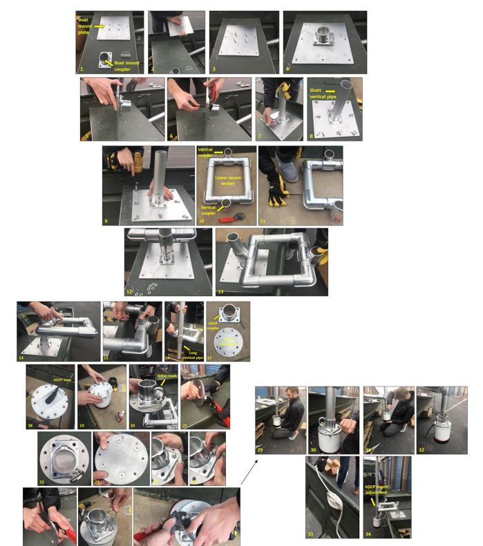
Figure 22. Assembling the ADCP mount on a piloted boat.
