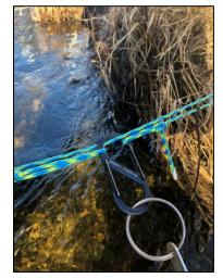
**Figure 12**. Paracord/S-Biner Carabiner/float ringer connection used for the Pulley Assembly during trimaran float deployments.
