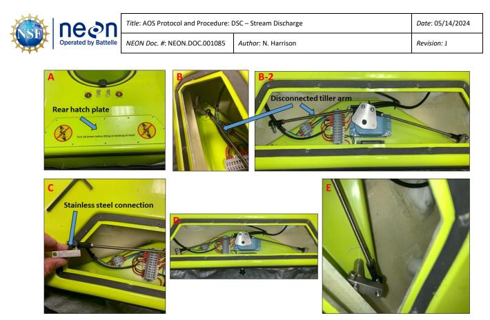
Figure 8. Repairing a disconnected tiller on the ARC-Boat.
