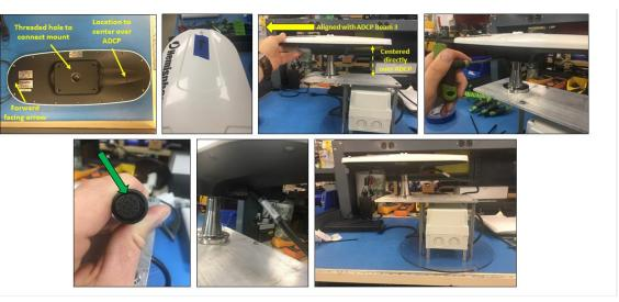
Figure 16. Installing the Hemisphere V102 GPS antenna onto the ARC-Boat GPS mount.
