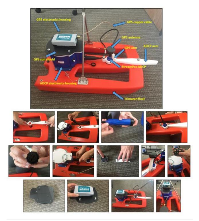
**Figure 9**. Above: Trimaran float, StreamPro ADCP, and SX Blue II GPS antenna components; Below: Illustrated workflow (top left to bottom right) detailing how to assemble the StreamPro ADCP unit and SX Blue II GPS antenna onto the trimaran float.
