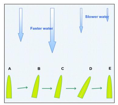
**Figure 20**. Illustration of different ways to control the ARC-Boat in a variety of streamflow regimes. See **Table 11** for corresponding controller tips.
