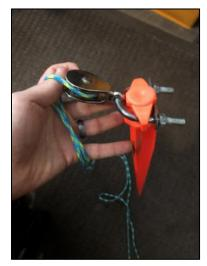
**Figure 11**. U-Bolt/Fixed Pully configuration used for the Pully Assembly trimaran float deployments. This example the U-Bolt is placed over a snow stake, rather than a post or unistrut.
