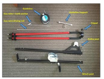
Figure 13. Materials included with the High Line Assembly kit.
