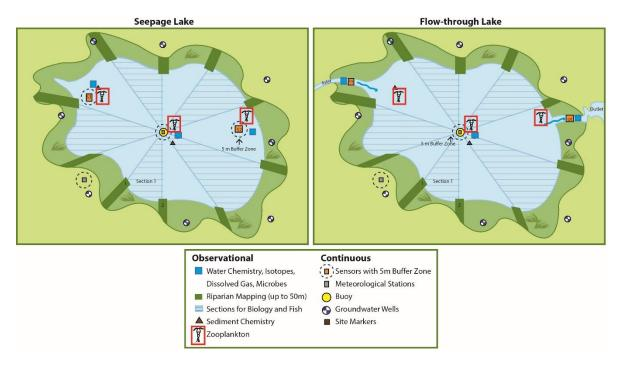
**Figure 3.** A generic lake site layout with zooplankton sampling locations. Seepage lakes have no true inlet or outlet stream. In flow-through streams, inlet and outlet infrastructure are located in the inlet or outlet stream channel.
