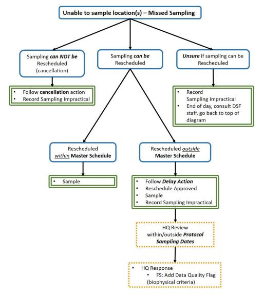
**Figure 4**. The documentation to account for a Missed Sampling event depends on the situation for each plot of each bout that is not sampled. Blue rounded boxes represent contingencies, green double line boxes describe the required actions, Orange dotted boxes indicate HQ actions. Required delay and cancellation actions are outlined for each protocol in the 'Scheduled Field Activities – Delays and Cancellations' spreadsheet available on the SSL.
