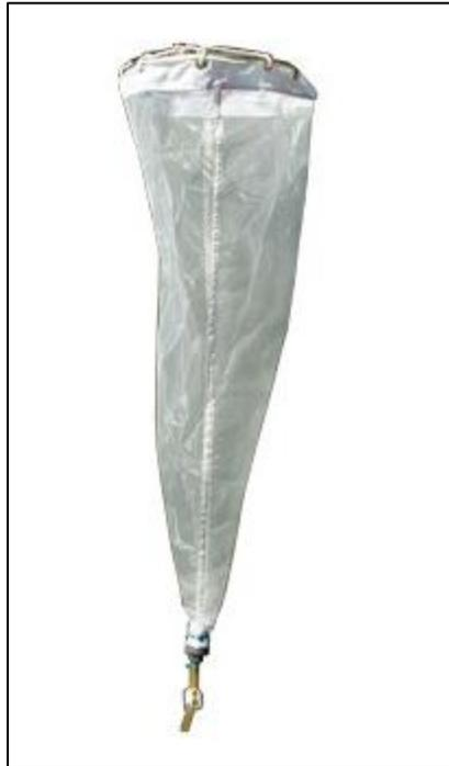
**Figure 13.** Zooplankton tow net with bottom tubing and clamp.
