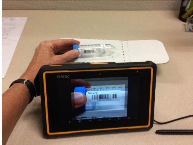
Figure 11. Barcode label scanning.
