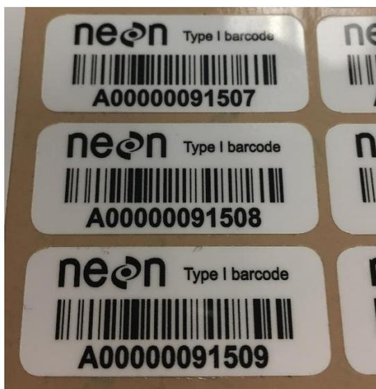
Figure 8. Example of adhesive barcode labels, Type I. These large-size, field-tolerant barcodes have a prefix of 'A' followed by 11 numbers.
