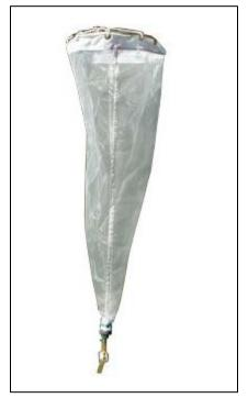
Figure 13. Zooplankton tow net with bottom tubing and clamp.
