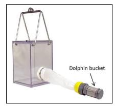
**Figure 10.** Example of a Schindler-Patalas sampler with Dolphin bucket.
