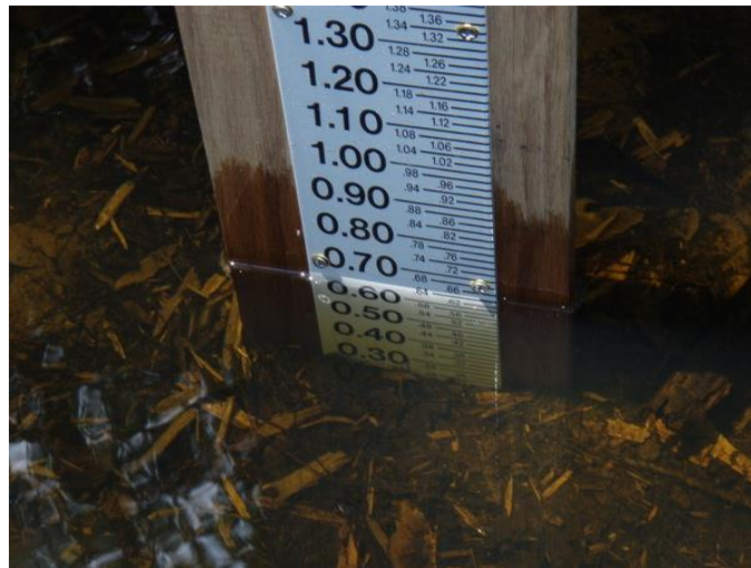
Figure 11. Example of a staff gauge. If conditions are wavy, note the mean height.
