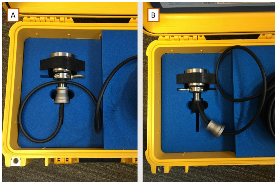
Figure 3. 0.5” to 0.75” reducer attached (panel A) and removed (panel B) to the sonar transducer.
