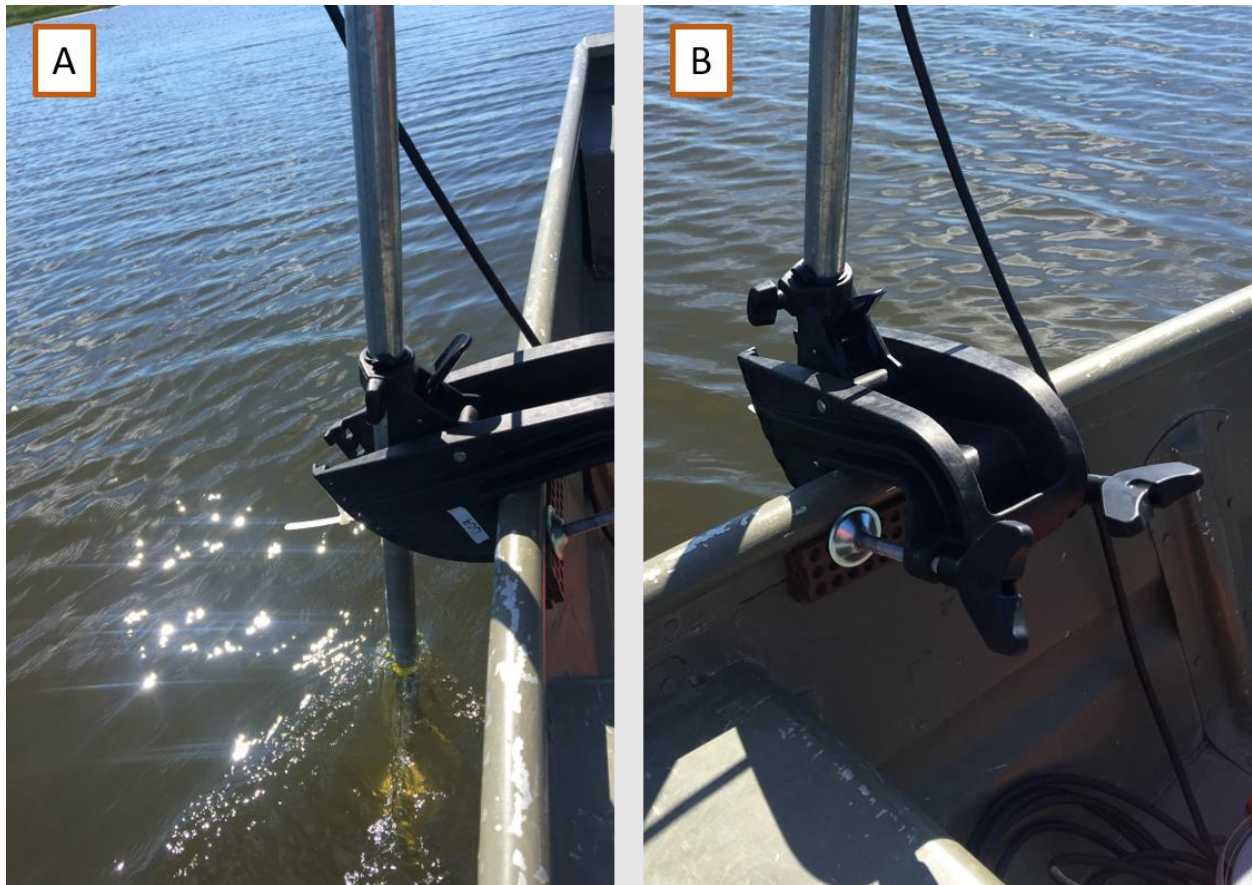
Figure 5. Example of pipe and trolling motor mount with transducer submerged (panel A). Shims used to make the mount more stable can be seen in panel B. The cable is fed out through the top of the pipe to be connected to the Biosonics case that contains the GPS receiver and power supply.
