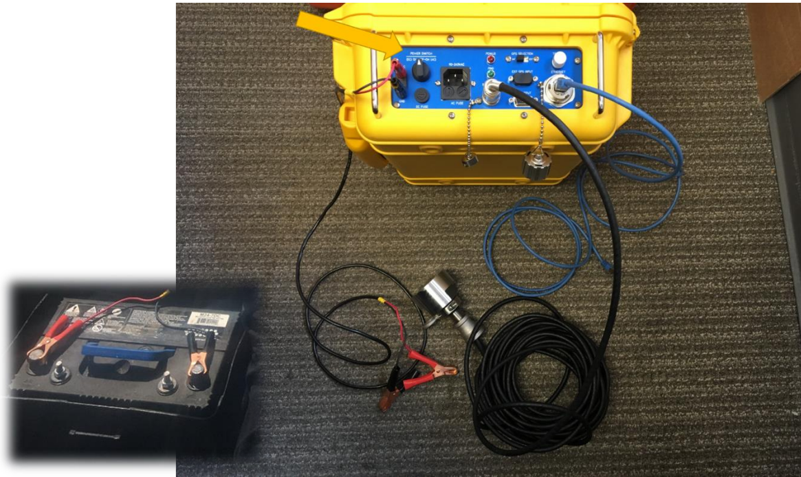
Figure 7. Example photo of all cables plugged into the case. Arrow points at the power switch that should be turned off until you’re ready to collect data. Alligator clips should be connected to a 12V DC deep cycle battery. The sonar unit should be installed on the boat mount prior to connecting to the case.
