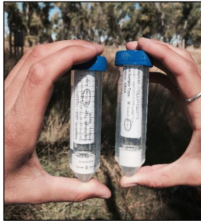
Figure 18. Dissolved gas samples stored upside-down in centrifuge tubes.
