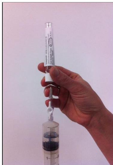
Figure 16. Transfer of dissolved gases to an evacuated gas vial.
