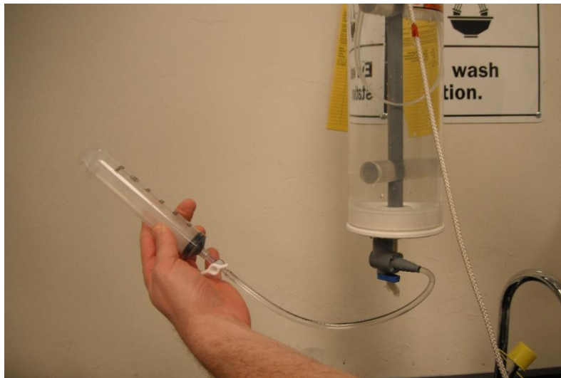
Figure 12. Syringe and 2-way stopcock attached to Kemmerer spigot.
