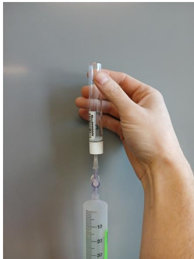
Figure 16. Transfer of dissolved gases to an evacuated gas vial.
