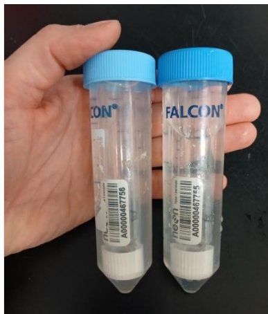
Figure 20. Dissolved gas samples stored upside-down in centrifuge tubes.
