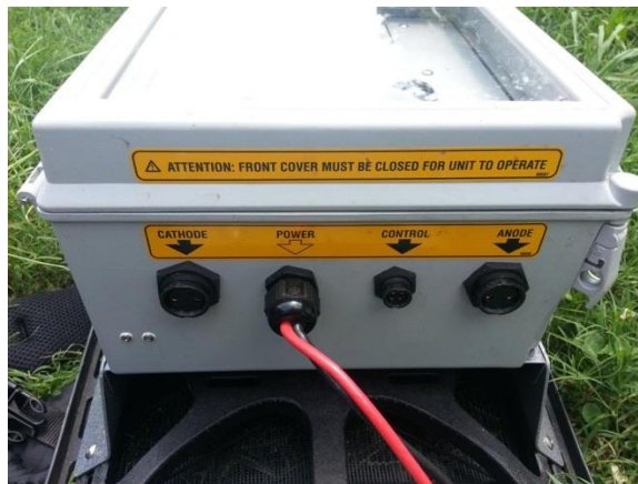
Figure 15. Cathode and anode connections on backpack electrofisher unit.
