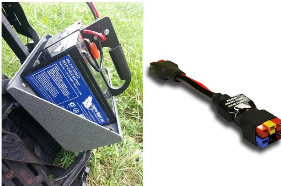
Figure 16. Left: Battery location and secure placement in the backpack electrofisher frame. Right: lithium-ion battery adapter.
