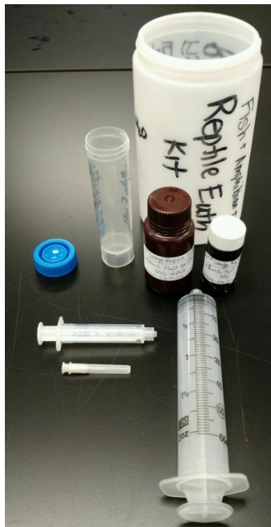
Figure 20. Reptile Euthanasia kit with 50 mL centrifuge tube to store the 5 mL syringe and needle, 60 mL HDPE amber bottle is for 1st stage solution, 20 mL HDPE scintillation vial for 2nd stage solution.
