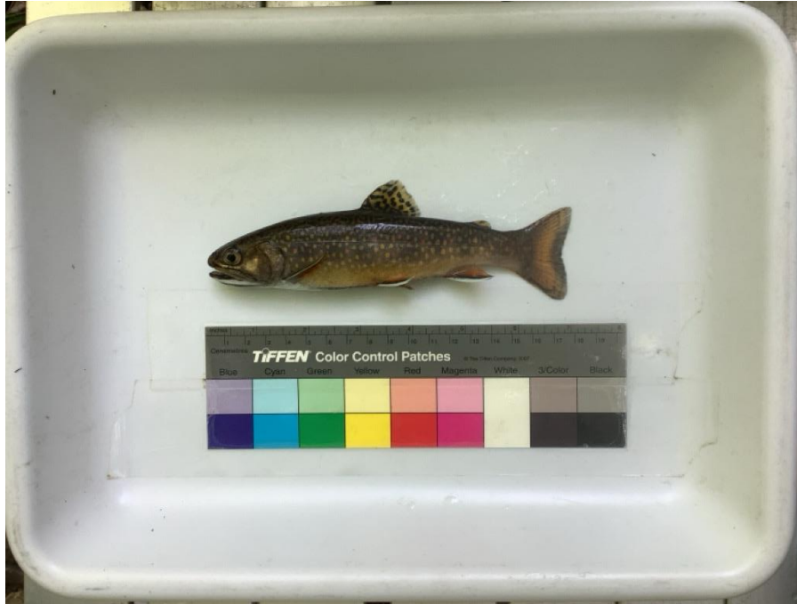
Figure 23. Example voucher photo. Lateral, head left, with color separation guide and scale bar. Photo from OSU 2017.
