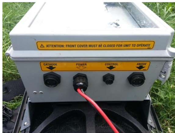
Figure 13. Cathode and anode connections on backpack electrofishing unit.
