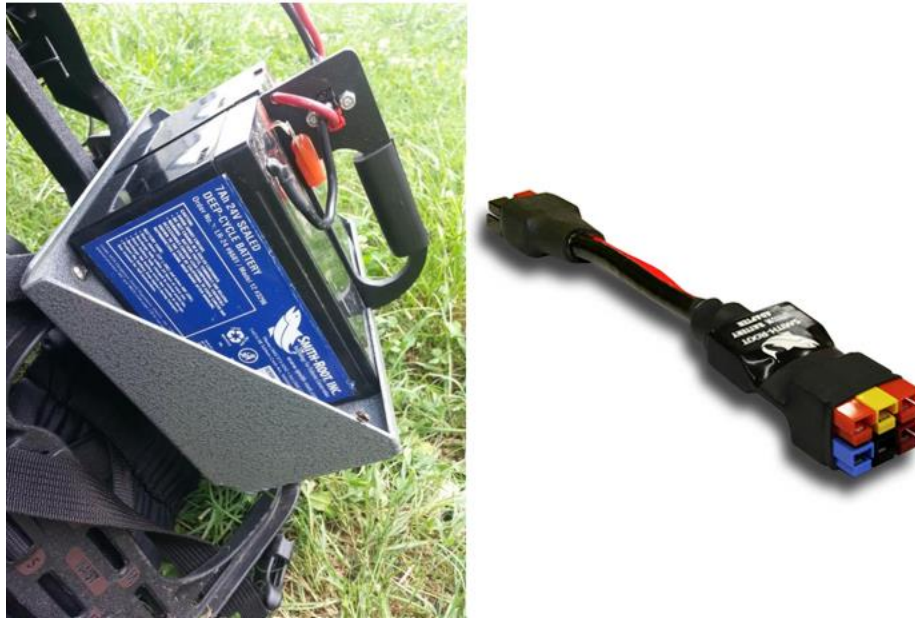
Figure 14. Left: Battery location and secure placement in the backpack electrofishing frame. Right: lithium-ion battery adapter.
