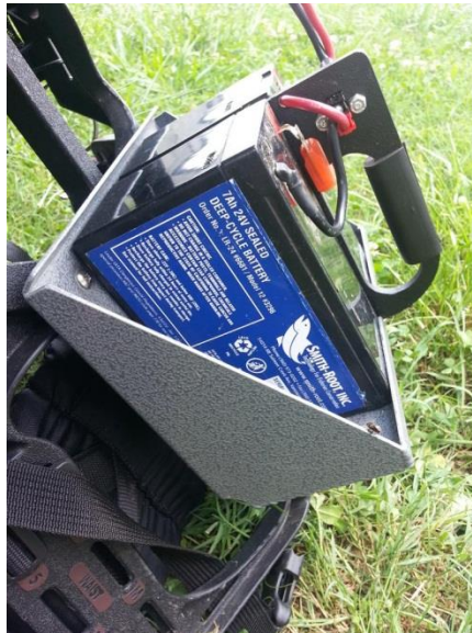
Figure 12. Battery location and secure placement in the backpack electrofishing frame.
