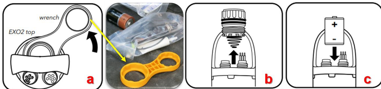
Figure 35. How to Replace Multisonde Internal D-Cell Batteries
