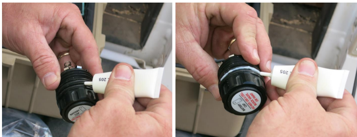
Figure 36. Lubricate Battery Cap with Krytox Grease
