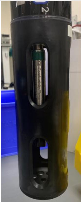
Figure 92. Multisonde Black Plastic Guard for Calibration of Optical Sensors
