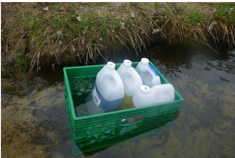
Figure 118. pH Buffer Solutions in Stream
