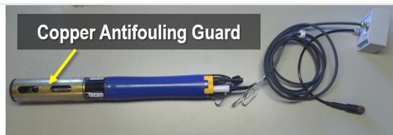
Figure 65. Antifouling Guard on Multisonde
