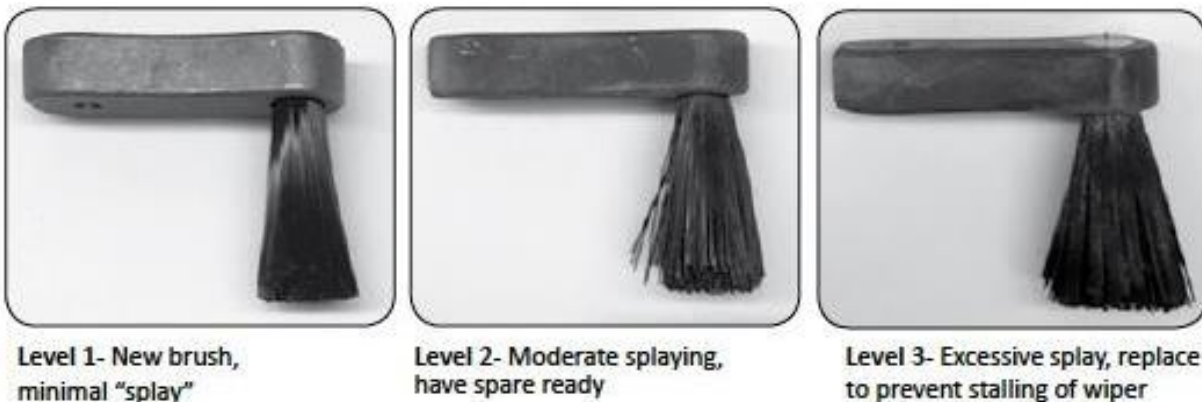
Figure 25. Multisonde Anti-Fouling Wiper: Levels of Wear over Time
