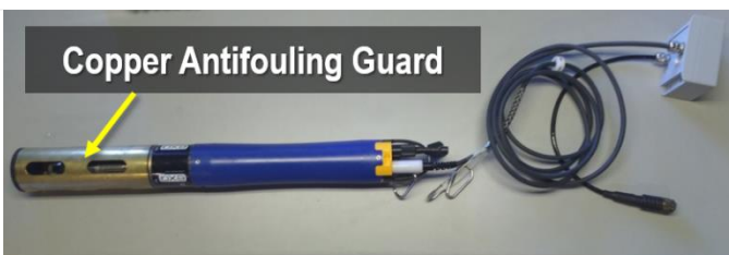
Figure 21. Location of Antifouling Guard
