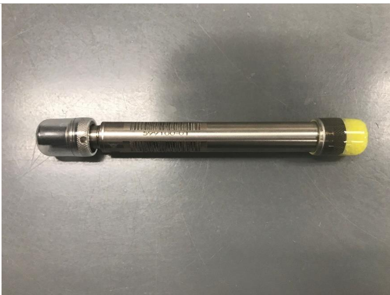
Figure 151. DO Sensor Probe Shipping Requirements
