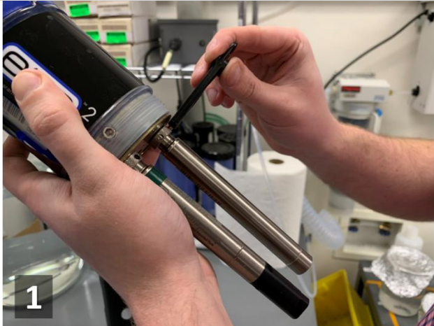
Figure 141. Use the Multisonde Probe Tool to Remove each Sensor Probe from the Multisonde
