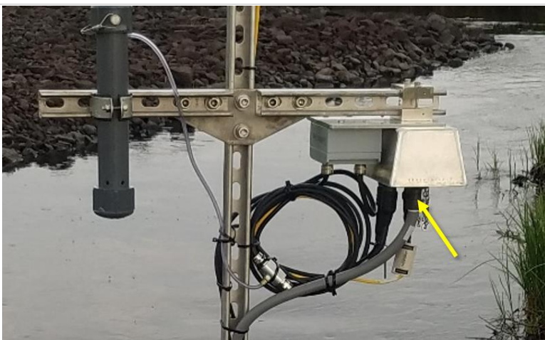
Figure 48. Merlot Grape with Signal Output Adapter (Splitter/Converter Box)
