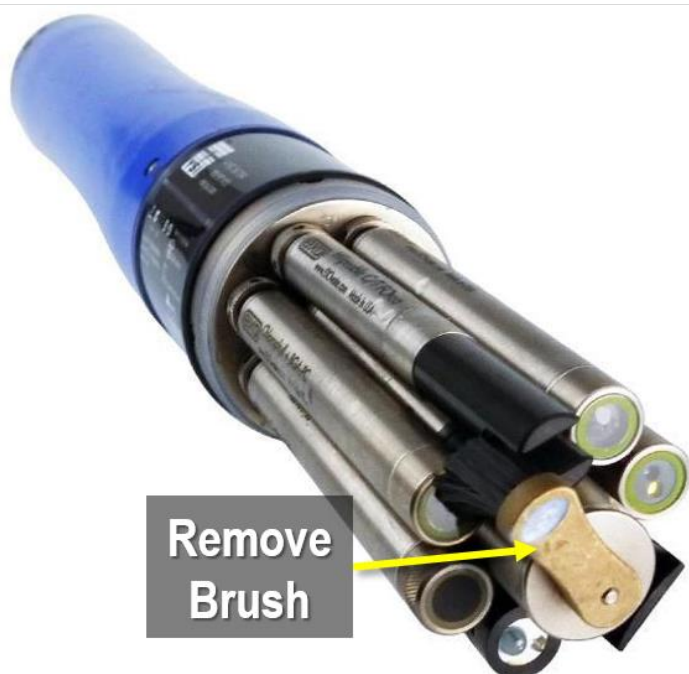
Figure 90. Remove Central Wiper Brush
