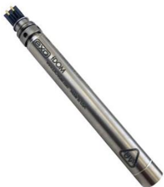
Figure 9. fDOM Probe Sensor
