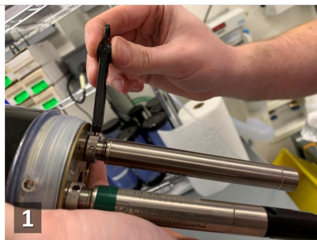
Figure 143. How to Reinstall a Sensor Probe
