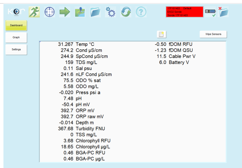
Figure 66. Capture a Pre-Cleaning Reading from Sensor Raw Data Output
