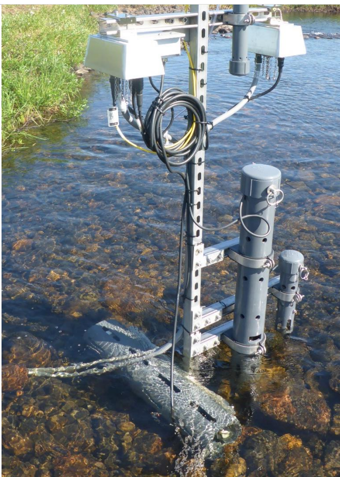
Figure 146. Multisonde Cable Dressing - Complete Installation
