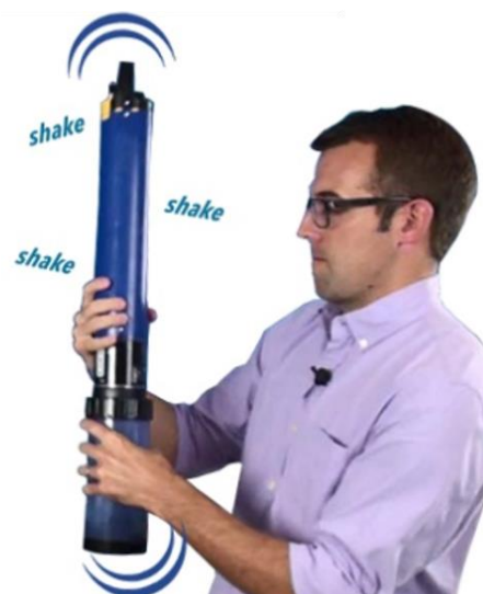
Figure 91. Triple Rinse Sensors & Calibration Cup with DI Water (Source: ER [08] Slide 10)
