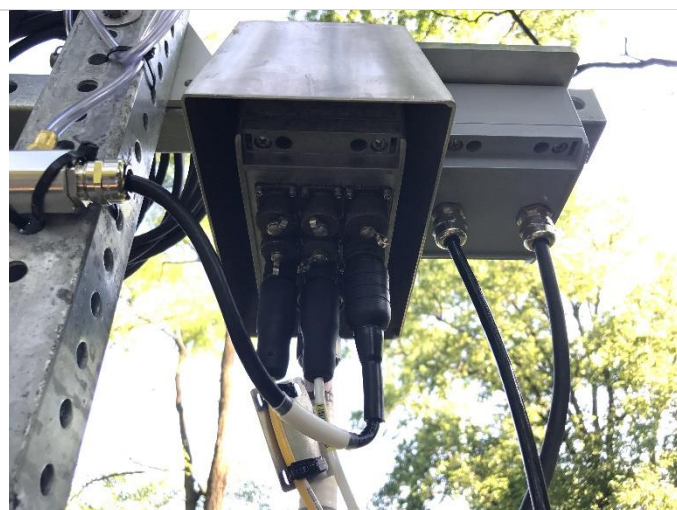
Figure 144. Reinstall the Multisonde Grape
