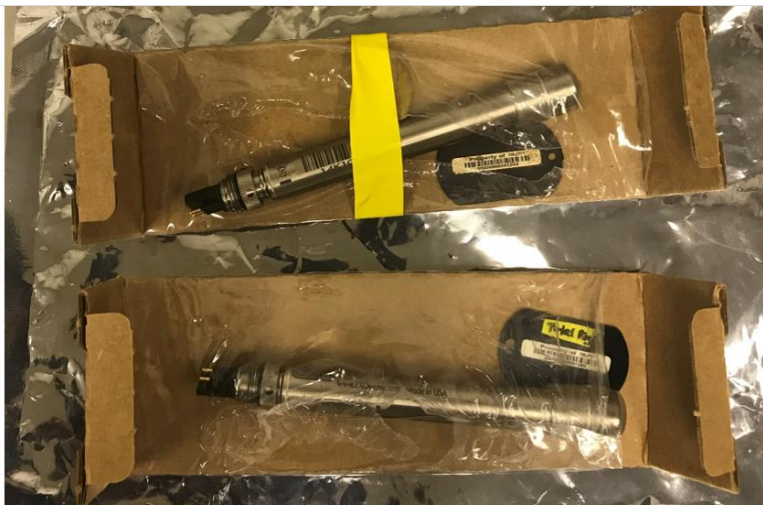
Figure 150. General Probe Sensor Packaging for Shipping/Handling
