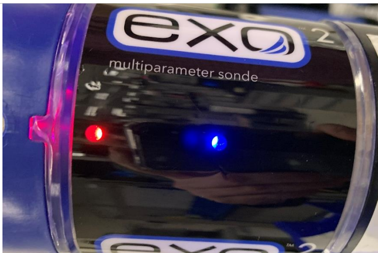
Figure 64. Example/Location of Bluetooth Blue LED
