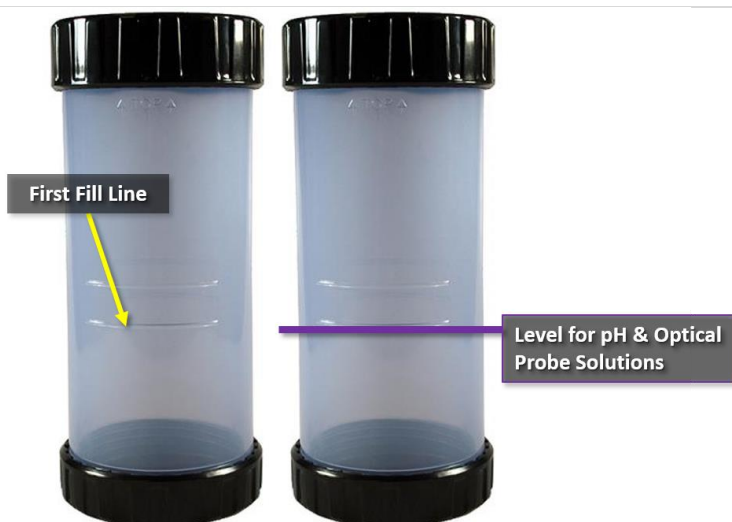
Figure 119. Fill the Calibration Cup with Buffer Solution to 1st Line
