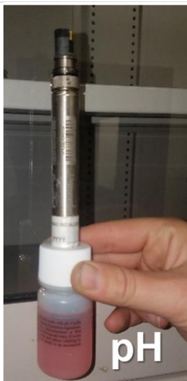
Figure 152. pH Probe Shipping Requirements
