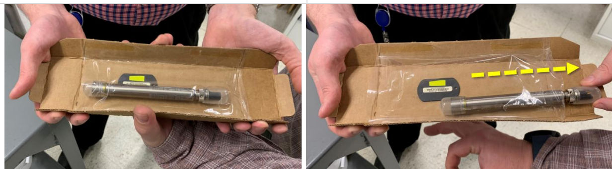
Figure 155. Move the Sides of the Insert up to Create Slack in Plastic Packaging to Remove Sensor and Asset Tag
