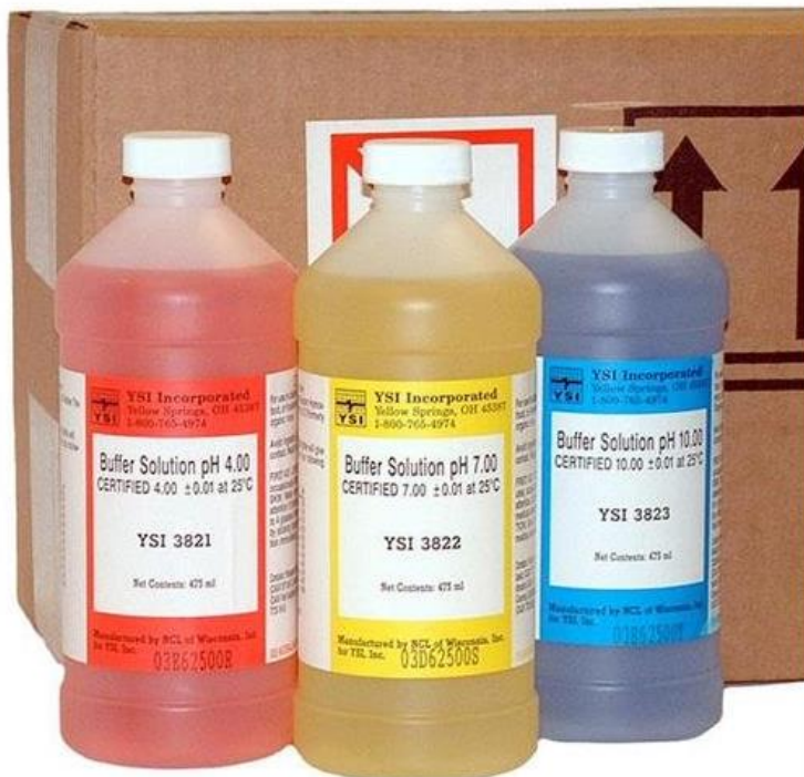
Figure 117. pH Probe Calibration Buffer Solutions
