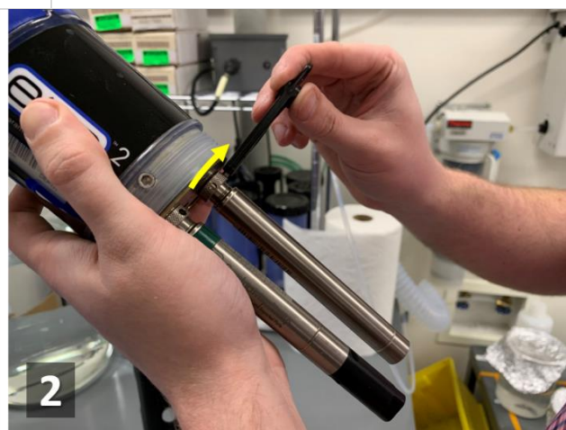
Figure 143. How to Reinstall a Sensor Probe
