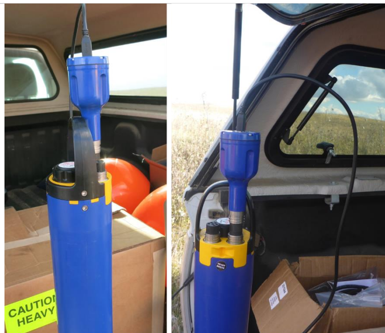
Figure 54. Complete Connection to Multisonde using a USB SOA
