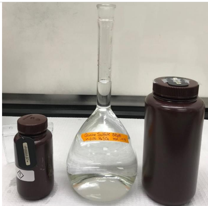
Figure 84. Prepared fDOM Calibration Solution with Amber/HDPE Bottles
