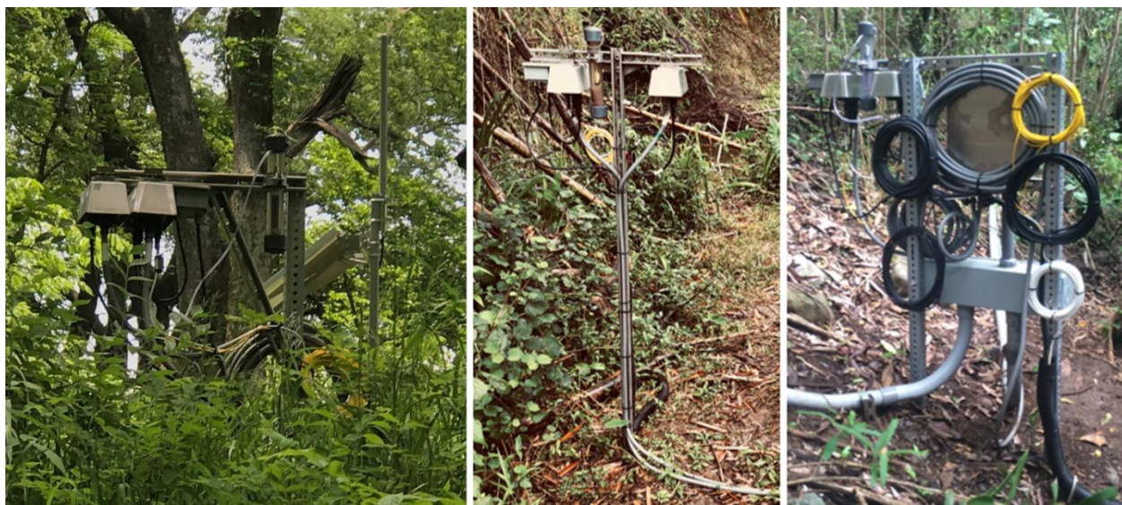
Figure 14. Stream Stand-Alone Arbors (left, middle) and Device Post Arbor (far right)
