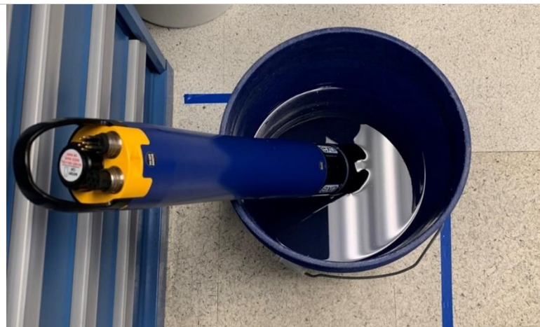
Figure 68. Capture Post-Clean Reading using Same Bucket of Water
