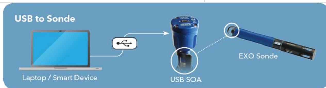
Figure 51. Connect to Multisonde using a USB SOA
