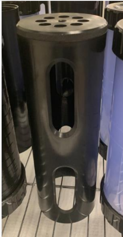
Figure 92. Multisonde Black Plastic Guard for Calibration of Optical Sensors
