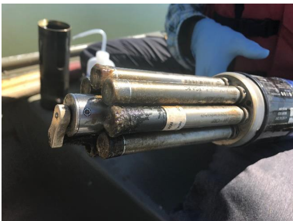
Figure 75. Example of Biofouling on Sensor Probes
