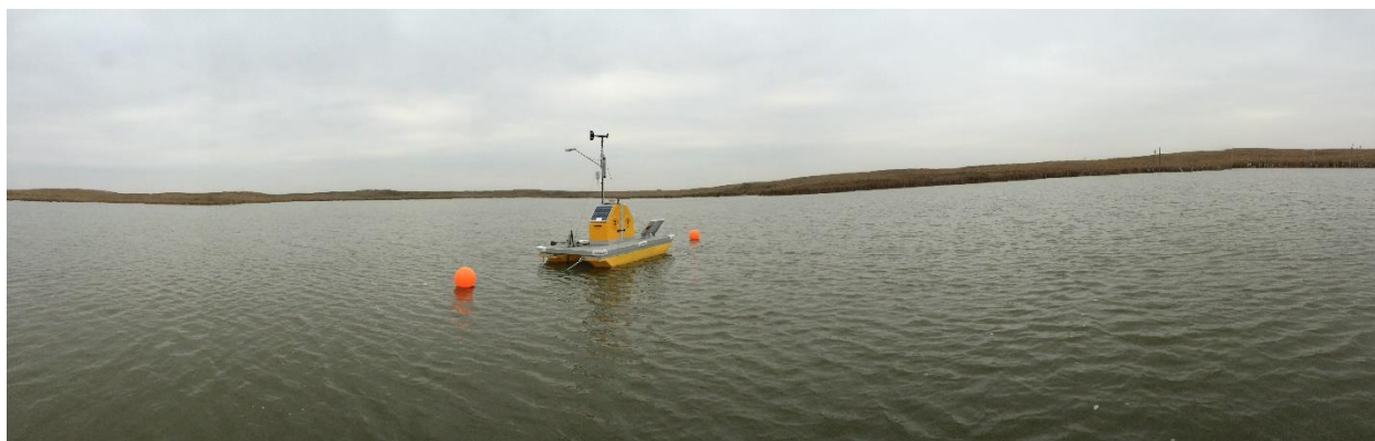
Figure 15. AIS Buoy for Lake and River Sites
