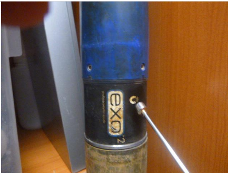
Figure 57. Wake up the Multisonde!
