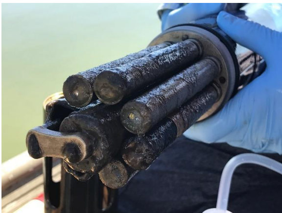
Figure 72. Example of Biofouling on Sensor Probes
