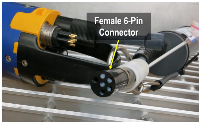
Figure 28. Greased Female 6-Pin Connector with Krytox
