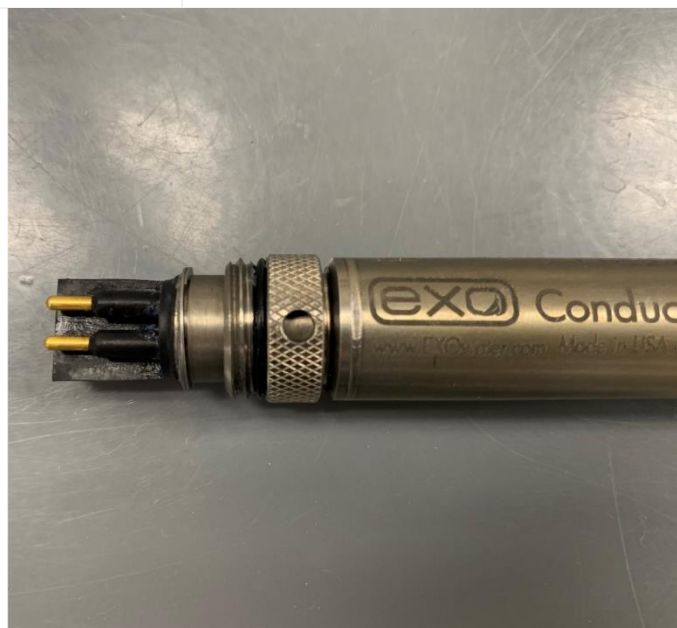
Figure 30. Sensor 4-Pin Connectors on Multisonde Body (Left) and Probe Sensor (Right)
