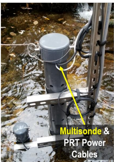
Figure 49. Disconnect the Black Power Cable
