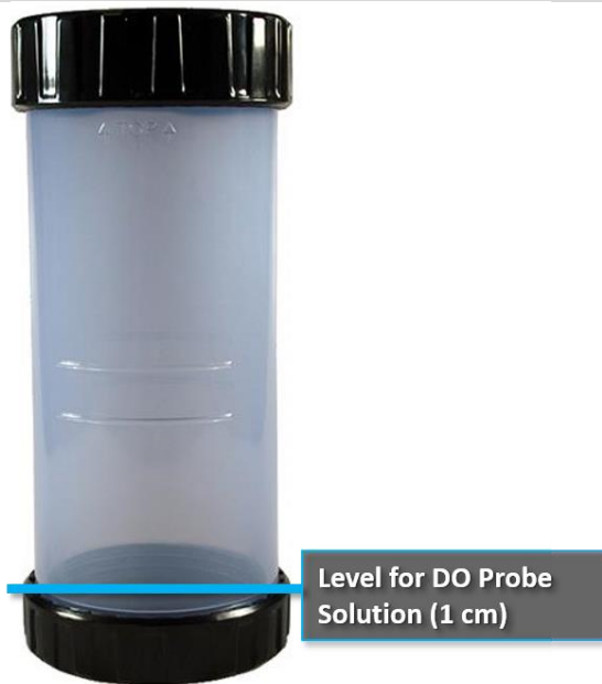
Figure 107. Fill Bottom of Calibration Cup with DI Water for DO Probe
