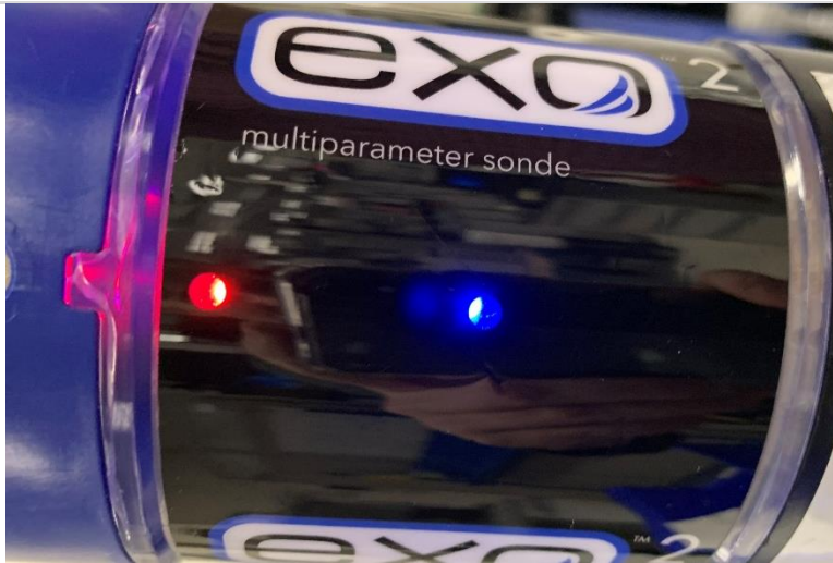
Figure 55. Example/Location of Bluetooth Blue LED
