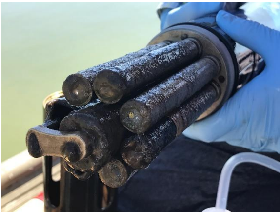
Figure 63. Example of Biofouling on Sensor Probes
