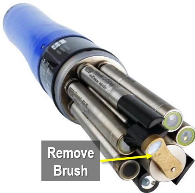
Figure 81. Remove Central Wiper Brush
