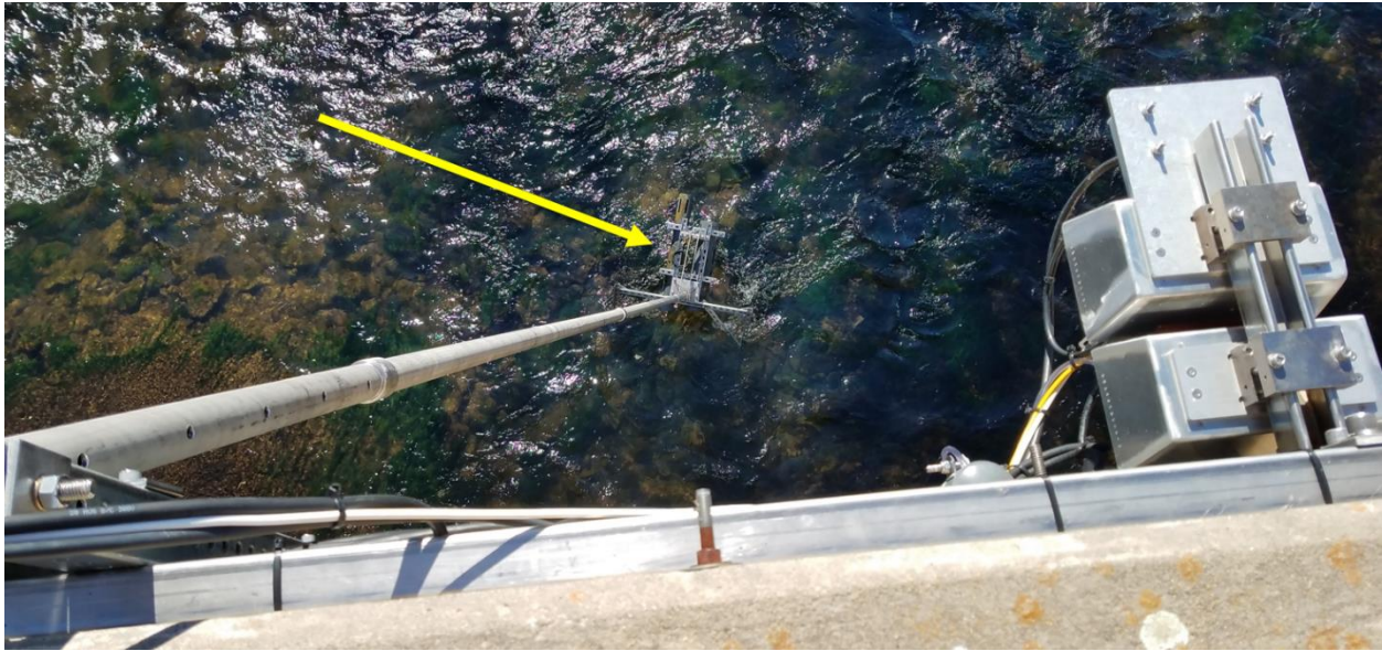
Figure 13. Domain 11, Southern Plains, BLUE Single Stream Sensor Set from Downrigger Mounting off Bridge
