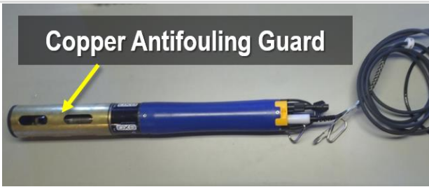
Figure 56. Antifouling Guard on Multisonde
