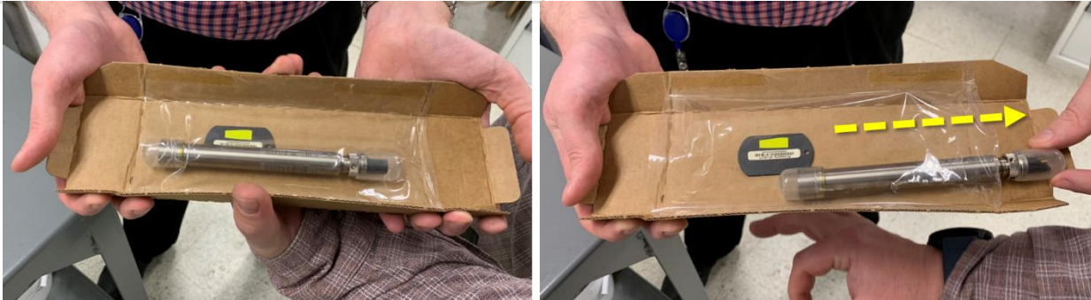
Figure 140. Move the Sides of the Insert up to Create Slack in Plastic Packaging to Remove Sensor and Asset Tag
