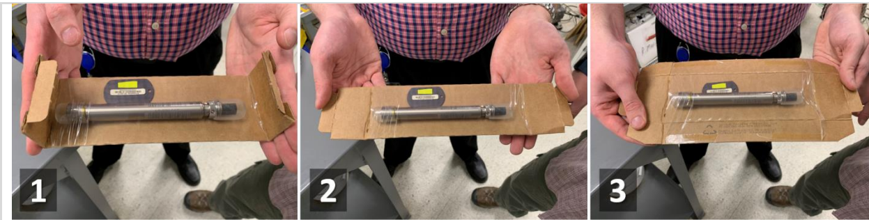
Figure 139. Remove the Sensor from the Box and Expand the Sides of the Cardboard Insert
