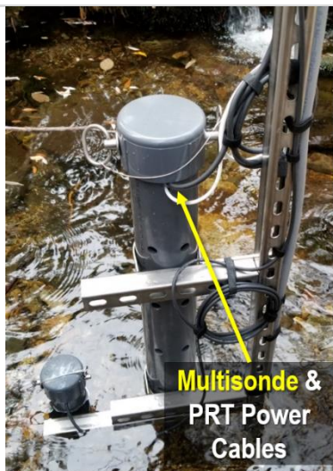
Figure 41. Disconnect the Black Power Cable
