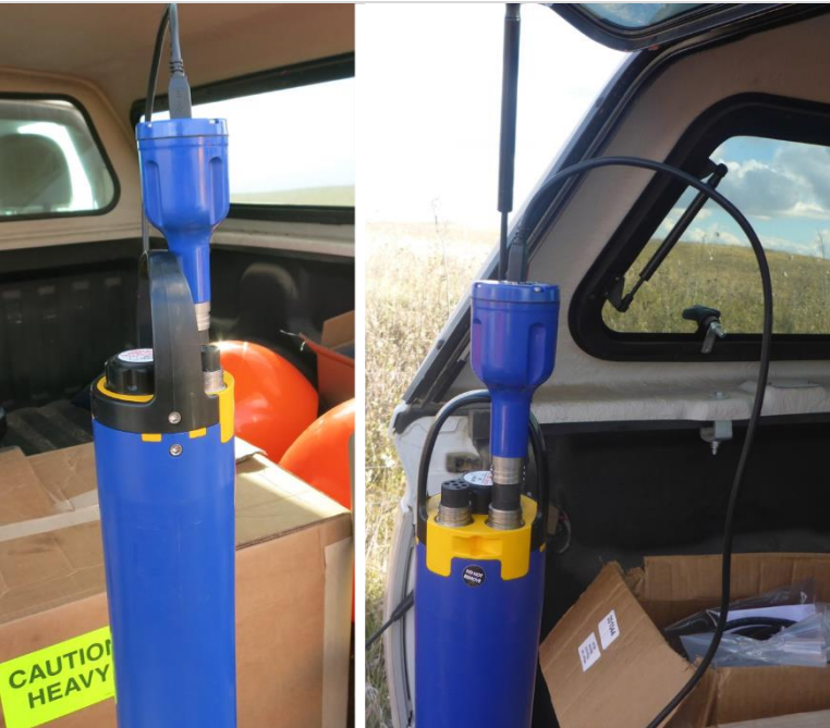
Figure 46. Complete Connection to Multisonde using a USB SOA
