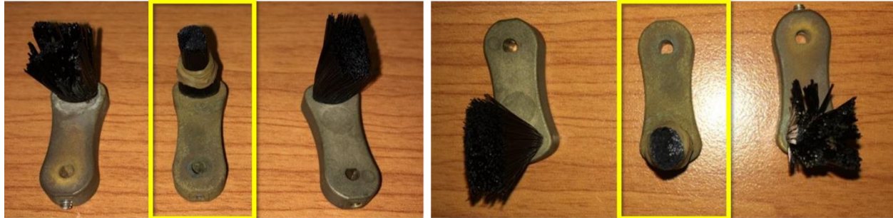
Figure 26. Use a Rubber Band to Control the Brush from Significant Splaying due to Turbulent Waterways
