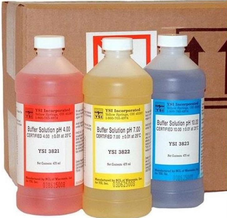
Figure 102. pH Probe Calibration Buffer Solutions
