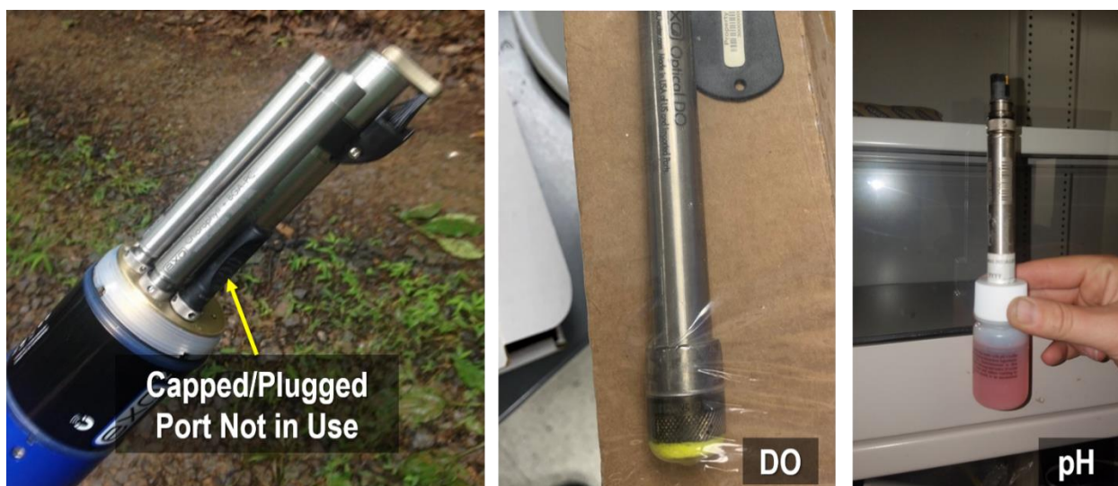
Figure 2. Example of a Plugged Port (Far Left) and Examples of the DO (Middle) and the pH Probe Caps (Far Right)
