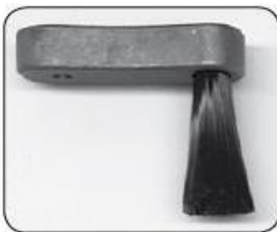
Level 1- New brush, minimal “splay”
