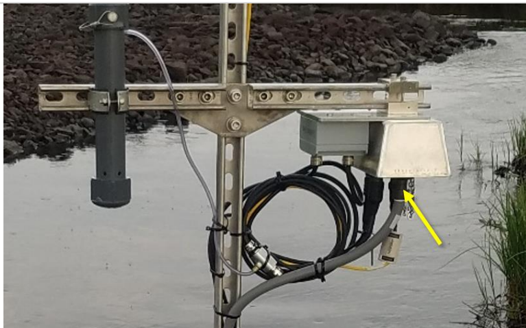
Figure 40. Merlot Grape with Signal Output Adapter (Splitter/Converter Box)
