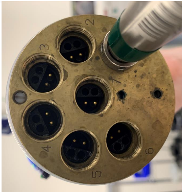
Figure 30. Sensor 4-Pin Connectors on Multisonde Body (Left) and Probe Sensor (Right)
