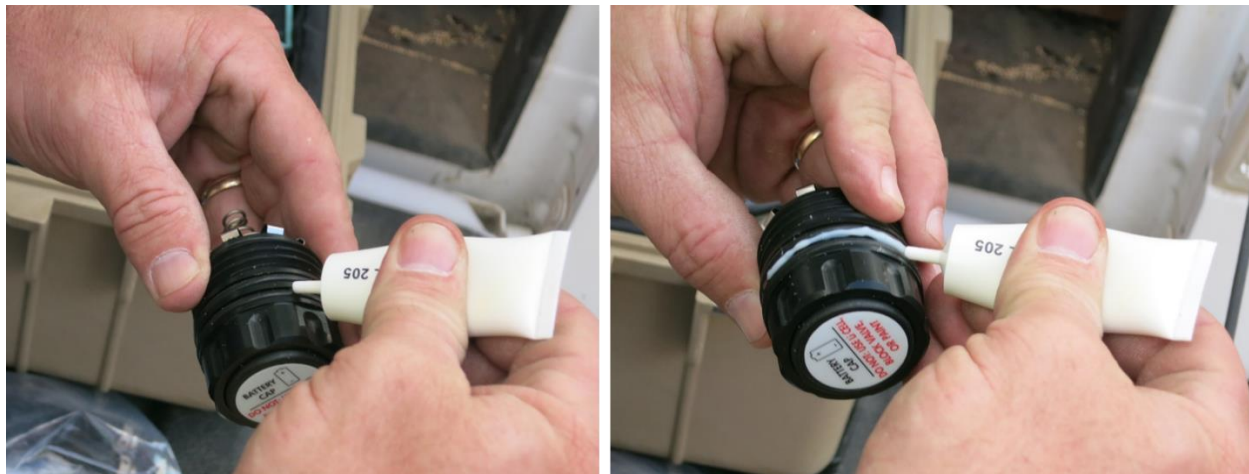
Figure 36. Lubricate Battery Cap with Krytox Grease
