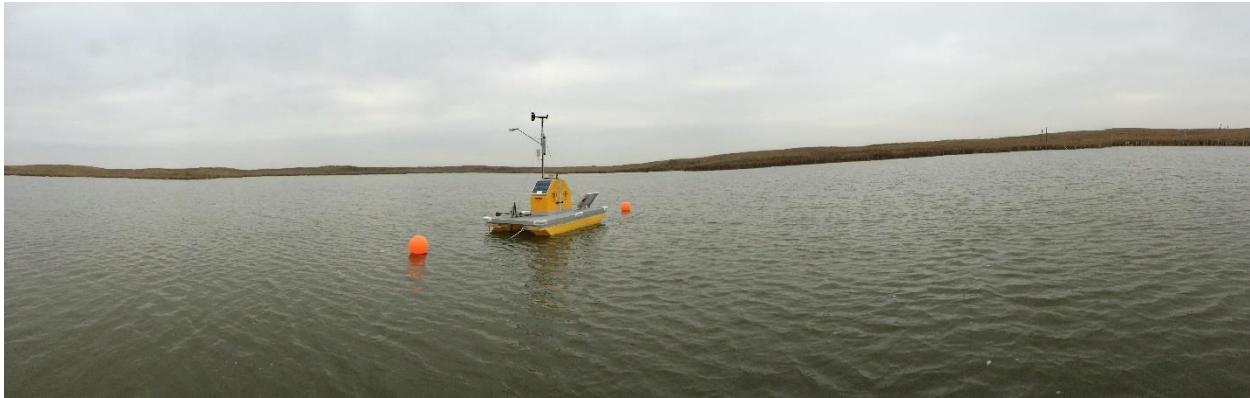
Figure 15. AIS Buoy for Lake and River Sites
