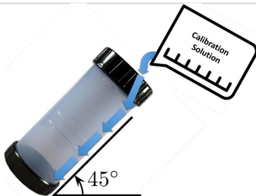
Figure 92. Pour Solution at an Angle to Decrease Aeration
