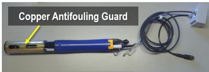
Figure 21. Location of Antifouling Guard
