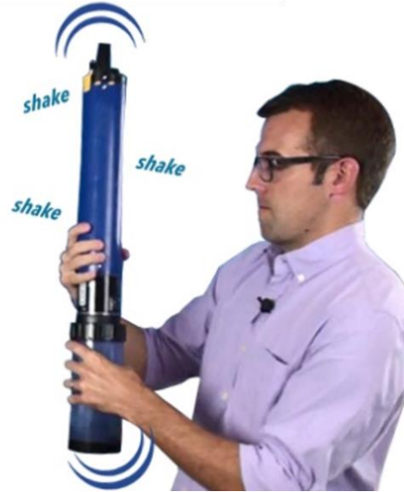
Figure 82. Triple Rinse Sensors & Calibration Cup with DI Water (Source: ER [08] Slide 10)
