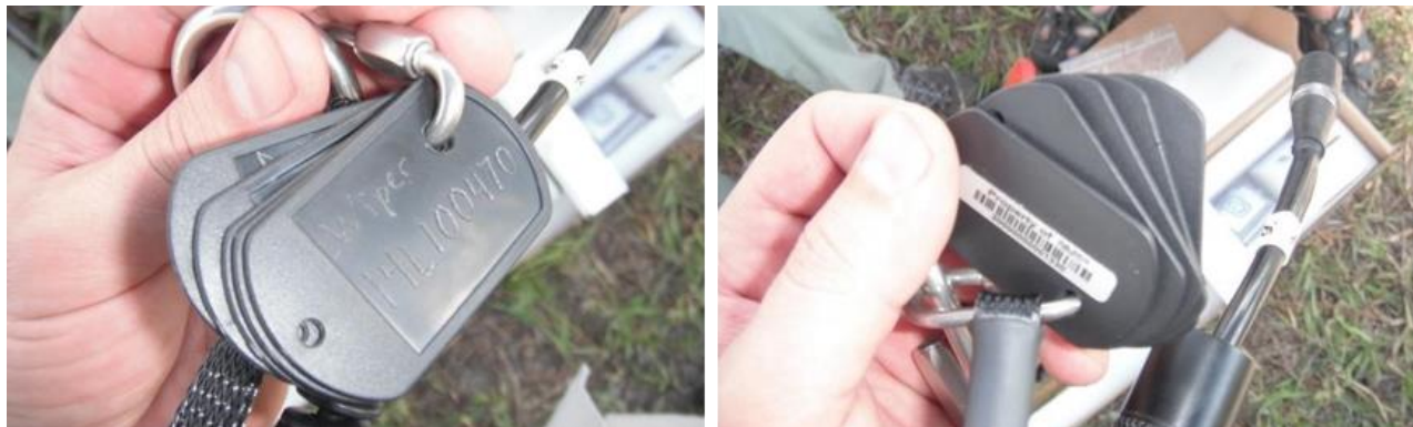
Figure 134. Multisonde Probe Sensor Asset Tags
