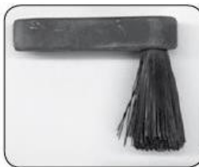
Level 2- Moderate splaying, have spare ready
