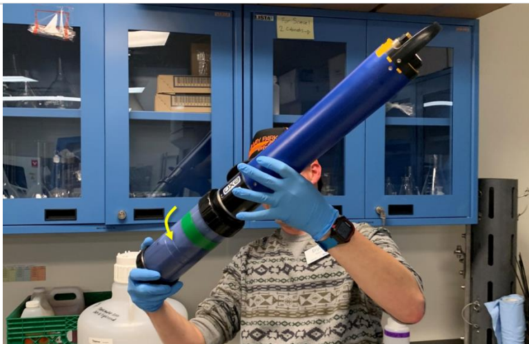
Figure 88. Bryce Nance is Gently Rotating the Multisonde to Remove Bubbles
