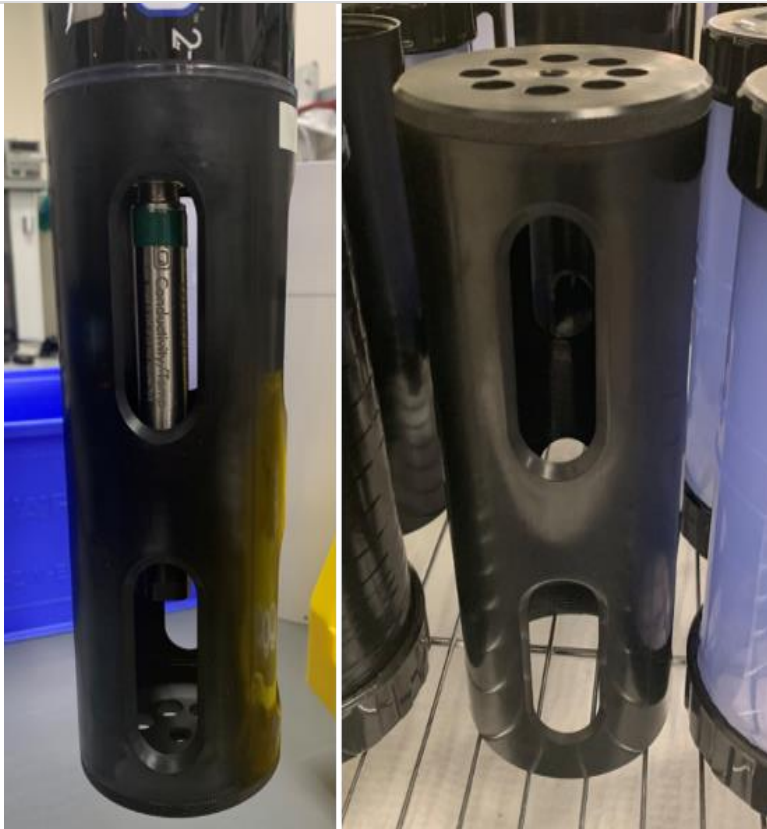
Figure 83. Multisonde Black Plastic Guard for Calibration of Optical Sensors
