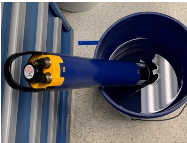
Figure 59. Capture Post-Clean Reading using Same Bucket of Water
