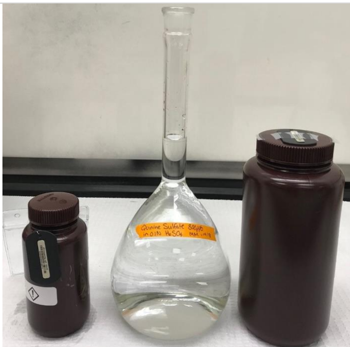
Figure 75. Prepared fDOM Calibration Solution with Amber/HDPE Bottles
