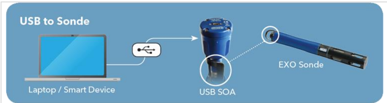
Figure 43. Connect to Multisonde using a USB SOA
