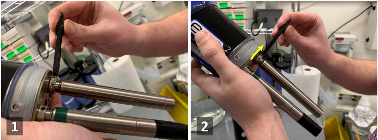
Figure 129. How to Reinstall a Sensor Probe
