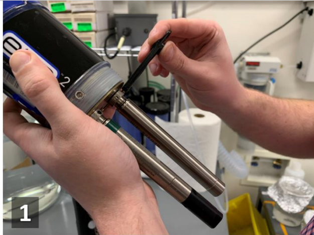
Figure 127. Use the Multisonde Probe Tool to Remove each Sensor Probe from the Multisonde
