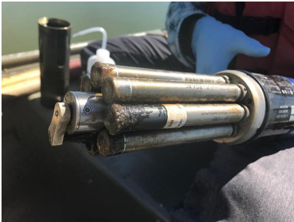
Figure 66. Example of Biofouling on Sensor Probes
