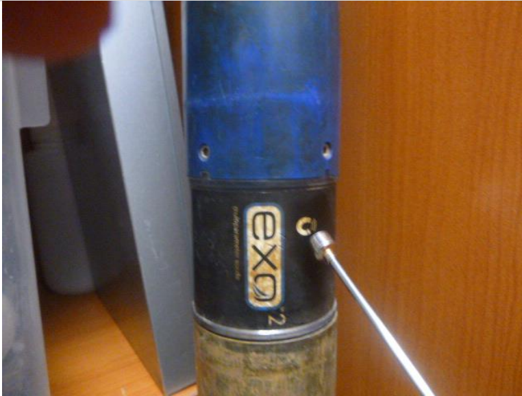
Figure 48. Wake up the Multisonde!
