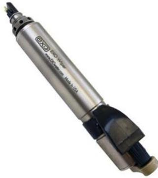
Figure 10. Central wiper (not a sensor)
