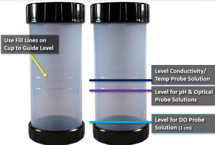
Figure 83. Amount of calibration solution to use for each sensor probe
