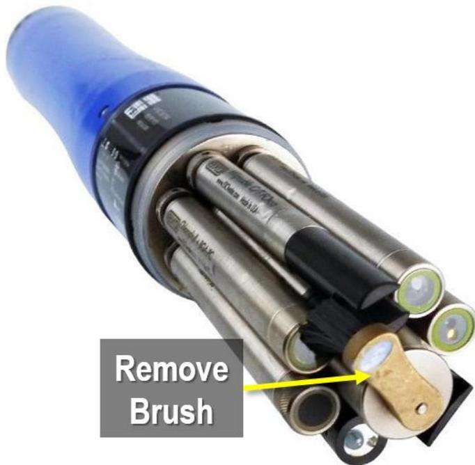
**Figure 80. Remove central wiper brush**
