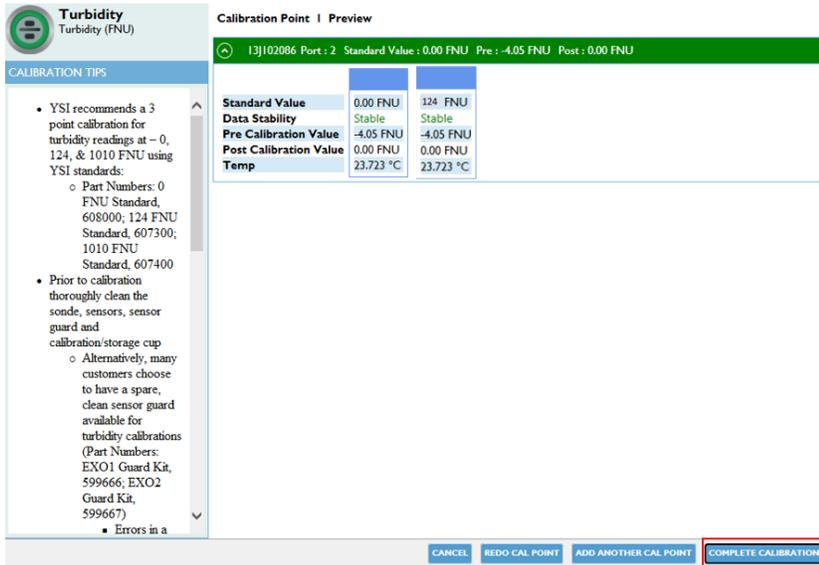
Figure 94. "Complete Calibration" once appropriate number of points complete.
