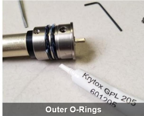
Figure 158. Grease the four o-rings
