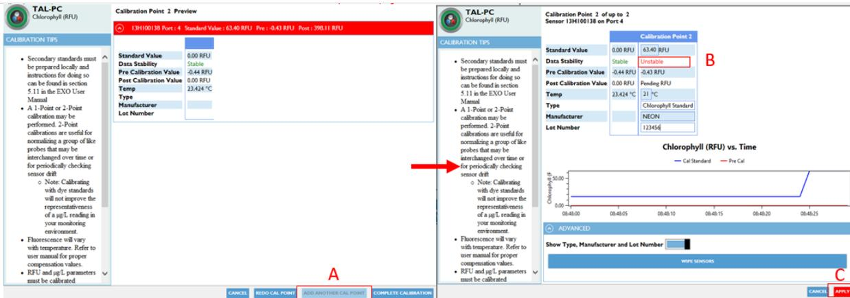
Figure 98. Complete first calibration point and then proceed to second.
