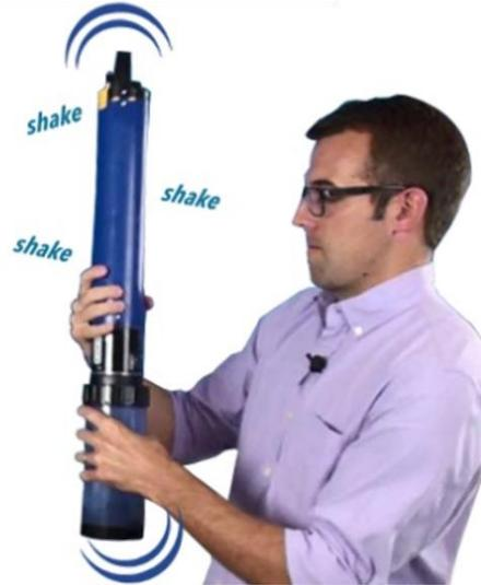
Figure 81. Triple rinse sensors & calibration cup with DI water (Source: [ER \[08\]](#) Slide 10)
