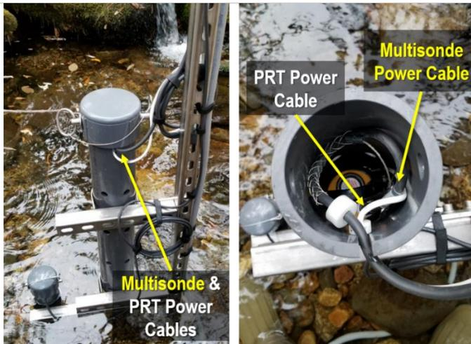
Figure 124. Disconnect sensor power cable
