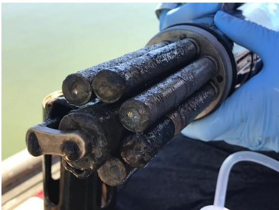
Figure 61. Example of biofouling on sensor probes
