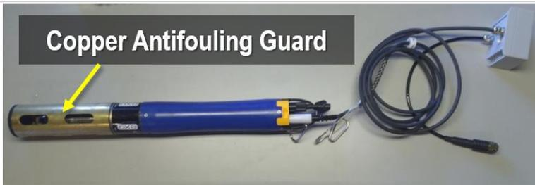
Figure 54. Antifouling guard on Multisonde
