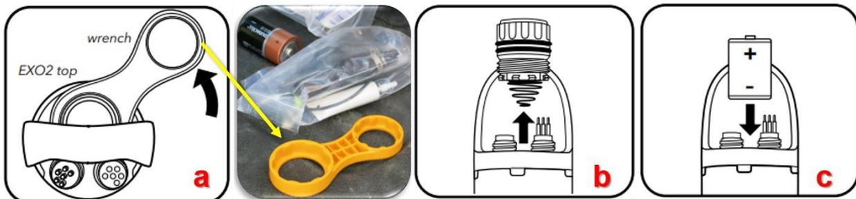
Figure 33. How to replace Multisonde internal D-Cell batteries [Source: ER [02]]
