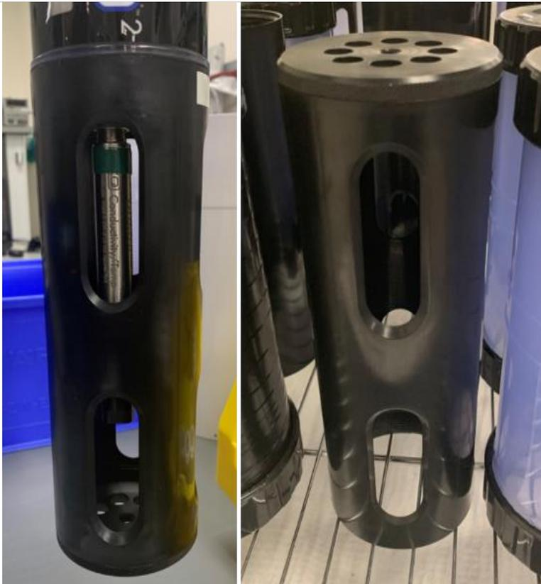
Figure 82. Multisonde black plastic guard for calibration of optical sensors
