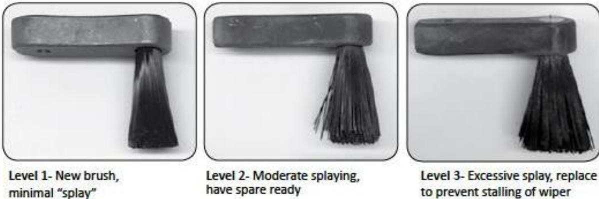
Figure 24. Multisonde anti-fouling wiper: Levels of wear over time [Source: [ER \[02\]](#)]
