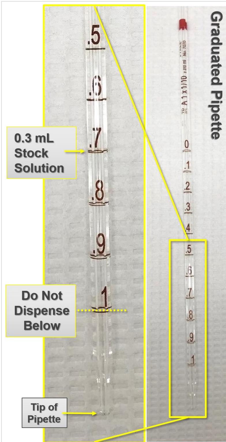
Figure 73. Graduated pipette use for fDOM calibration solution
