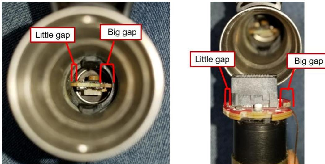
Figure 161. Align gaps on motor and housing
