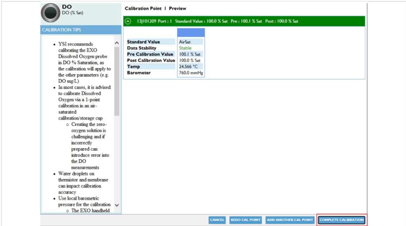
Figure 109. Complete the single point calibration..
