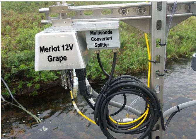
Figure 126. Multisonde Merlot Grape in Grape shield with converter/splitter box
