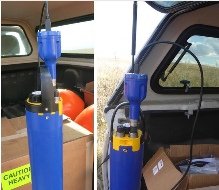
Figure 44. Complete connection to Multisonde using a USB SOA
