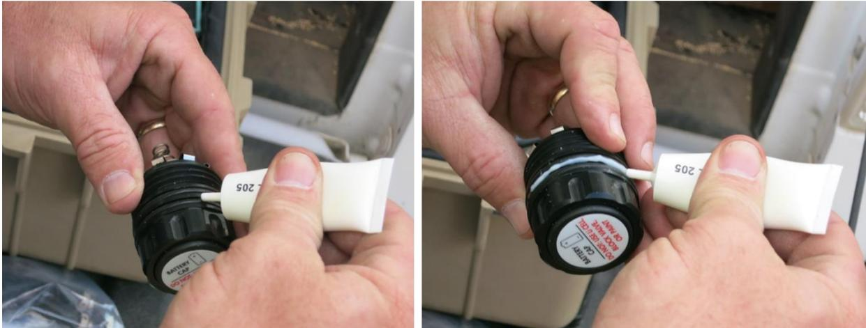
Figure 34. Lubricate battery cap with Krytox grease
