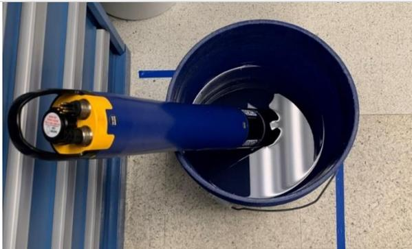
Figure 57. Capture post-clean reading using same bucket of water
