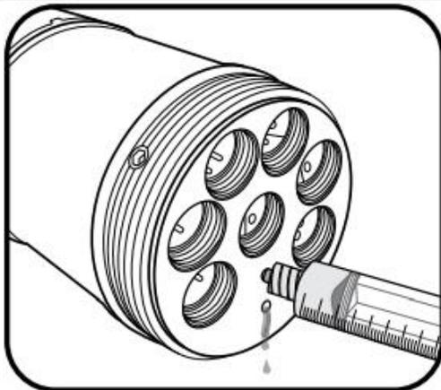
Figure 32. Depth port quarterly maintenance [Source: ER [02]]
