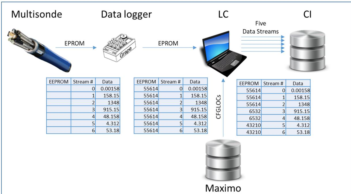
Figure 153. How a Multisonde streams with multiple EPROM IDs
