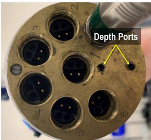
Figure 31. Depth ports on EXO2 Multisonde
