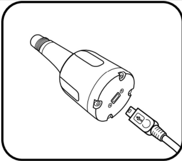
Figure 42. Insert small end of USB cable into SOA connector [Source: [ER \[02\]](#)]
