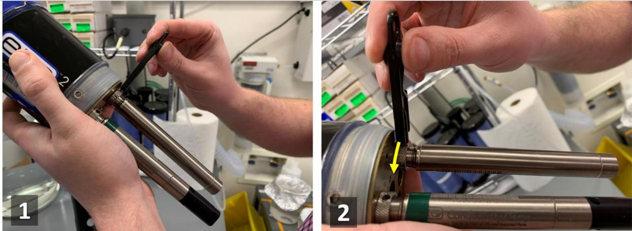
Figure 125. Use the Multisonde probe tool to remove each sensor probe from the Multisonde
