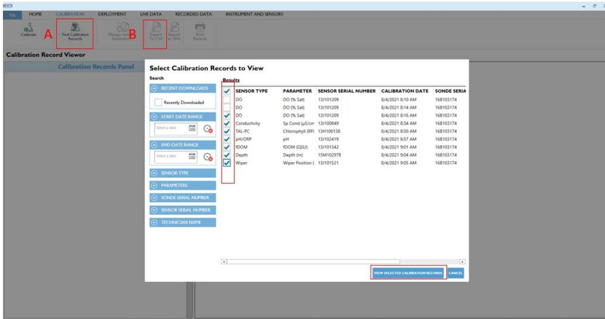
Figure 116. At the end of every PM, collect calibration into one CSV.
