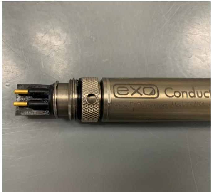
Figure 28. Sensor 4-Pin connectors on Multisonde body (left) and probe sensor (right)
