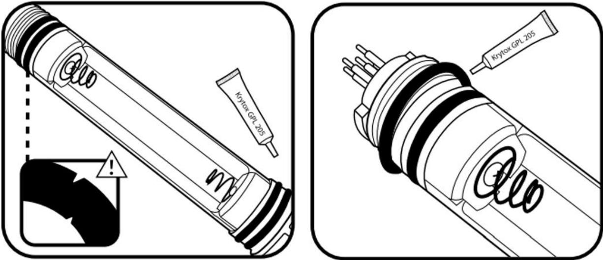
Figure 35. Remove damaged o-rings and replace with lightly greased new o-rings [Source: [ER \[02\]](#)]
