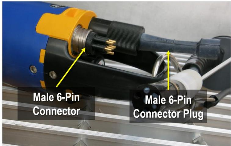
Figure 27. Male 6-Pin connector and dummy plug for 6-Pin connectors [Source: [ER \[02\]](#)]
