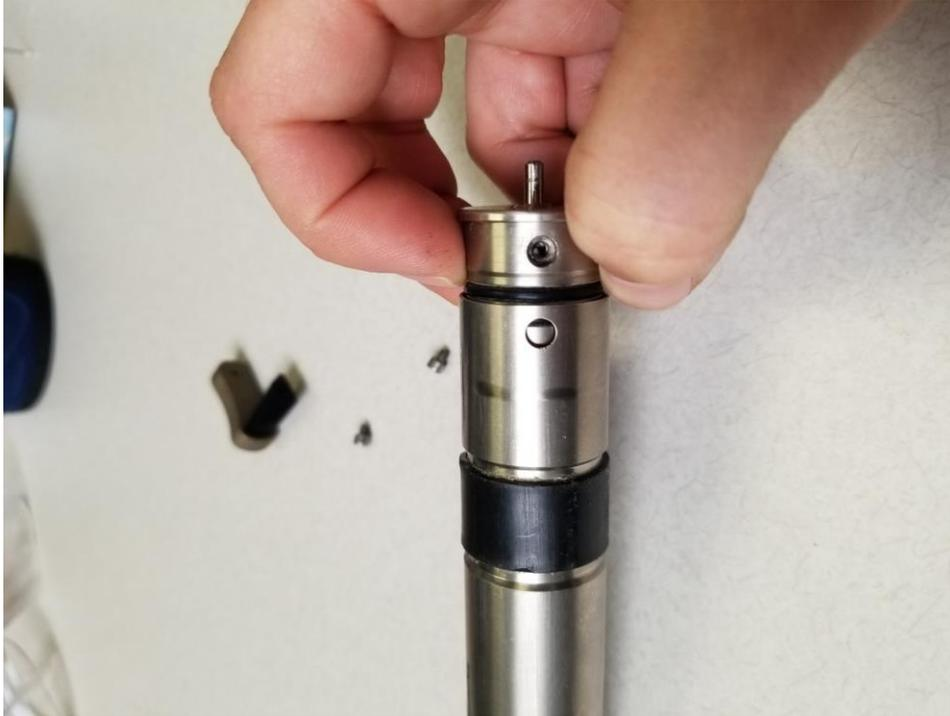
Figure 156. Pull the wiper motor out
