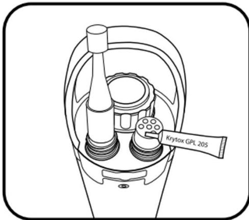
**Figure 26. Greased female 6-Pin connector with Krytox [Source: ER [021)]**
