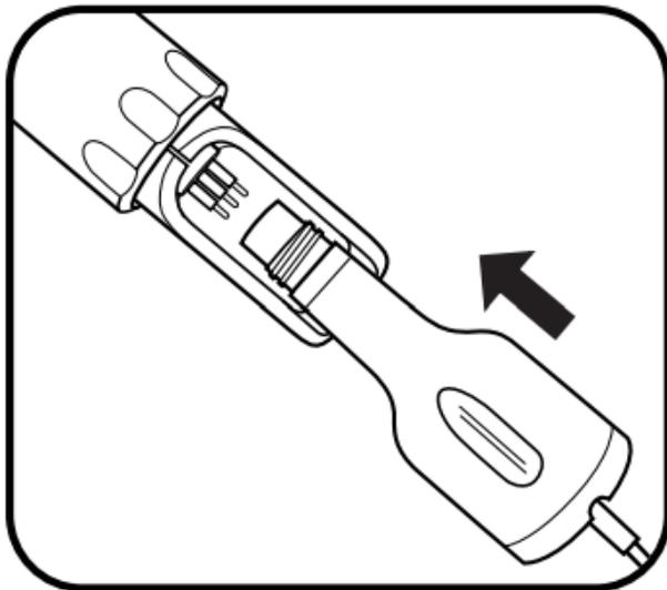
Figure 43. Align the connector's six pins and jackets with sensor [Source: [ER \[02\]](#)]
