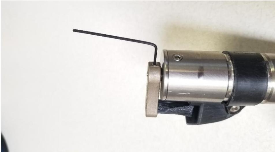
Figure 154. Brush head retention screw
