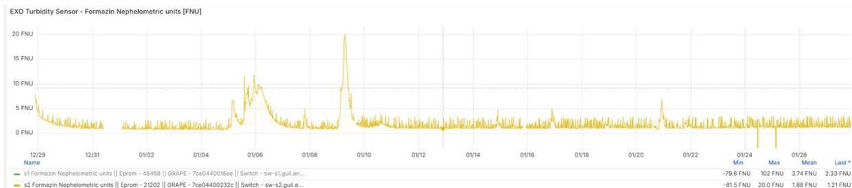
Figure 172. Wiper interference within optical path
