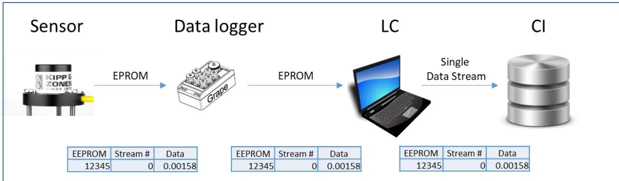
Figure 152. How a sensor streams with a single EPROM ID
