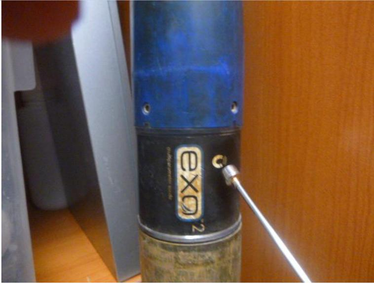
Figure 46. Wake up the Multisonde!
