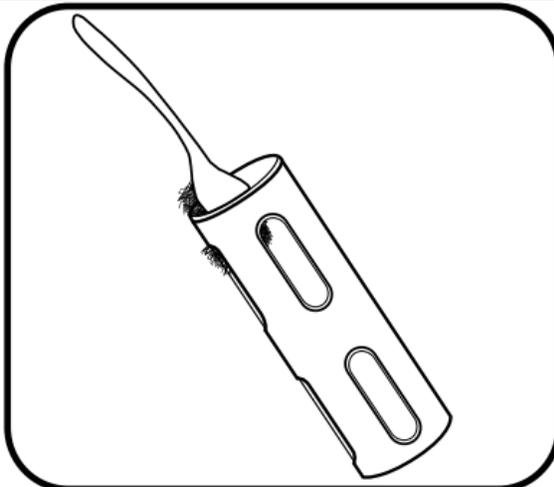
Figure 23. Scrub to remove heavy biofouling [Source: [ER \[02\]](#)]
