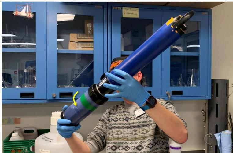
Figure 87. Bryce Nance is gently rotating the Multisonde to remove bubbles
