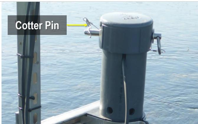
Figure 123. Remove cotter pin to remove PVC slip cap
