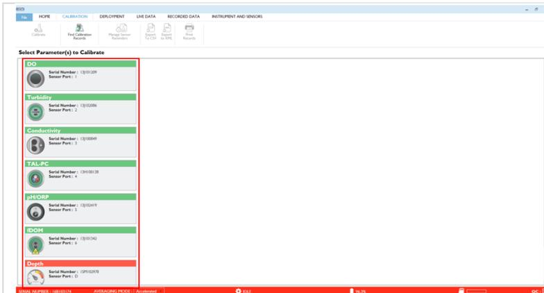
Figure 86. Select parameters for calibration.
