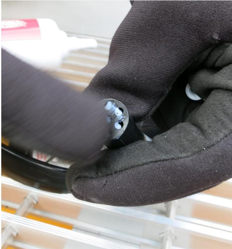
**Figure 25. Apply Krytox to female 6-Pin connectors**
