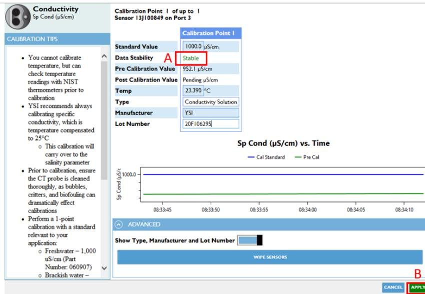
Figure 89. Wait for stable data before applying.
