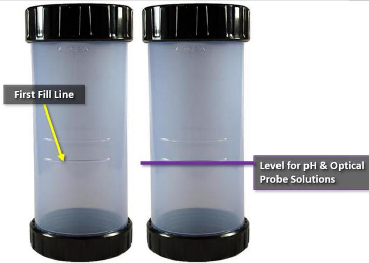
Figure 103. Fill the calibration cup with buffer solution to 1st line
