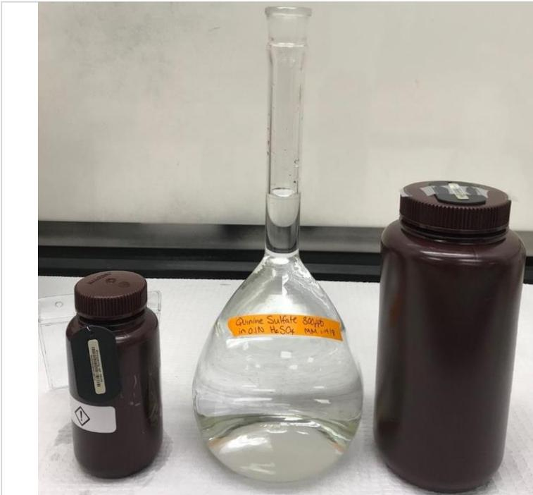
Figure 74. Prepared fDOM calibration solution with Amber/HDPE bottles
