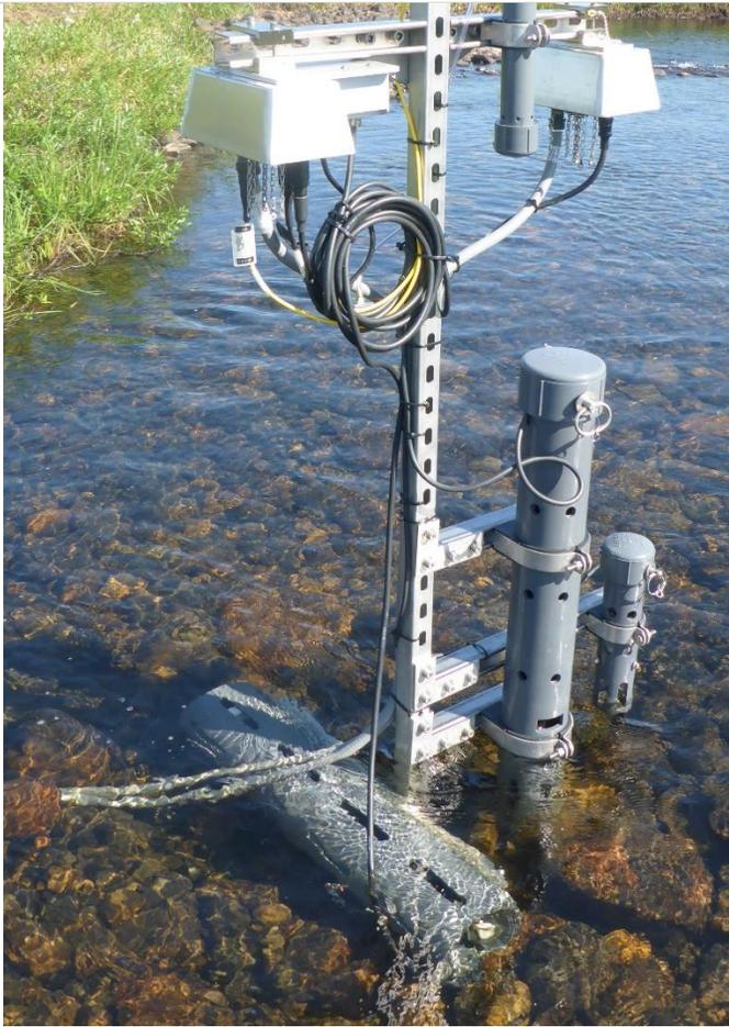
Figure 129. Multisonde cable dressing - complete installation
