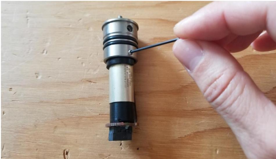
Figure 157. Access the internal o-rings
