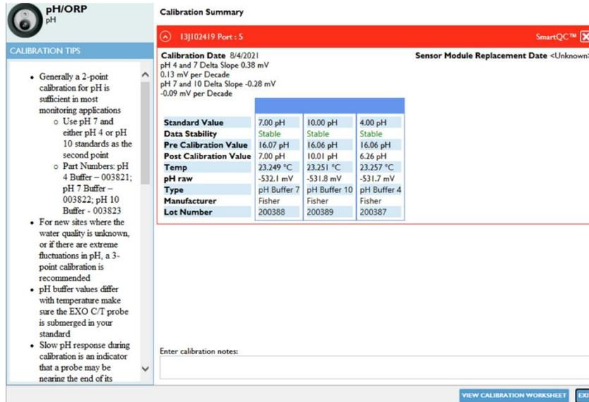
Figure 115. Red bar indicates a failed calibration.
