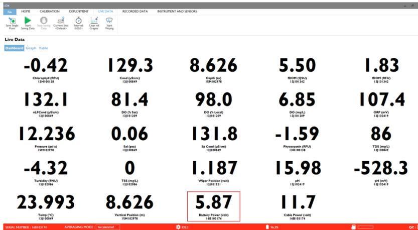
Figure 36. Battery voltage can be found under live data
