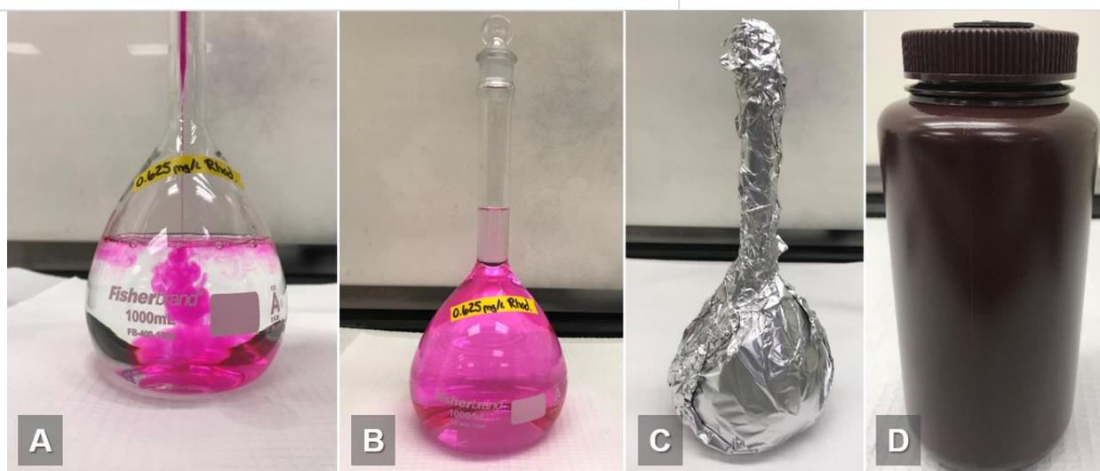
Figure 77. Prepare Total Algae/Chlorophyll calibration solution with Rhodamine WT and DI water
