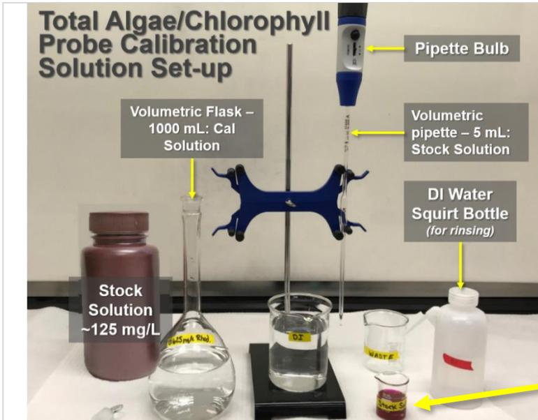
Figure 75. Total Algae/Chlorophyll calibration solution preparation
