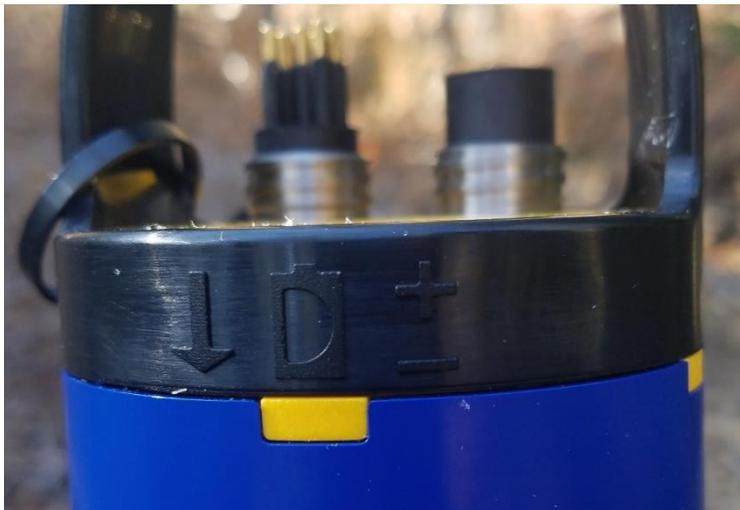
Figure 37. Battery orientation on battery cap
