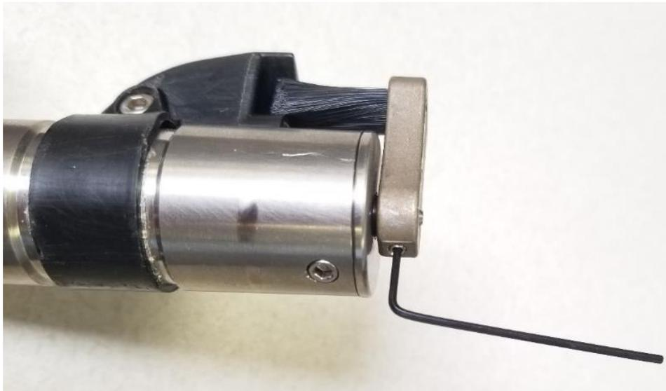
Figure 162. Tighten brush set screw
