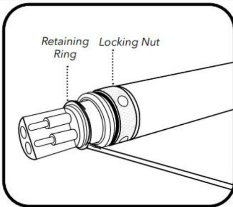
Figure 30. Sensor locking nuts & retaining ring [Source: ER [02]]
