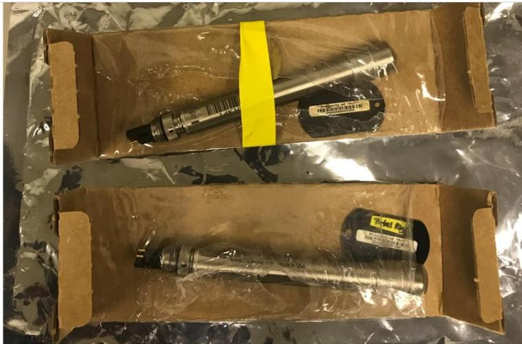
**Figure 132. General probe sensor packaging for shipping/handling**
