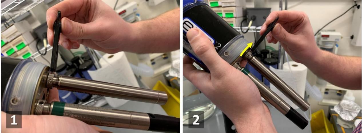
Figure 127. How to reinstall a sensor probe
