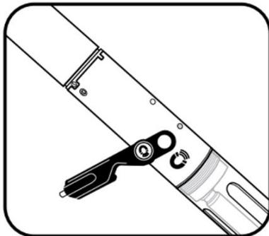
Figure 47. Activate the Multisonde's Bluetooth capability [Source: [ER \[02\]](#)]
