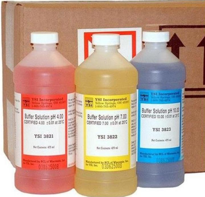
Figure 101. pH probe calibration buffer solutions
