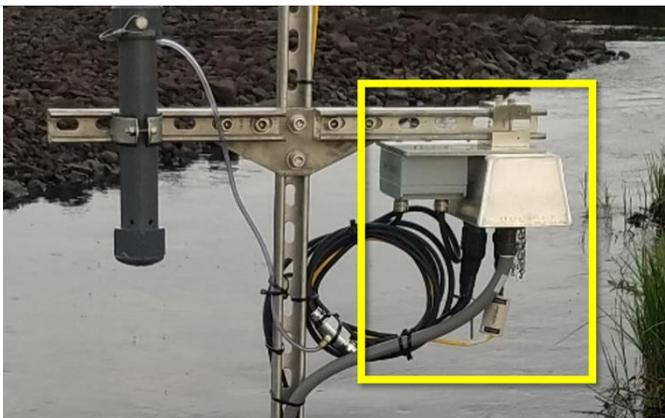
Figure 128. Connect sensor cables to Grape
