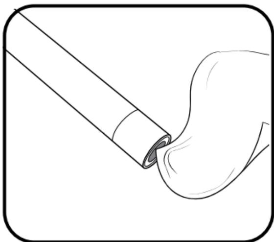
Figure 60. Clean optical sensor windows [Source: ER [02]]
