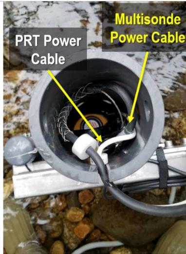
Figure 39. Disconnect the black power cable
