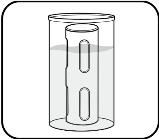
Figure 22. Soak to remove heavier biofouling [Source: [ER \[02\]](#)]
