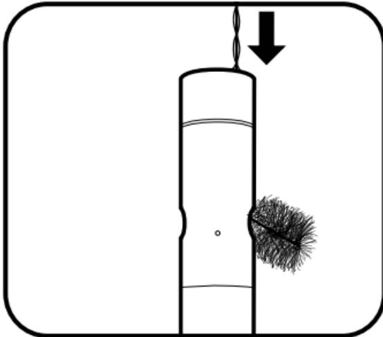
Figure 66. Clean conductivity & temperature sensor probe
