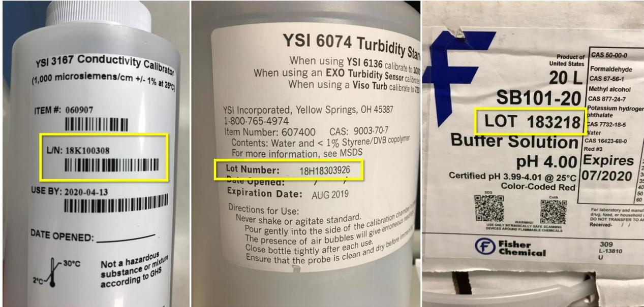
**Figure 68. Lot numbers on Multisonde calibration solutions**
