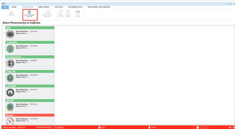
Figure 85. Navigate to calibration menu.
