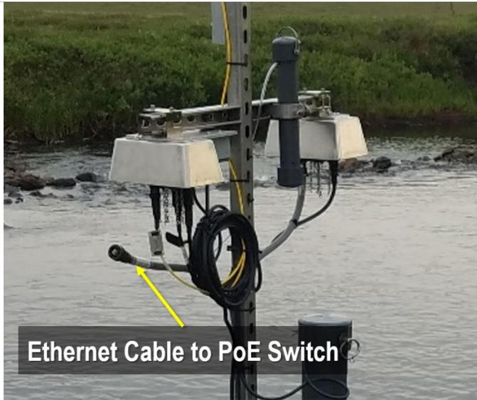
Figure 122. Disconnect ethernet cable (RJF) from Merlot Grape
