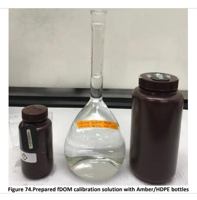
**STEP 3** | For storage and when traveling to site, protect this solution from light by using an amber or HDPE bottle (**Figure 74**).
