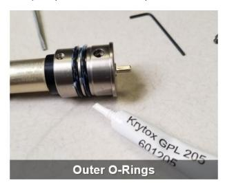
Figure 158. Grease the four o-rings
