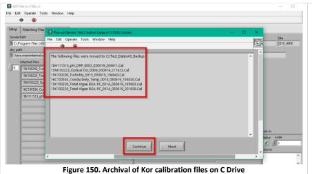
STEP 7 | This screen displays the files that the application moves from the Kor folder to an Archive folder on the C Drive. Notice in Figure 150, there are two files for Chlorophyll. That is because the probe sensor failed its initial calibration.
