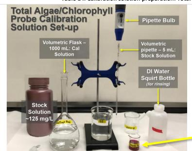
Figure 75. Total Algae/Chlorophyll calibration solution preparation
