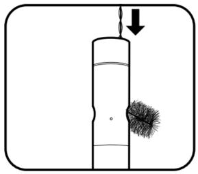
Figure 66. Clean conductivity & temperature sensor probe [Source: ER [02])
