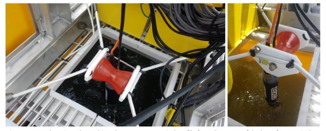
Figure 16. At select sites, the Multisonde measures a vertical profile from the center of the buoy from a winch
