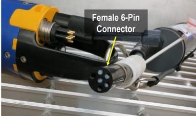
Figure 26. Greased female 6-Pin connector with Krytox [Source: ER [02])
