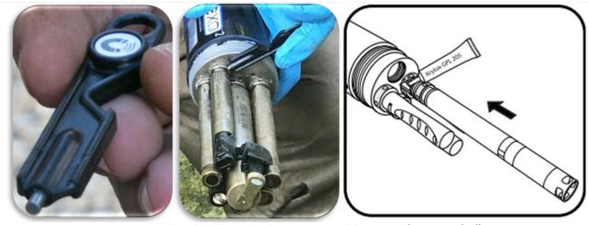
Figure 29.Multisonde probe tool and Krytox GPL 205 lubricant use [Source: ER [02])
