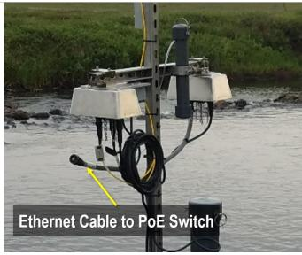
Figure 122. Disconnect ethernet cable (RJF) from Merlot Grape
