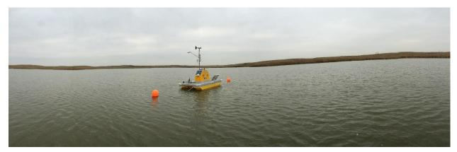
Figure 15. AIS buoy for lake and river sites
