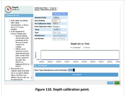
**STEP 2** | In the Kor software, under the Calibration Menu, select Depth. Input the following information (**Figure 110**):
