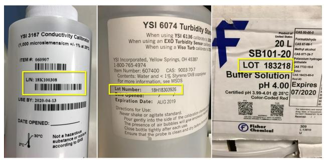
Figure 68. Lot numbers on Multisonde calibration solutions
