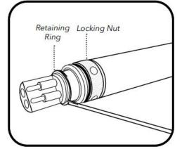
Figure 30. Sensor locking nuts & retaining ring [Source: ER [02])
