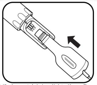
Figure 43. Align the connector's six pins and jackets with sensor [Source: ER [02])
