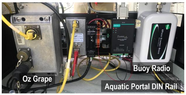
Figure 17. Aquatic portal precip DIN rail: AIS buoy portal radio/Oz grape subsystem
