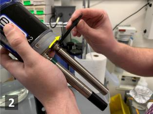
Figure 127. How to reinstall a sensor probe
