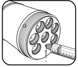
Figure 32. Depth port quarterly maintenance [Source: ER [02])
