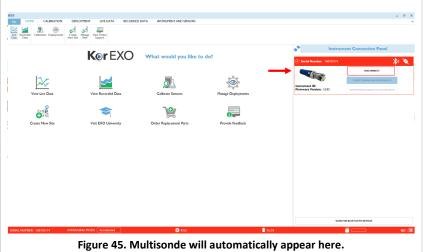
**STEP 5.2** | Launch the Kor software on a laptop. The EXO Multisonde should appear in the **Instrument Connection Panel**.
