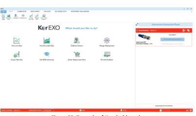
STEP 5 | With the anti-fouling guard still on, collect a stabilized pre-clean reading in Fulcrum by navigating to the Dashboard in the Kor Software and selecting the "Live Data" icon in the top left banner on the screen in Figure 55.
