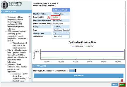
Figure 89. Wait for stable data before applying.
