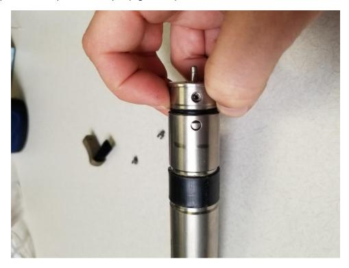
Figure 156. Pull the wiper motor out
