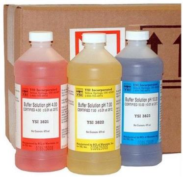
**STEP 1** | This sensor requires three buffer solutions for a three-point calibration: pH 7.00, pH 10.00, and pH 4.00
