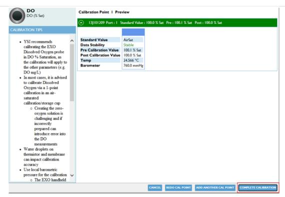
Figure 109. Complete the single point calibration..
