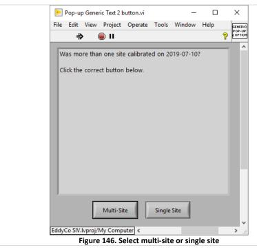
STEP 7 | If this is for two sites on the same day, select the "Multi-Site" button to select the sensor files for the site you selected in Step 5. You will need to do the same process again for the second site after you complete the first site's file transfer process.
