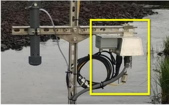
Figure 128. Connect sensor cables to Grape
