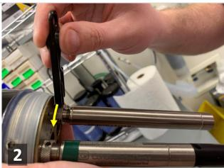
Figure 125. Use the Multisonde probe tool to remove each sensor probe from the Multisonde
