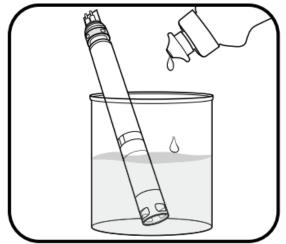
Figure 64. Clean pH/ORP sensor probe [Source: ER [02])
