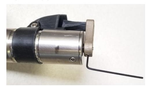
Figure 162. Tighten brush set screw
