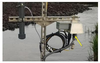
Figure 38. Merlot grape with signal output adapter (splitter/converter box)
