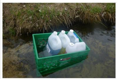
Figure 102. pH buffer solutions in stream
