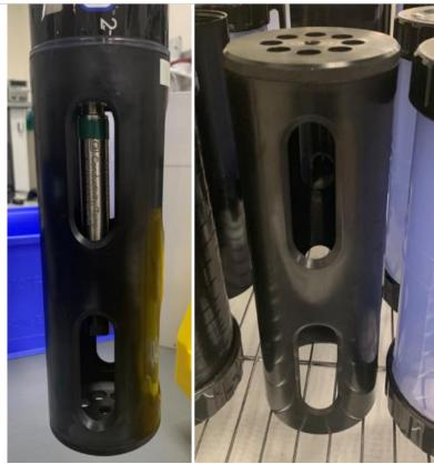
Figure 82. Multisonde black plastic guard for calibration of optical sensors
