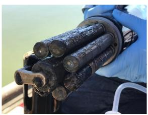
Figure 61. Example of biofouling on sensor probes
