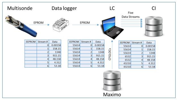
Figure 153. How a Multisonde streams with multiple EPROM IDs
