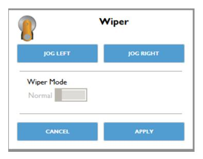
Figure 163. When calibrating wiper, click left/right to adjust position
