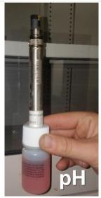
Figure 134. pH probe shipping requirements
