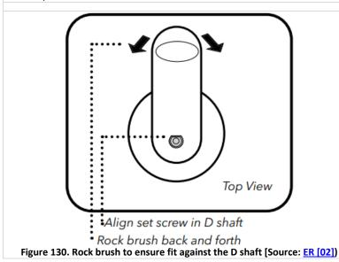
**STEP 5** | Tighten setscrew to a torque of 4 inch-pounds.
