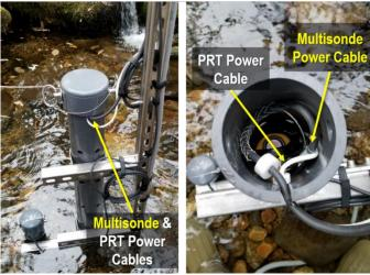
Figure 124. Disconnect sensor power cable
