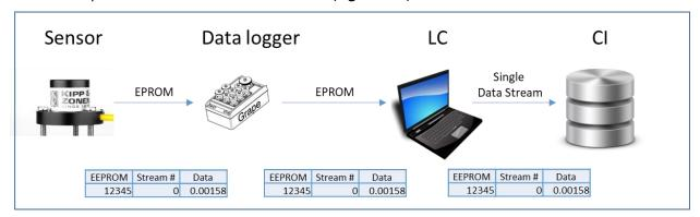
Figure 152. How a sensor streams with a single EPROM ID
