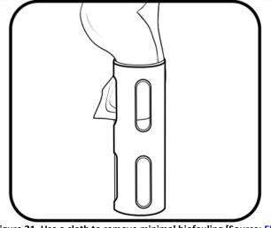
Figure 21. Use a cloth to remove minimal biofouling [Source: <u>ER</u> [02])
