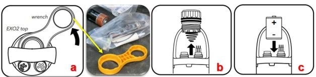
Figure 33. How to replace Multisonde internal D-Cell batteries [Source: ER [02])
