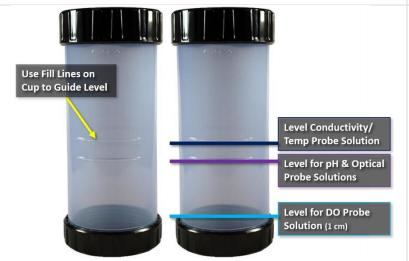
Figure 83. Amount of calibration solution to use for each sensor probe
