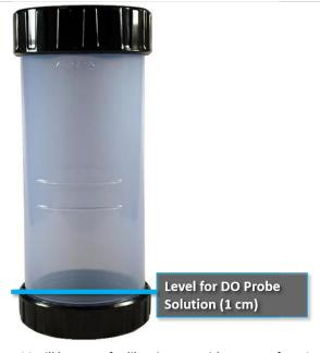
Figure 106. Fill bottom of calibration cup with DI water for DO probe
