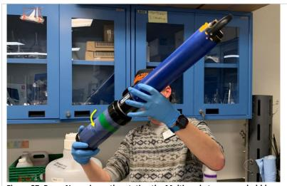
Figure 87. Bryce Nance is gently rotating the Multisonde to remove bubbles
