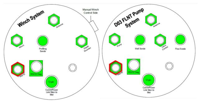
Figure 19. Disable the buoy from its power source: disconnect the "Pwr In" cable on the profile canister (Source: AD [10])
