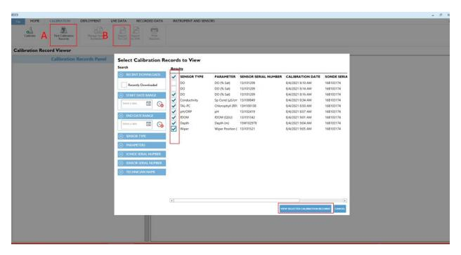
Figure 116. At the end of every PM, collect calibration into one CSV.
