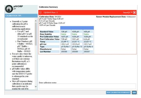
Figure 115. Red bar indicates a failed calibration.
