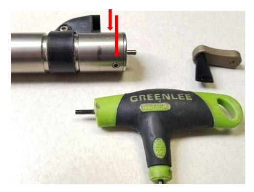
Figure 155. Two screws located at top of wiper
