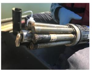
Figure 65. Example of biofouling on sensor probes
