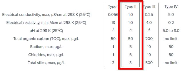
Figure 78. DI water minimum requirements: ATSM Type II<sup>2</sup>
