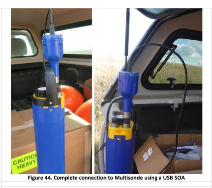
**Figure 44** displays the complete connection: USB to USB-SOA to EXO Multisonde.
