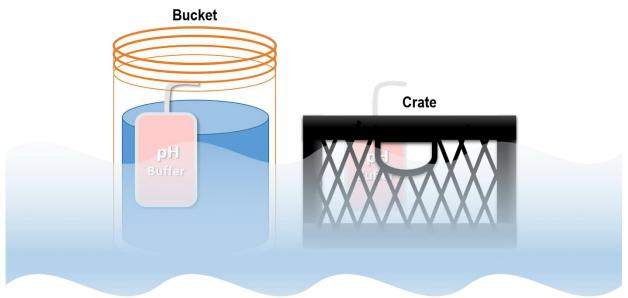
Figure 79. Alternate setups for pH and DI water temperature equilibration
