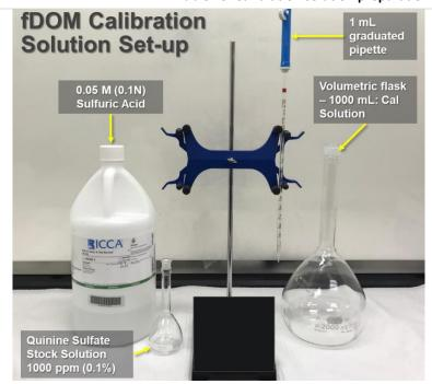
Figure 72. fDOM calibration solution set-up
