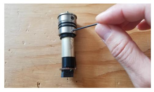
Figure 157. Access the internal o-rings
