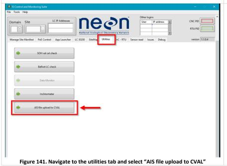
STEP 2 | Navigate to the Utilities tab and select "AIS file upload to CVAL" (Figure 141).
