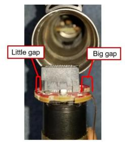
Figure 161. Align gaps on motor and housing
