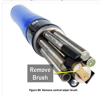
STEP 3 | It is assumed that the brush was removed during the cleaning process. If not, remove the central wiper brush and clean the area around and under where the brush was installed. (Biofouling may accumulate under the brush over time.) Additionally, the copper in the assembly degrades the fDOM calibration solution (quinine sulfate solution) within minutes.
