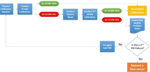
Figure 113. Calibration Pass/Fail criteria for sites with one (1) Multisonde.
