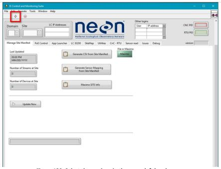
STEP 1 | Launch the IS Control and Monitoring Suite and select the Run icon in the upper left hand corner of the window (white arrow in Figure 139 and Figure 140).
