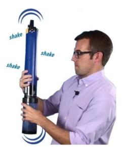
Figure 81. Tripe rinse sensors & calibration cup with DI water (Source: ER [08] Slide 10)
