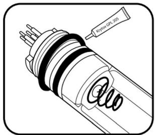
Figure 35. Remove damaged o-rings and replace with lightly greased new o-rings [Source: ER [02])
