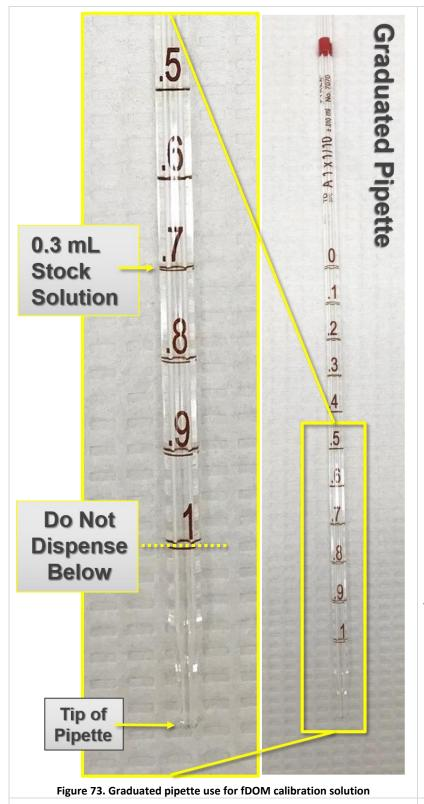
STEP 2 | Prepare the 300 ug/L fDOM calibration solution. Fill the flask approximately half way with 0.1 N H2SO4. Dilute 0.3 mL of stock solution into the 1000 mL volumetric flask (Figure 73).
