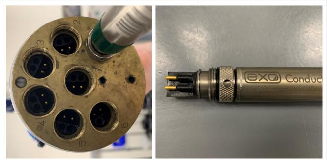
Figure 28. Sensor 4-Pin connectors on Multisonde body (left) and probe sensor (right)
