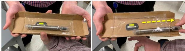
Figure 137. Move the sides of the Insert up to create slack in plastic packaging to remove sensor and asset tag
