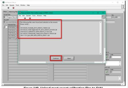
Figure 149. Upload most recent calibration files to CVAL
