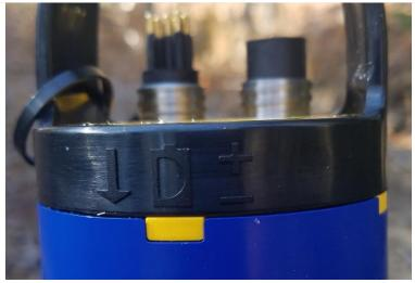
Figure 37. Battery orientation on battery cap
