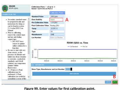
**STEP 2** | In the Kor software, select the port with the fDOM sensor probe in the Calibration Menu. Input the following information for the first point of a twopoint calibration:
