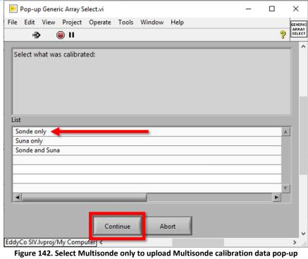
STEP 3 | Select the Multisonde only to upload the calibration data for the Multisonde (Figure 142). Click "Continue" to move to the next step.
