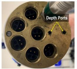
Figure 31. Depth ports on EXO2 Multisonde
