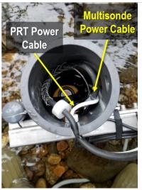
Figure 39. Disconnect the black power cable
