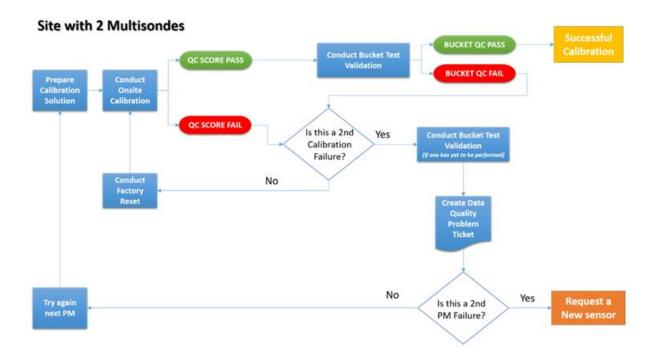
Figure 112. Calibration Pass/Fail criteria for sites with two (2) multisondes.
