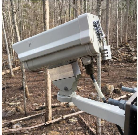
**Figure 4. TIS Tower Snow Depth Camera (Domain 07, GRSM)**
