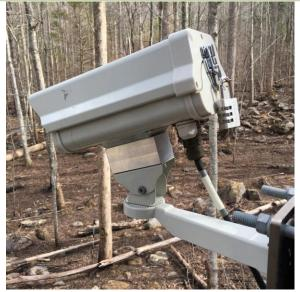
Figure 4. TIS Tower Snow Depth Camera (Domain 07, GRSM)
