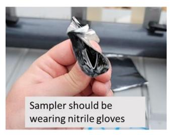
Figure 12. Correctly folded foil pack ready to be placed in the drying oven.
