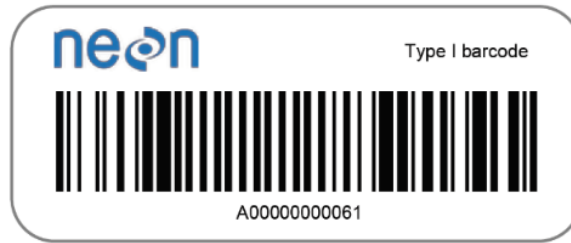
Figure 3. An example of a Type I barcode. These large-size, field-tolerant barcodes have a prefix of 'A' followed by 11 numbers.
