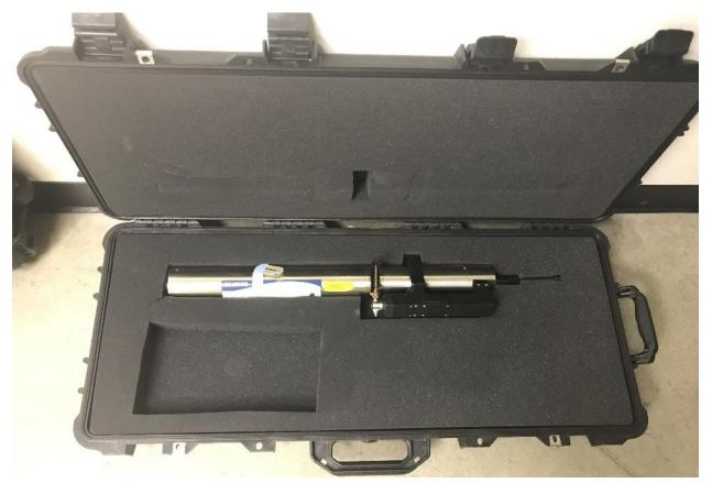
Figure 79. Example of SUNA for Shipping/Storage
