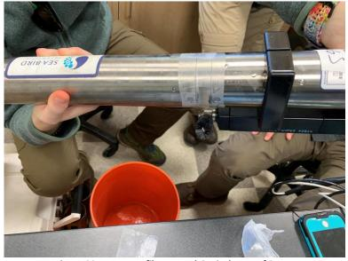
**STEP 9.2** | Wrap the Parafilm around the optical area of the sensor (Figure 33).
