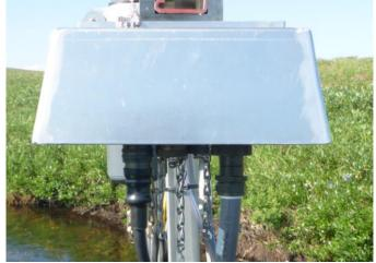
**STEP 12** | Remove dust caps on sensor connectors and Eth-To-Comm connector. Reconnect sensor and armored Ethernet cable in accordance with AD [06].
