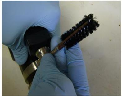
Figure 31. Physically Move Wiper on SUNA
