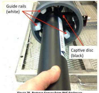
**STEP 8** | Slide the sensor assembly out of the enclosure by grabbing onto the wiper housing at the top of the sensor (Figure 75). The color of the captive discs may vary, but the design and material are the same across stream sites.
