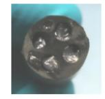
Lubricant on socket end of the connector Lubricant pushed into the sockets of the connector
