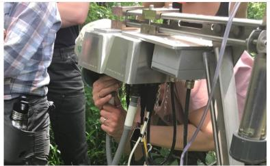
Figure 14. Disconnect the SUNA 12V Merlot Grape
