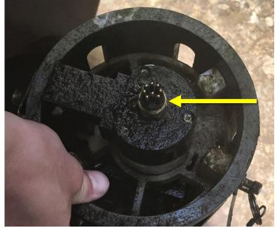
**STEP 3** | Disconnect the power cable from the SUNA bulkhead connector (Figure 16).
