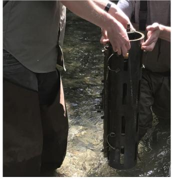
Figure 72. Remove SUNA PVC Enclosure
