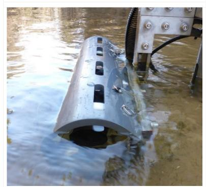
Figure 65. SUNA Partially Submerged in Stream
