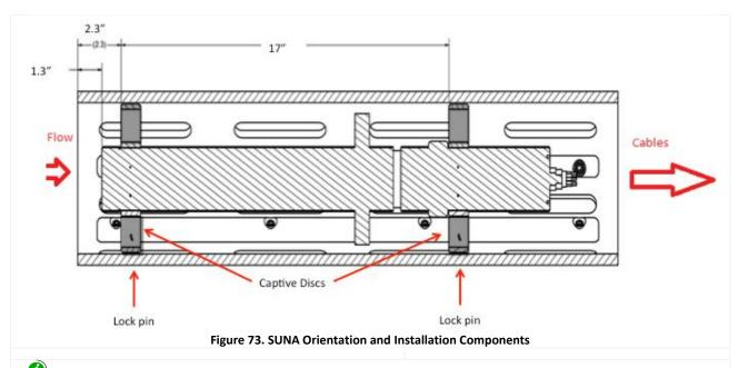
Note: Bio-fouling may accumulate in the tracks, which may cause difficulty removing and reinstalling the SUNA into the PVC enclosure. Try to flush the PVC enclosure with water to dislodge any debris, if possible.
