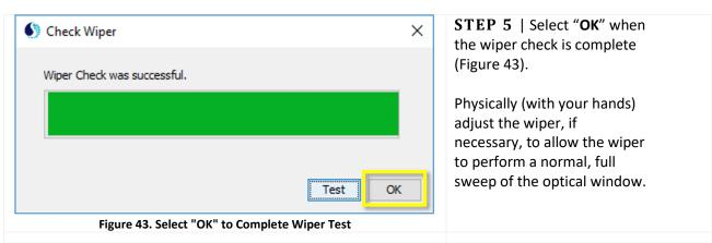
**STEP 6** | Repeat the wiper check until the wiper successfully passes 3 to 4 tests in a row. If the wiper fails this check, it is likely the coupler, submit an incident ticket in the NEON Project's Issue Reporting and Management System.
