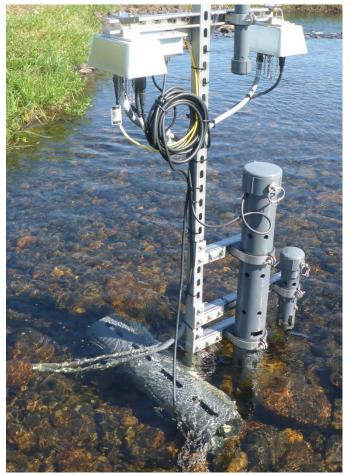
Figure 78. SUNA Cable Dressing - Complete Installation
