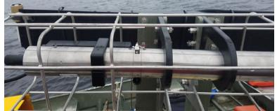
Figure 18. SUNA in Cage on Dual PAR SUNA Mount on the Buoy
