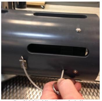
**STEP 7** | Pull the four lock pins from the enclosure to free the two captive discs (Figure 74).
