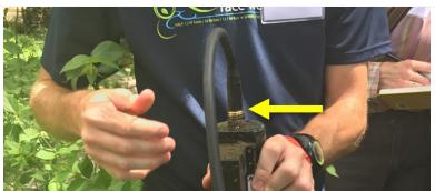
Figure 19. Connect the SUNA to the Y Cable
