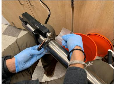
Figure 32. Cut Parafilm to Size
