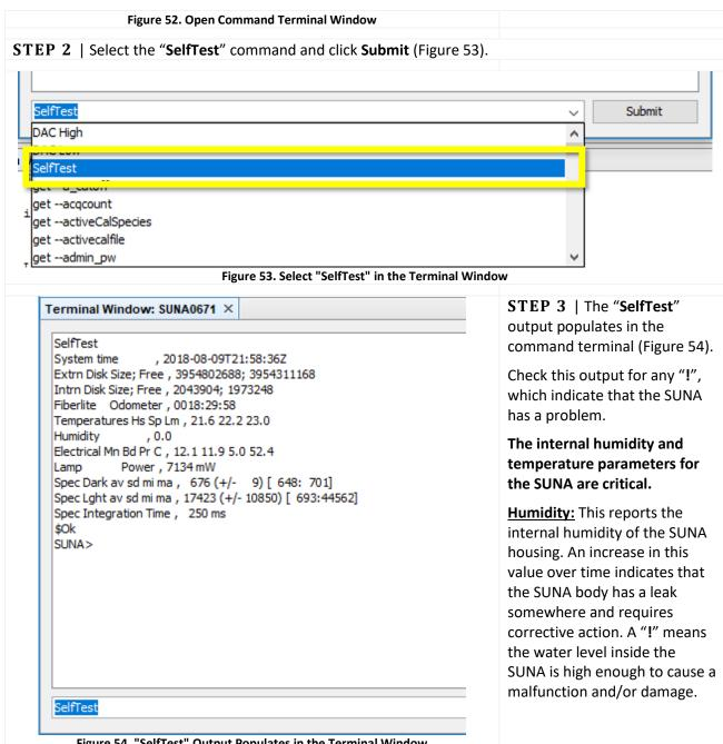
Figure 54. "SelfTest" Output Populates in the Terminal Window
