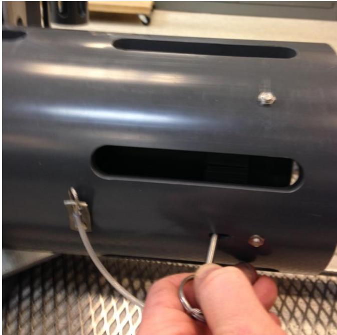
**Figure 74. Pull 4 Lock Pins to Remove Captive Discs**
