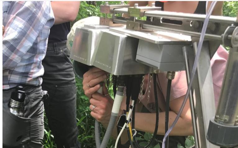
**Figure 14. Disconnect the SUNA 12V Merlot Grape**
