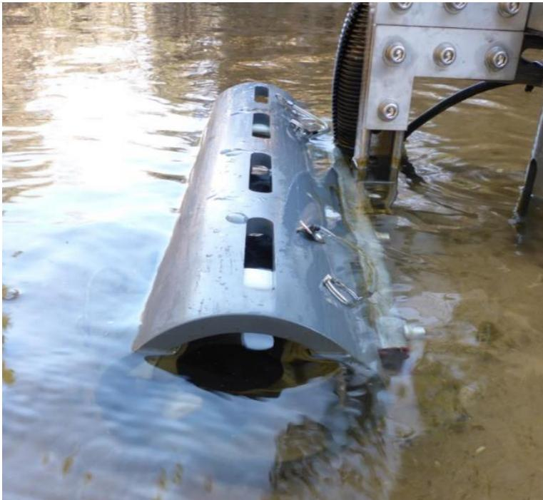
**Figure 65. SUNA Partially Submerged in Stream**
