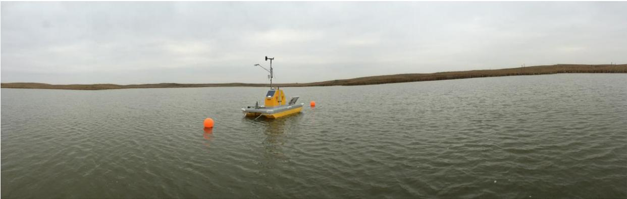
Figure 5. AIS Buoy for Lake and River Sites
