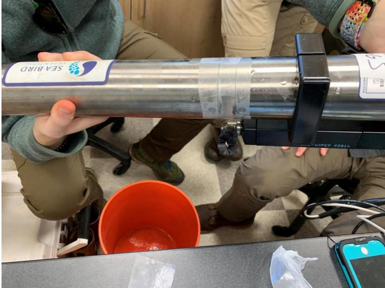
Figure 33. Wrap Parafilm around Optical Area of SUNA
