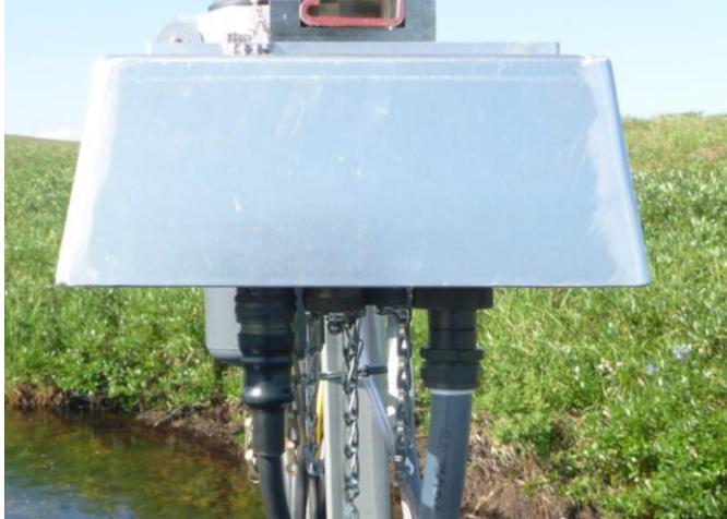
Figure 77. Reconnect Sensor Cable and Ethernet Cable to Grape
