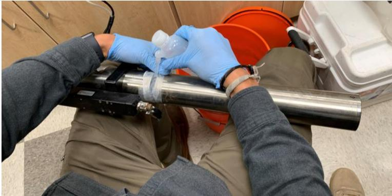
Figure 34. Fill Optical Area with Equilibrated DI Water
