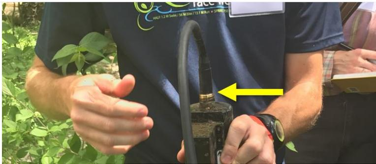
Figure 19. Connect the SUNA to the Y Cable
