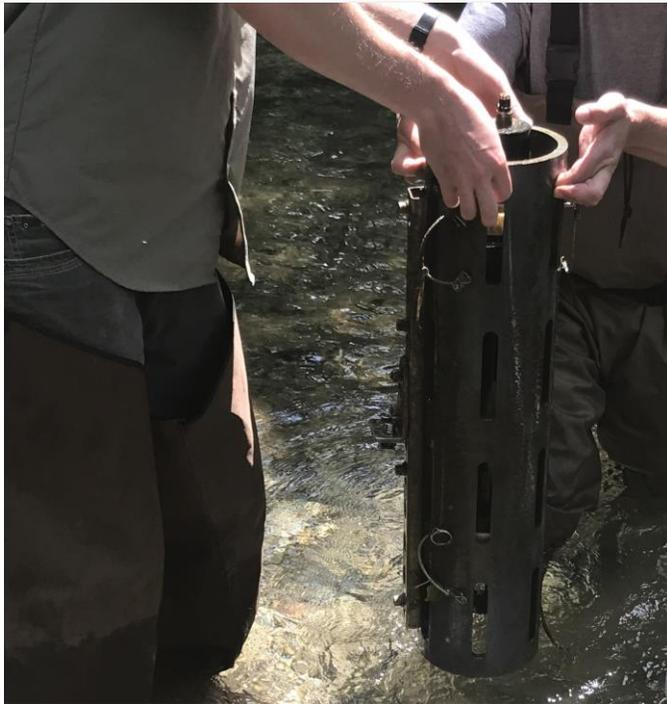
Figure 72. Remove SUNA PVC Enclosure
