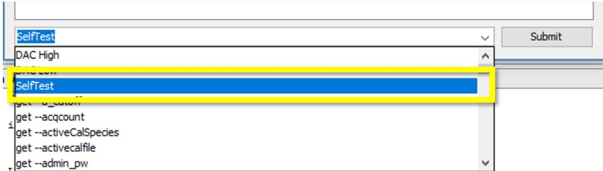
Figure 53. Select "SelfTest" in the Terminal Window
