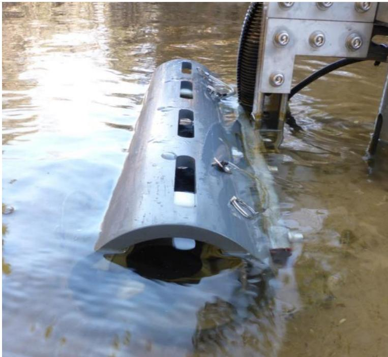
Figure 17. SUNA Mount and Enclosure in Stream Locations
