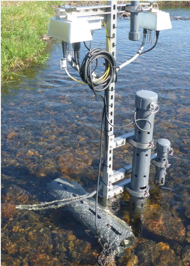
Figure 78. SUNA Cable Dressing - Complete Installation
