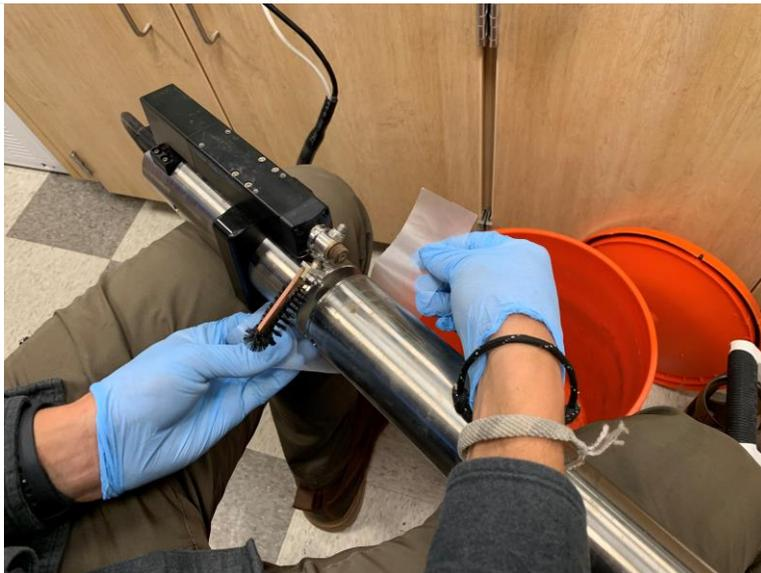
Figure 32. Cut Parafilm to Size
