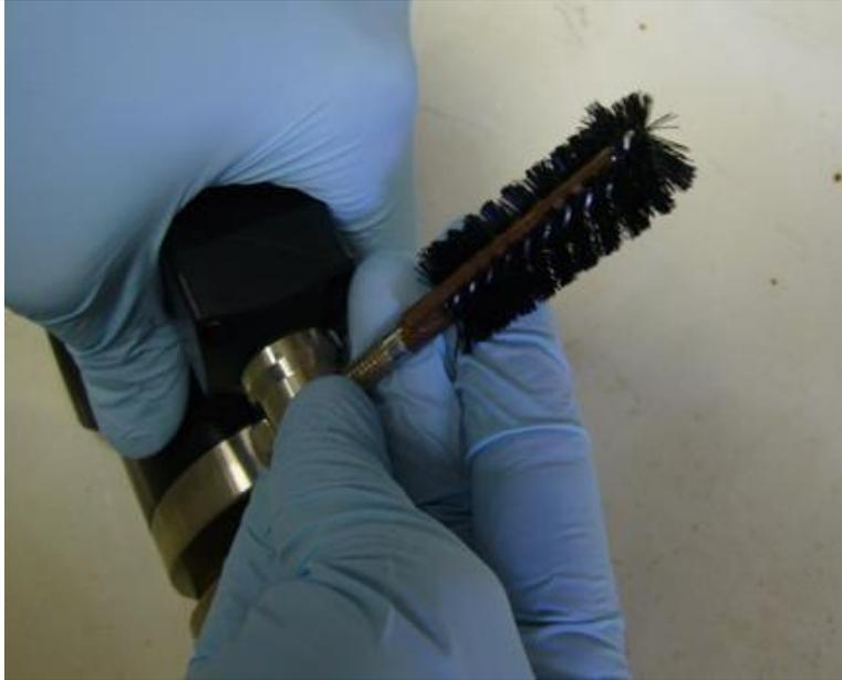
Figure 31. Physically Move Wiper on SUNA
