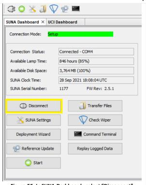
**STEP 1** | In the **SUNA Dashboard**, select the "**Disconnect**" button <u>BEFORE</u> disconnecting the USB connection from the laptop and cable from the SUNA (**Figure 55**).
