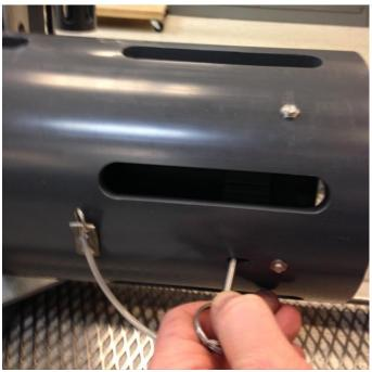
Figure 77. Pull 4 Lock Pins to Remove Captive Discs
