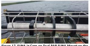
Figure 17. SUNA in Cage on Dual PAR SUNA Mount on the Buoy
