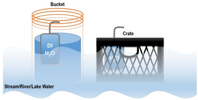
Figure 12. Alternate Setups for DI Water Temperature Equilibration.
