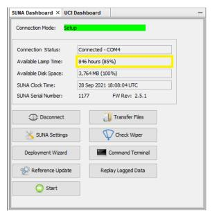
Figure 46. SUNA Dashboard: Available Lamp Time | Verify Lamp Time is > 50 Hours.
