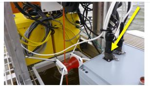
Figure 22. Attach Y-Cable to SUNA Radio Box at Buoy Sites
