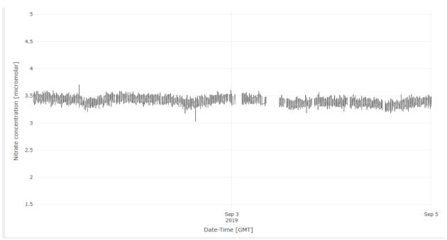
**Figure 95**. This example shows otherwise good data with gaps in it. This is usually a communication issue, not a sensor issue. Check the connection between the SUNA and the Grape data logger. For buoy sites, check the radio link. This particular example occurred for a buoy whose moorings were lose allowing wind to rotate the SUNA antenna out of line of sight with the shore receiver.
