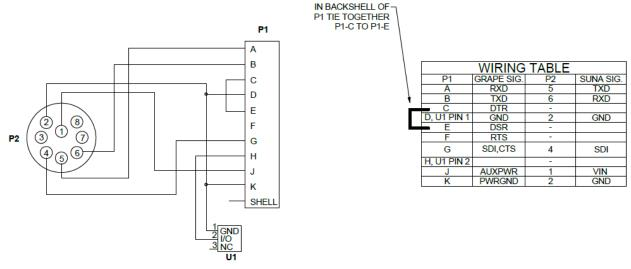
Figure 86. SUNA Power Cable Wiring.
