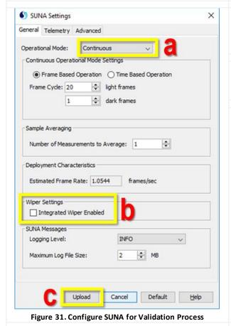
STEP 4 | In the SUNA Settings, switch the Operational Mode from "Periodic" to "Continuous" ("a" in Figure 31).
