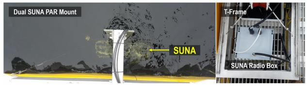
Figure 6. Dual SUNA PAR Mount and Radio Box on AIS Buoy.
