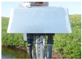
Figure 80. Reconnect Sensor Cable and Ethernet Cable to Grape
