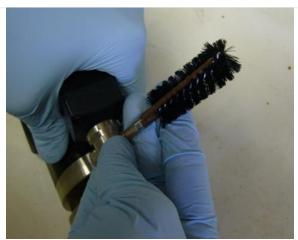
Figure 32. Physically Move Wiper on SUNA
