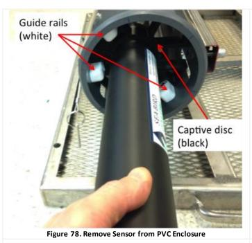
**STEP 8** | Slide the sensor assembly out of the enclosure by grabbing onto the wiper housing at the top of the sensor (**Figure 78**). The color of the captive discs may vary, but the design and material are the same across stream sites.
