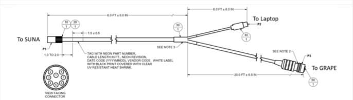
Figure 13. NEON Custom Y-Cable for Stream, Lake and River SUNA Field Validations/Calibrations (HB09780000)
