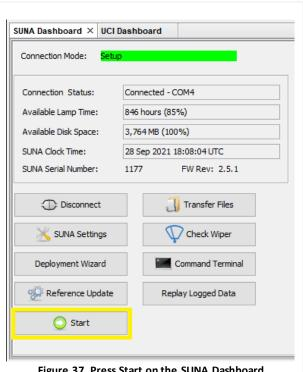
**STEP 1** | Press the "Start" button in the **SUNA** Dashboard to begin a real-time SUNA nitrate measurement (Figure 37).
