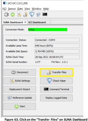
**STEP 7** | Transfer the .cal calibration file from the SUNA to the laptop.
