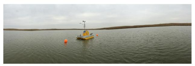
**Figure 5.** AIS Buoy for Lake and River Sites.
