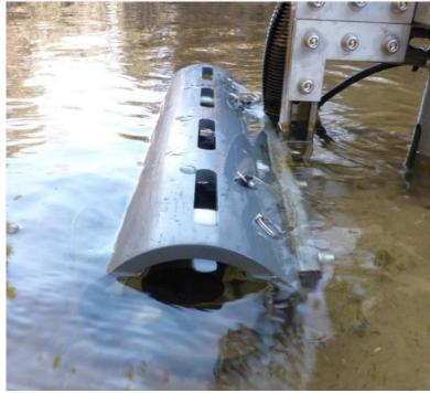
Figure 68. SUNA Partially Submerged in Stream
