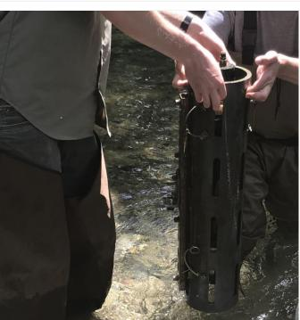
Figure 75. Remove SUNA PVC Enclosure
