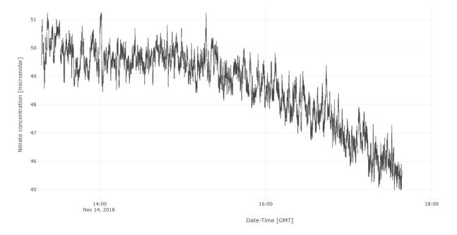
**Figure 93**. This example shows continuous data rather than 15 minute bursts. The SUNA was accidentally left in Continuous mode following PM. Reconnect to the SUNA and correct the settings to Periodic.
