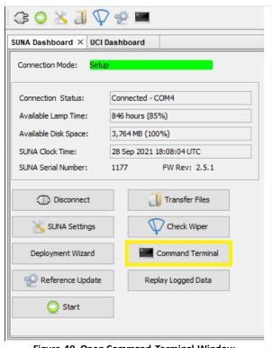
**STEP 1** | To verify the SUNA settings, click the "Command Terminal" button on the SUNA Dashboard (Figure 49).
