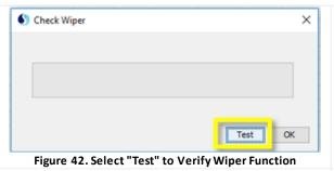
**STEP 3** | Select "Test" and watch the wiper move through the optical window (Figure 42).
