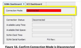
**STEP 2** | You must wait for the software to successfully disconnect from the SUNA; it will show the **Connection Mode** as "Disconnected" in red (**Figure 56**).
