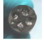
Lubricant pushed into the sockets of the connector
