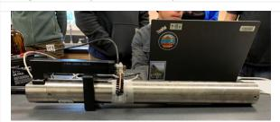
Figure 36. Validate SUNA Vertically to Prevent Bubbles on **Optical Bench**
