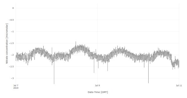
**Figure 90**. This example shows data with low variance and diel variation, but the concentrations are negative. The reference spectrum may have been calibrated incorrectly (the lens was not clean or DI was contaminated). Reperform the update. If the problem persists the SUNA needs to be serviced.
