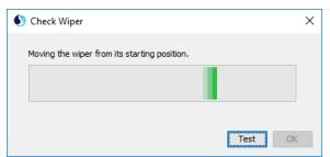
**STEP 4** | Monitor the wiper movement during the function test (**Figure 43**). Pay careful attention to verify if the wiper is sweeping through the entire window, stopping halfway through, or gets stuck on the edge of the window and does not complete a wipe
