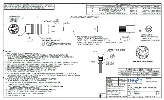
Figure 85. SUNA Power Cable Drawing.
