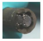
Lubricant on socket end of the connector
