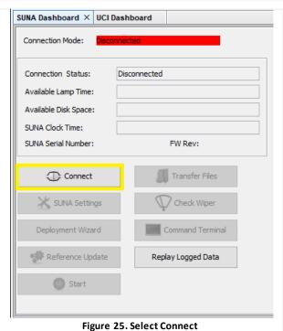
**STEP 8** | Launch UCI 2.0.3 (formerly SUNACom) on a laptop. Select the "Connect" button under the SUNA Dashboard (**Figure 25**).
