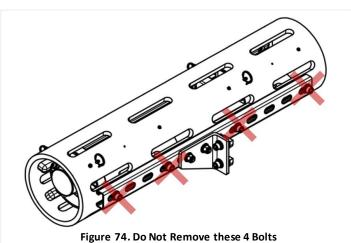
Do not remove these bolts, unless you want to have a bad time when reinstalling the enclosure (**Figure 74**).
