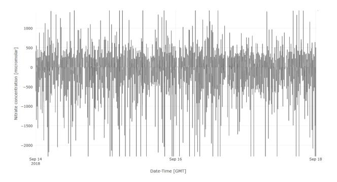
**Figure 91**. This example shows data with large variance both within and across bursts. The sensor is potentially fouled or the lamp has degraded. Check that the sensor is not buried, clean the optical lens, perform a reference spectrum update and then a self-test to measure the lamp output.
