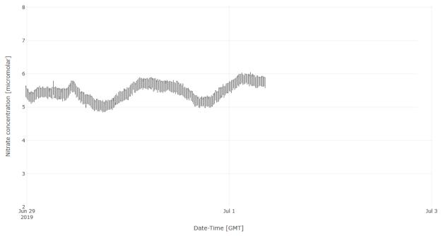
**Figure 94**. This example shows the SUNA was transmitting quality data until a PM occurred, at which point it stopped streaming. Check that UCI was exited out of correctly (5.5 Step 2), re-open and disconnected correctly if needed. Check that the SUNA cable was reconnected to the Grape data logger. Check that the SUNA was acquired by the Grape (5.5 Step 5); power cycle the Grape, if necessary.
