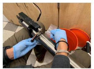
Figure 33. Cut Parafilm to Size
