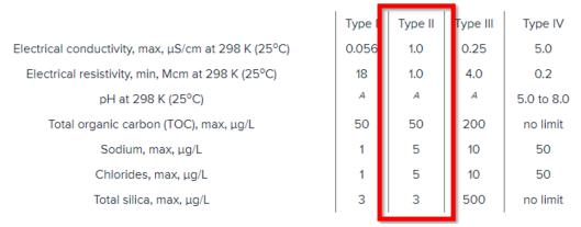
Figure 11. DI Water Minimum Requirements: ATSM Type II<sup>1</sup>.
