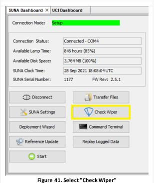
**STEP 2** | Verify wiper function by conducting wiper tests with the UCI software. Click on the "Check Wiper" button under the **SUNA Dashboard** (**Figure 41**).
