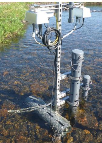
Figure 81. SUNA Cable Dressing - Complete Installation
