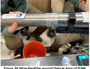
Figure 34. Wrap Parafilm around Optical Area of SUNA
