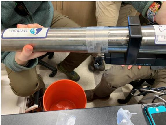
Figure 34. Wrap Parafilm around Optical Area of SUNA
