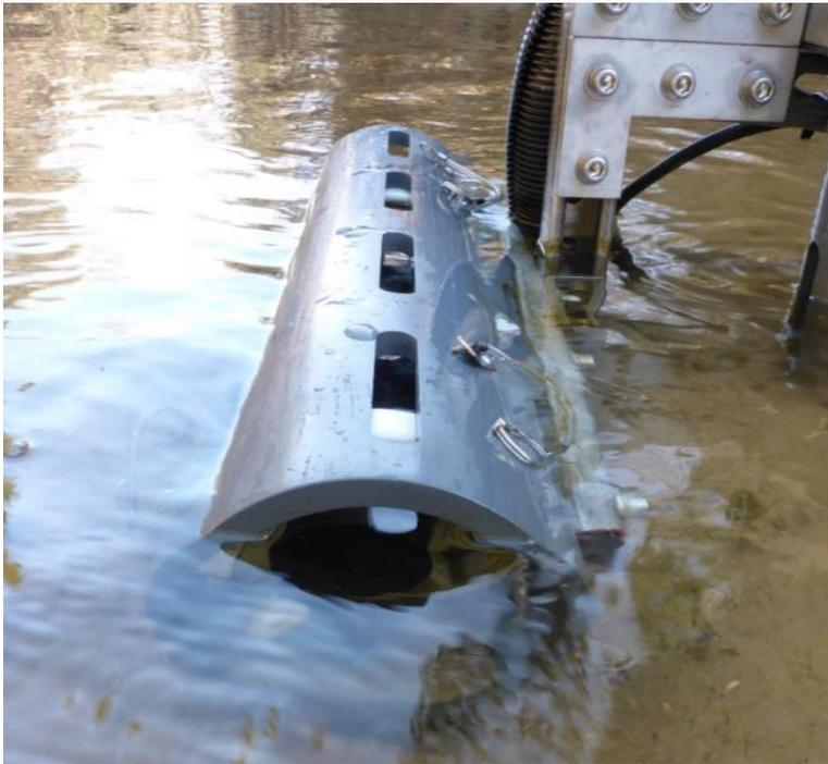
Figure 68. SUNA Partially Submerged in Stream
