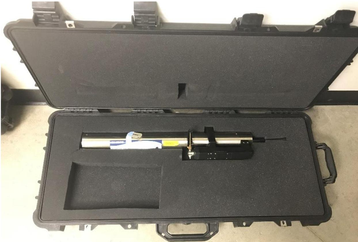
**Figure 82. Example of SUNA for Shipping/Storage.**
