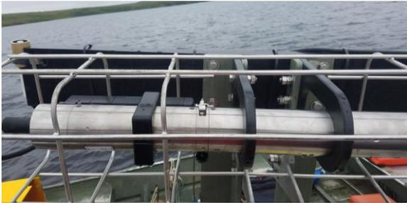
Figure 17. SUNA in Cage on Dual PAR SUNA Mount on the Buoy
