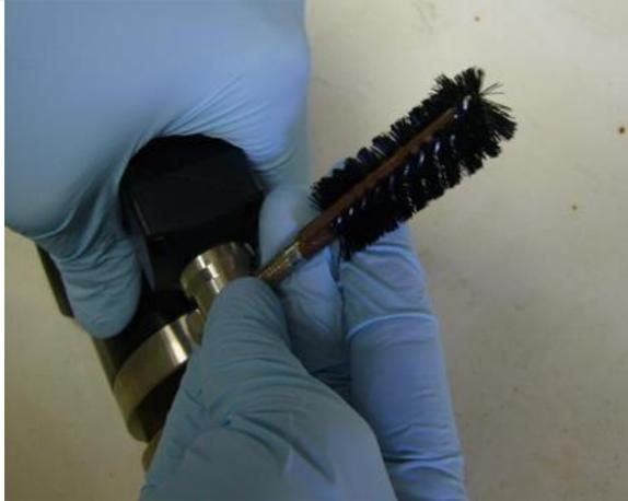
Figure 32. Physically Move Wiper on SUNA
