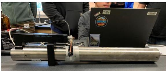
Figure 36. Validate SUNA Vertically to Prevent Bubbles on Optical Bench
