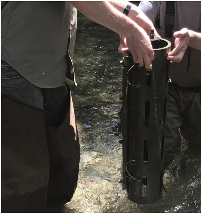
Figure 75. Remove SUNA PVC Enclosure
