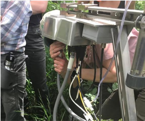
Figure 14. Disconnect the SUNA 12V Merlot Grape
