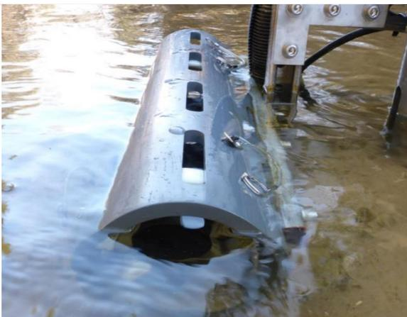
Figure 16. SUNA Mount and Enclosure in Stream Locations
